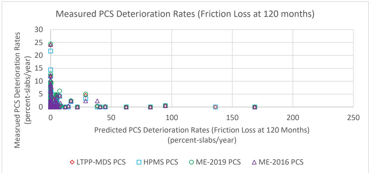
**Figure 8. Comparison Between the Predicted PCS Rate from MEPDG and Other PCS Prediction Methods for the Scenario with Friction-Loss at 120 Months**
