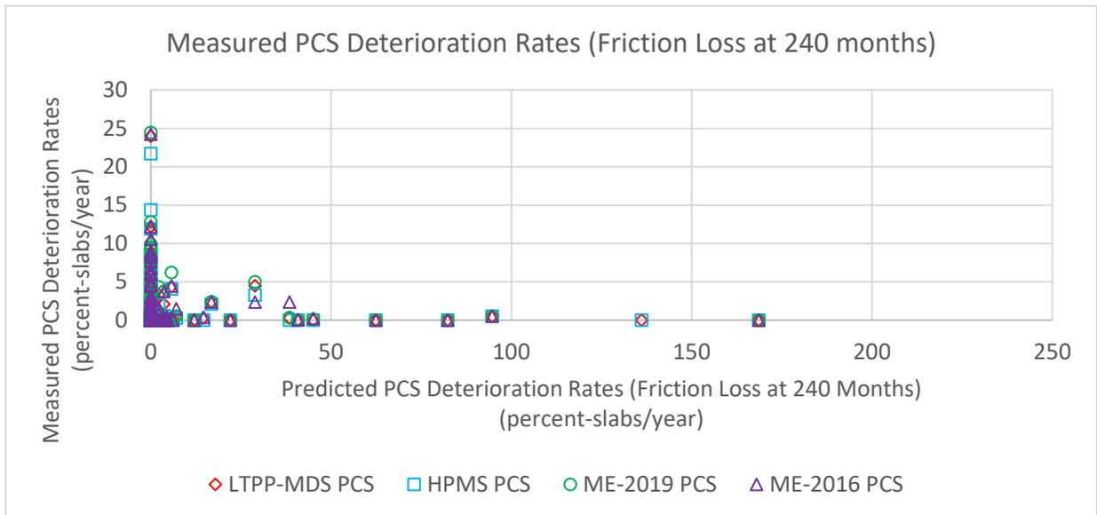
**Figure 9. Comparison Between the Predicted PCS Rate from MEPDG and Other PCS Prediction Methods for the Scenario with Friction-Loss at 240 Months**
