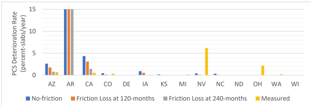
**Figure A 6. Comparison Between Measured and Predicted Deterioration Rates for PCS on Average by State.**
