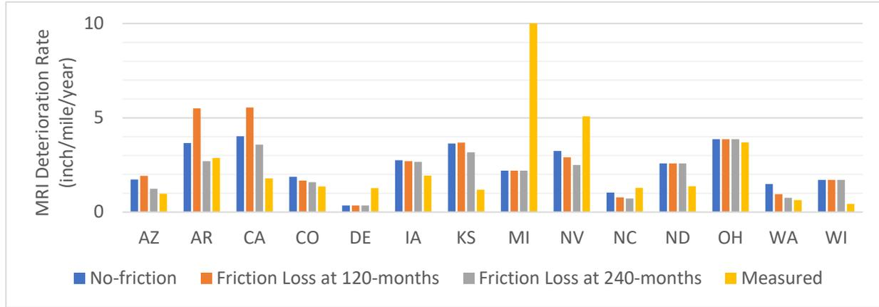
**Figure A 22. Comparison Between Measured and Predicted Deterioration Rates for MRI on Average by State.**
