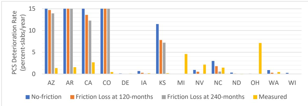
**Figure A 3. Comparison Between Measured and Predicted Deterioration Rates for PCS on Average by State.**
