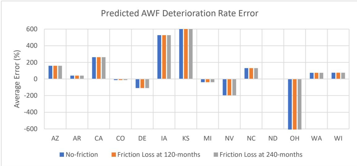
**Figure B 26. Average Error (%) Between AWF Deterioration Rates When Comparing the Predicted Values to the LTPP Measured Values.**
