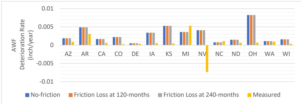
**Figure A 2. Comparison Between Measured and Predicted Deterioration Rates for AWF on Average by State.**
