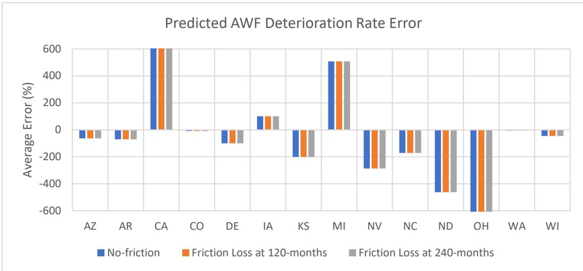
**Figure B 23. Average Error (%) Between AWF Deterioration Rates When Comparing the Predicted Values to the LTPP Measured Values.**
