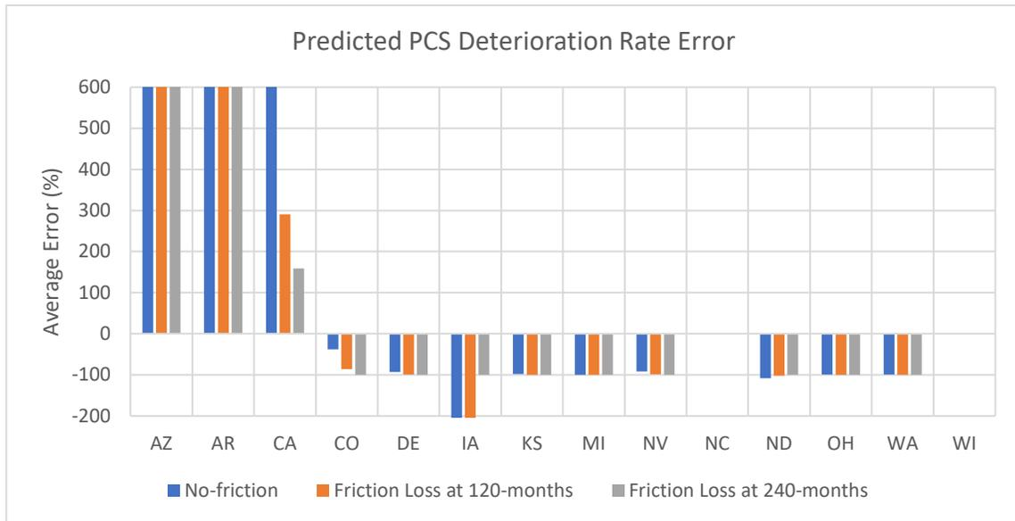
**Figure B 27. Average Error (%) Between PCS Deterioration Rates When Comparing the Predicted Values to the LTPP Measured Values.**
