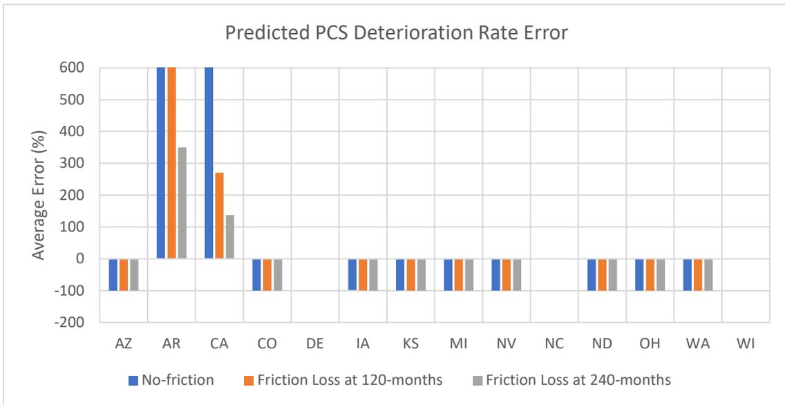
**Figure B 21. Average Error (%) Between PCS Deterioration Rates When Comparing the Predicted Values to the LTPP Measured Values.**
