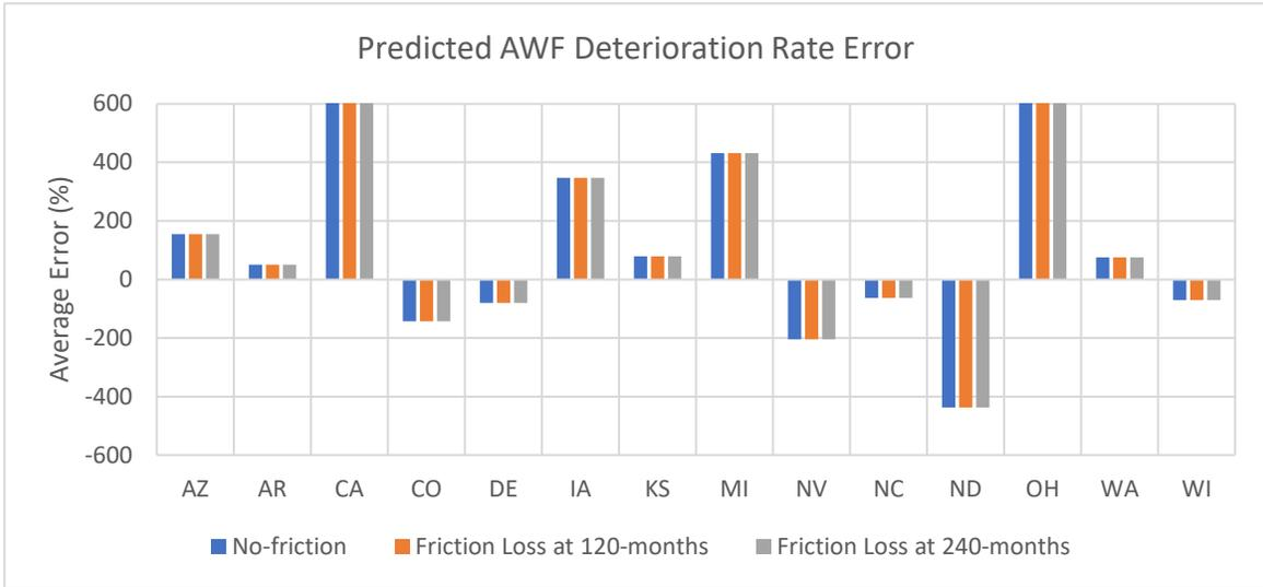
**Figure B 20. Average Error (%) Between AWF Deterioration Rates When Comparing the Predicted Values to the LTPP Measured Values.**
