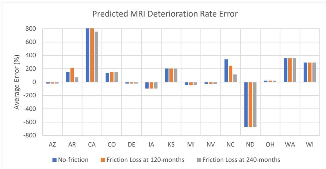
**Figure B 19. Average Error (%) Between MRI Deterioration Rates When Comparing the Predicted Values to the LTPP Measured Values.**
