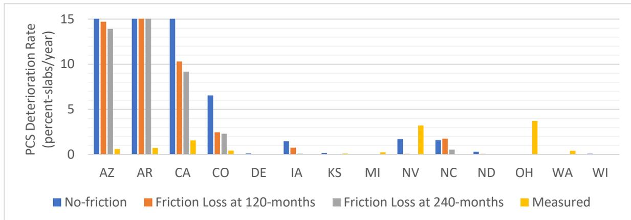
**Figure A 27. Comparison Between Measured and Predicted Deterioration Rates for PCS on Average by State.**
