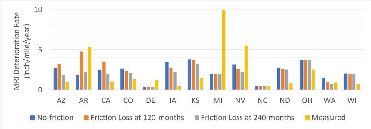
**Figure A 16. Comparison Between Measured and Predicted Deterioration Rates for MRI on Average by State.**
