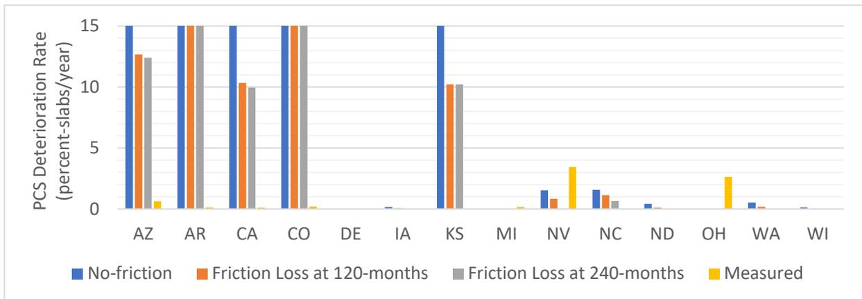
**Figure A 15. Comparison Between Measured and Predicted Deterioration Rates for PCS on Average by State.**
