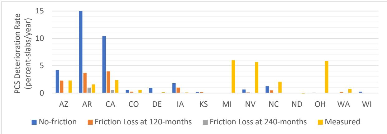
**Figure A 12. Comparison Between Measured and Predicted Deterioration Rates for PCS on Average by State.**
