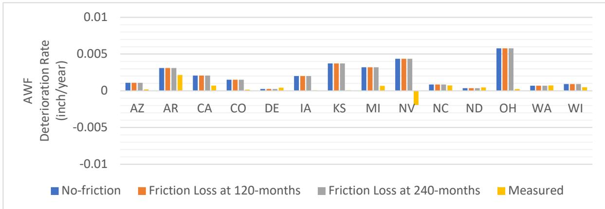
**Figure A 14. Comparison Between Measured and Predicted Deterioration Rates for AWF on Average by State.**
