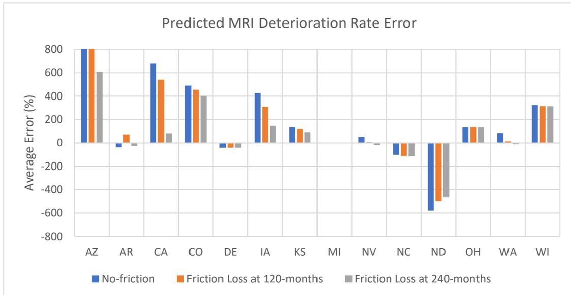
**Figure B 16. Average Error (%) Between MRI Deterioration Rates When Comparing the Predicted Values to the LTPP Measured Values.**
