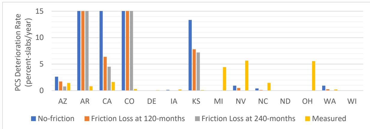
**Figure A 24. Comparison Between Measured and Predicted Deterioration Rates for PCS on Average by State.**
