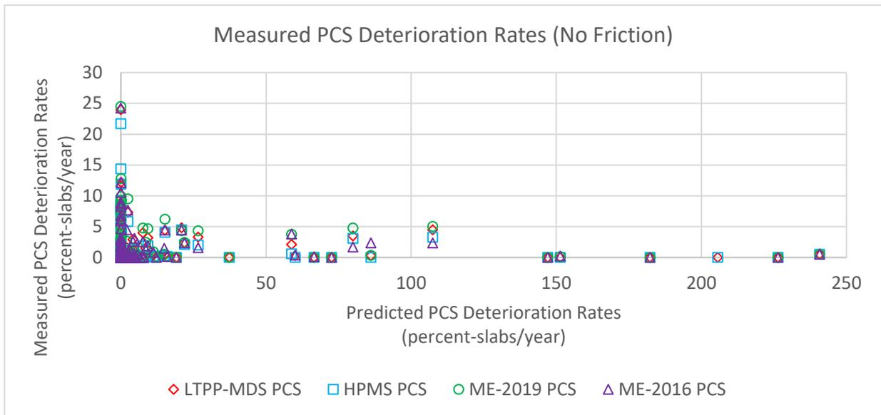
**Figure 7. Comparison Between the Predicted PCS Rate from MEPDG and Other PCS Prediction Methods for the Scenario with No Initial Friction**
