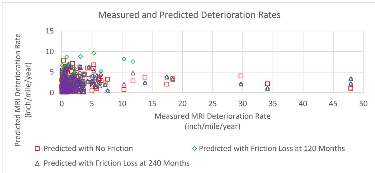
Figure 4. Comparison Between Predicted and Measured MRI Deterioration Rates for Each Test Section
