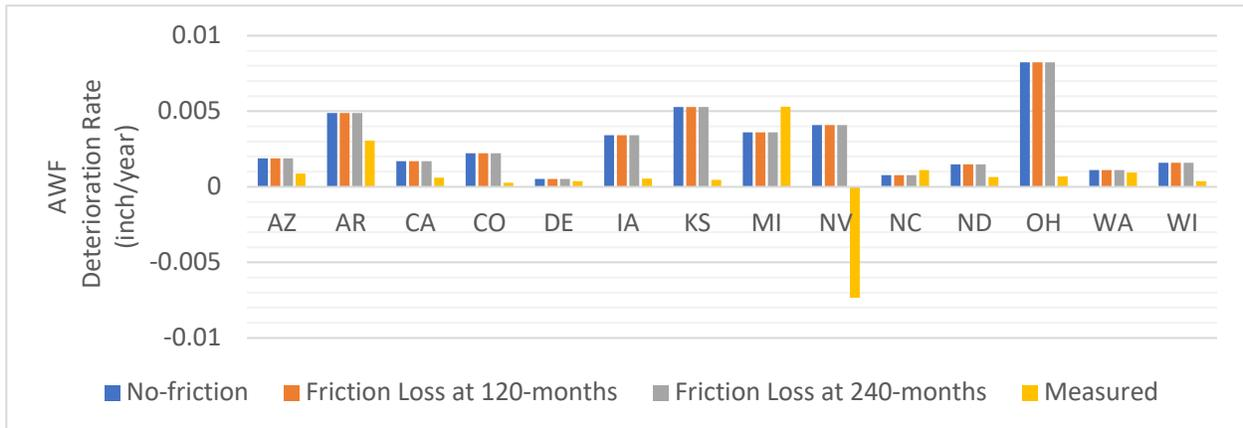
**Figure A 5. Comparison Between Measured and Predicted Deterioration Rates for AWF on Average by State.**
