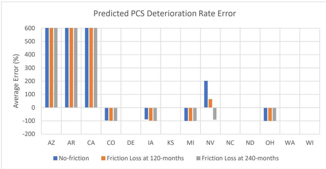
**Figure B 15. Average Error (%) Between PCS Deterioration Rates When Comparing the Predicted Values to the LTPP Measured Values.**
