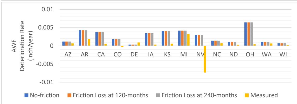
**Figure A 20. Comparison Between Measured and Predicted Deterioration Rates for AWF on Average by State.**
