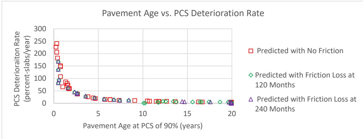
As seen in Figures 1 and 2, test sections in the 120-month and 240-month scenarios with a pavement age range of 0-to-10 years match up in terms of PCS deterioration. Only after the 10 years do test sections in the 120-month and 240-scenarios show different PCS deterioration rates. Test sections in the no-friction scenario were predicted to deteriorate faster than test sections with full-friction.
