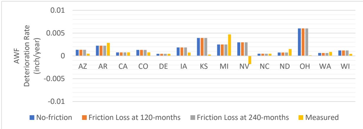
**Figure A 17. Comparison Between Measured and Predicted Deterioration Rates for AWF on Average by State.**
