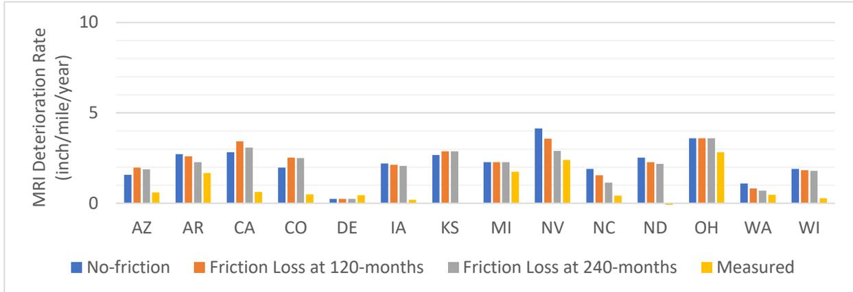
**Figure A 13. Comparison Between Measured and Predicted Deterioration Rates for MRI on Average by State.**
