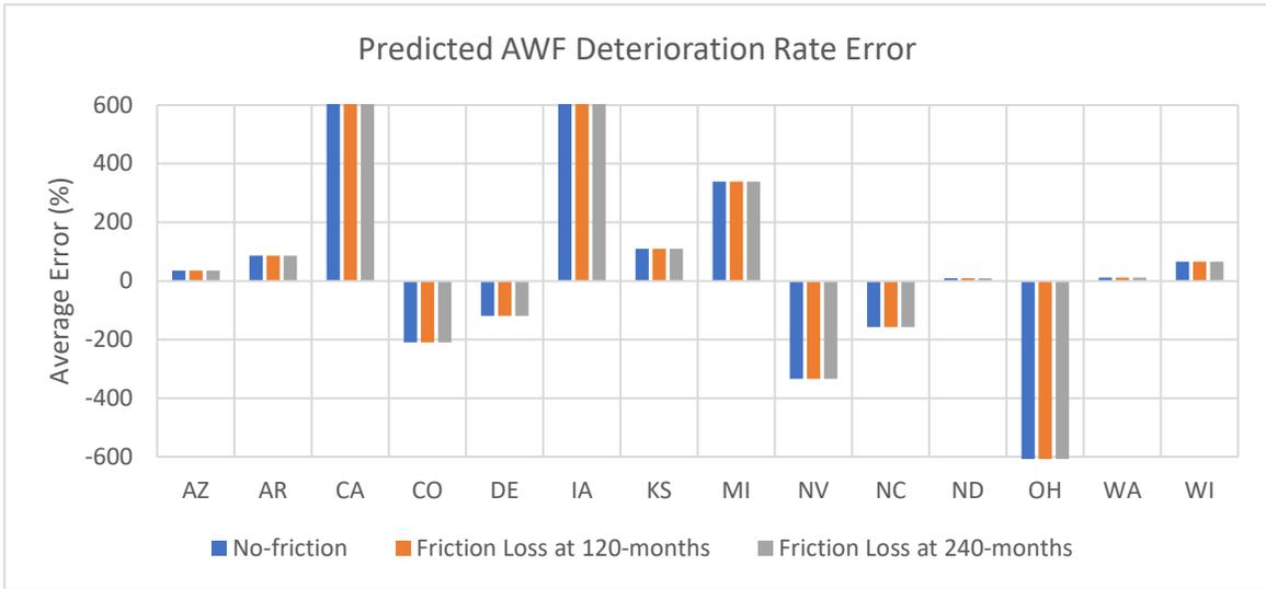
**Figure B 14. Average Error (%) Between AWF Deterioration Rates When Comparing the Predicted Values to the LTPP Measured Values.**
