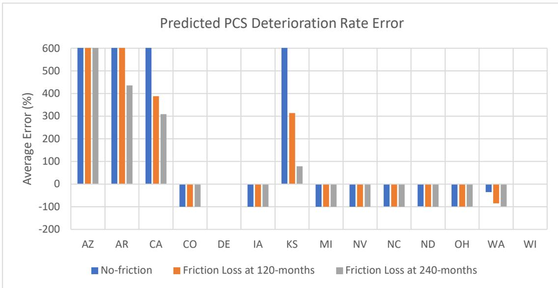
**Figure B 9. Average Error (%) Between PCS Deterioration Rates When Comparing the Predicted Values to the LTPP Measured Values.**
