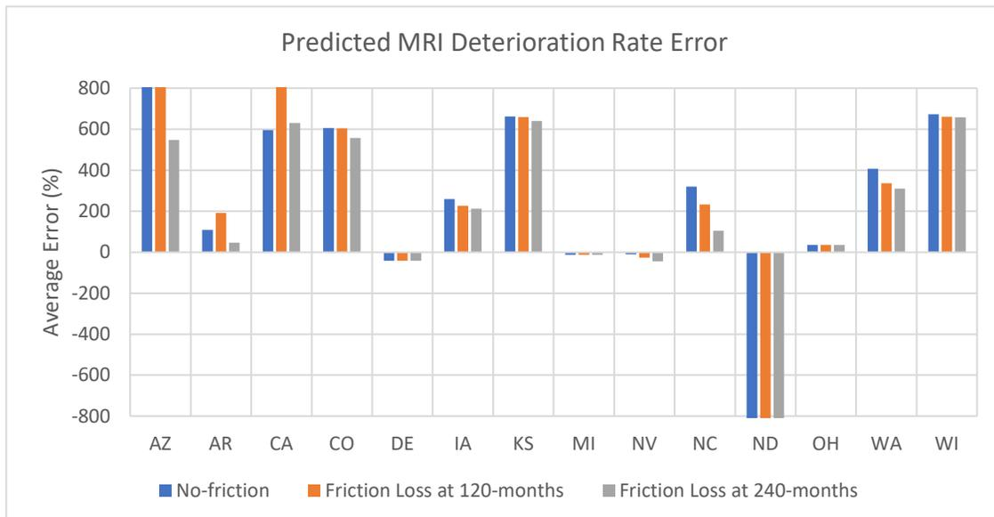
**Figure B 1. Average Error (%) Between MRI Deterioration Rates When Comparing the Predicted Values to the LTPP Measured Values.**
