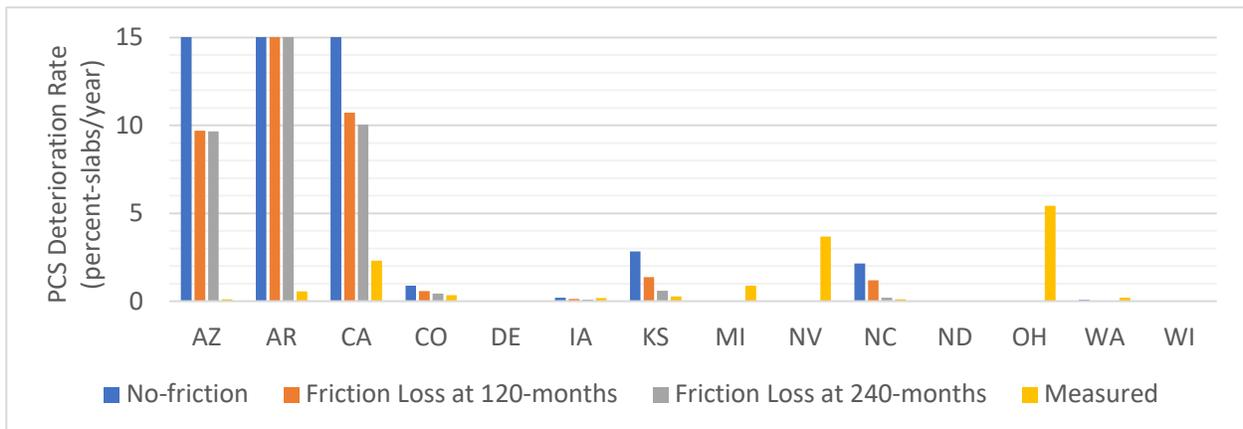
**Figure A 9. Comparison Between Measured and Predicted Deterioration Rates for PCS on Average by State.**
