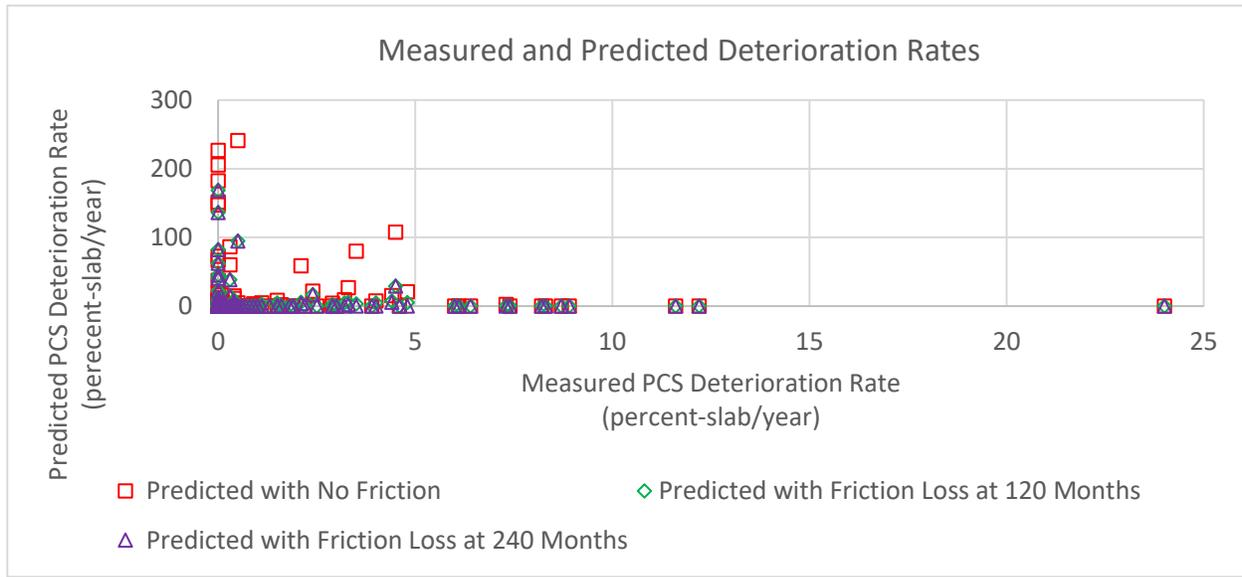
**Figure 6. Comparison Between Predicted and measured PCS Deterioration Rates for Each Test Section**
