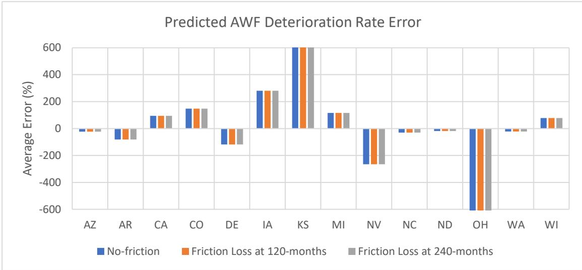
**Figure B 17. Average Error (%) Between AWF Deterioration Rates When Comparing the Predicted Values to the LTPP Measured Values.**
