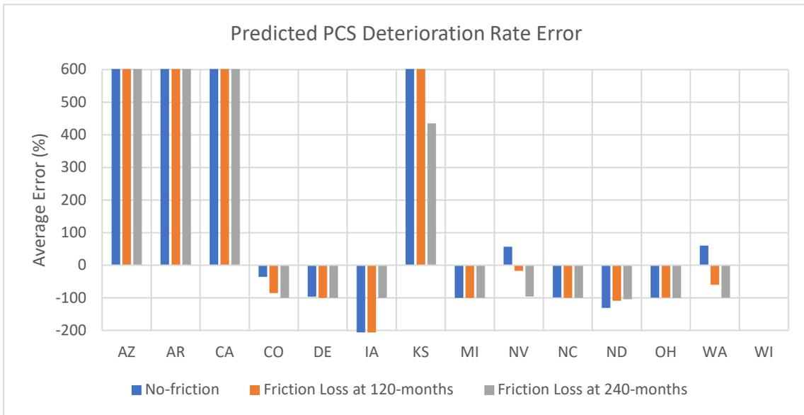
**Figure B 18. Average Error (%) Between PCS Deterioration Rates When Comparing the Predicted Values to the LTPP Measured Values.**
