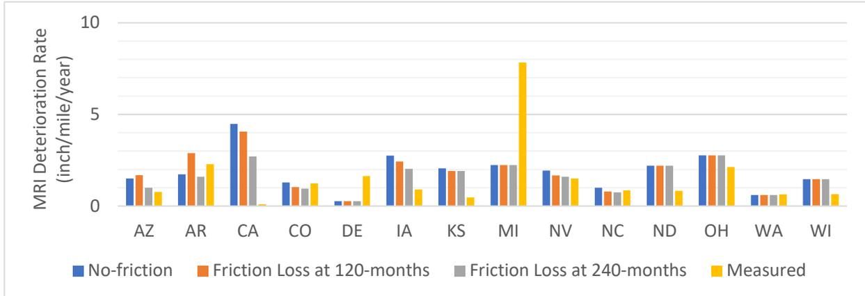
**Figure A 4. Comparison Between Measured and Predicted Deterioration Rates for MRI on Average by State.**
