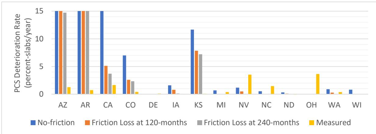
**Figure A 18. Comparison Between Measured and Predicted Deterioration Rates for PCS on Average by State.**
