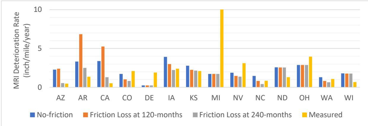
**Figure A 10. Comparison Between Measured and Predicted Deterioration Rates for MRI on Average by State.**
