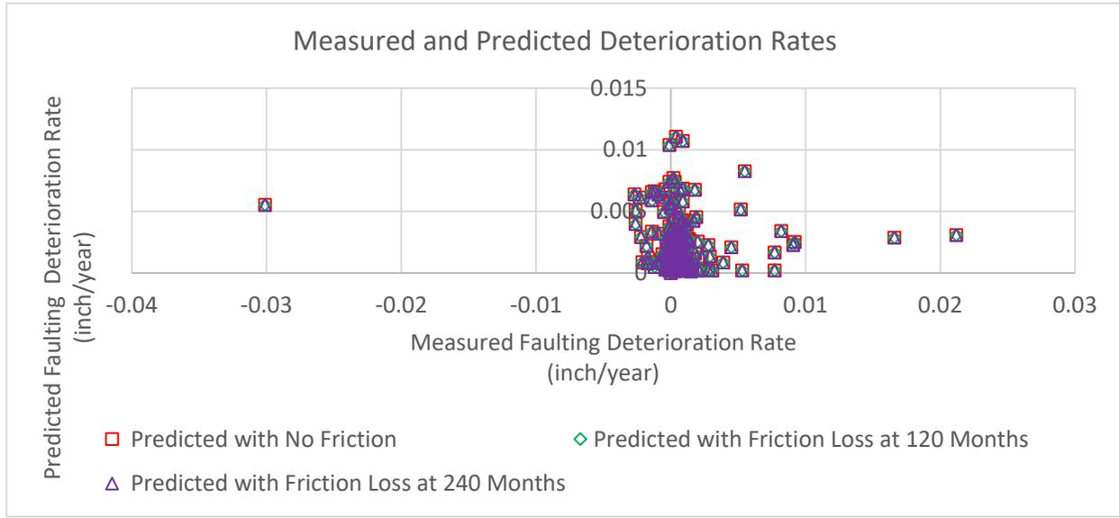
**Figure 5. Comparison Between Predicted and Measured AWF Deterioration Rates for Each Test Section**
