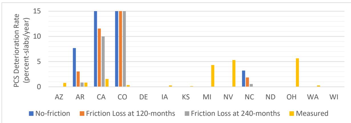
**Figure A 21. Comparison Between Measured and Predicted Deterioration Rates for PCS on Average by State.**
