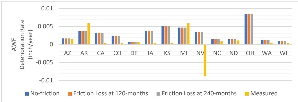
**Figure A 8. Comparison Between Measured and Predicted Deterioration Rates for AWF on Average by State.**
