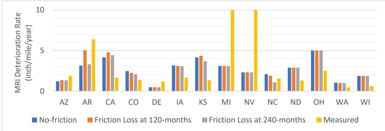
**Figure A 7. Comparison Between Measured and Predicted Deterioration Rates for MRI on Average by State.**
