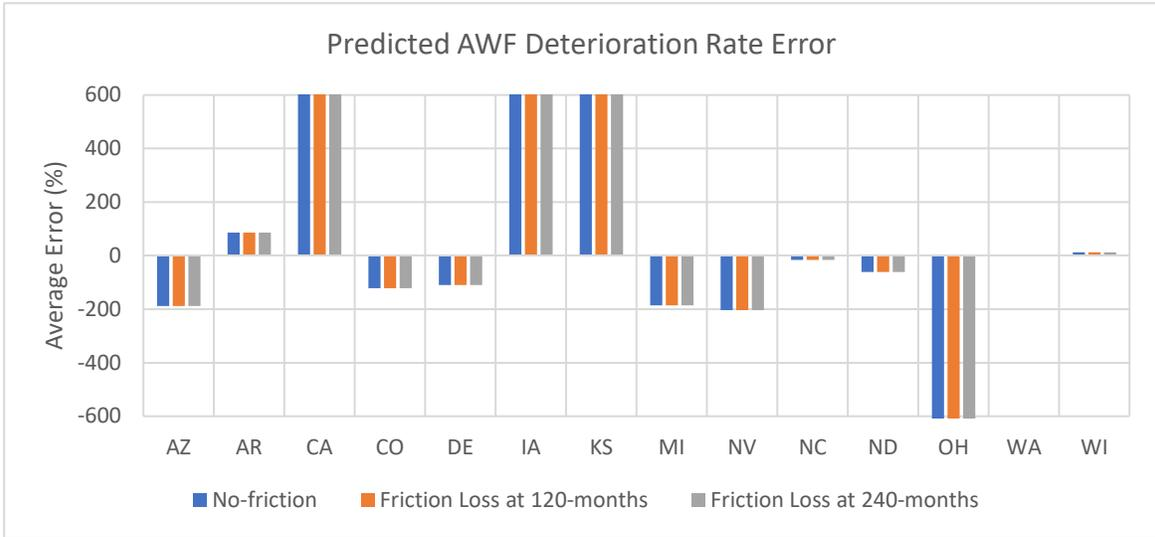
**Figure B 5. Average Error (%) Between AWF Deterioration Rates When Comparing the Predicted Values to the LTPP Measured Values.**
