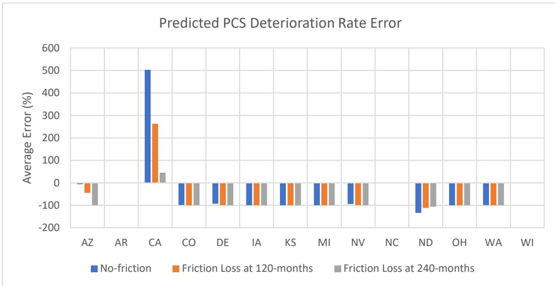
**Figure B 6. Average Error (%) Between PCS Deterioration Rates When Comparing the Predicted Values to the LTPP Measured Values.**
