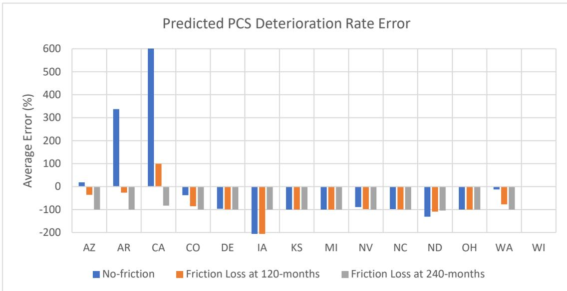
**Figure B 12. Average Error (%) Between PCS Deterioration Rates When Comparing the Predicted Values to the LTPP Measured Values.**
