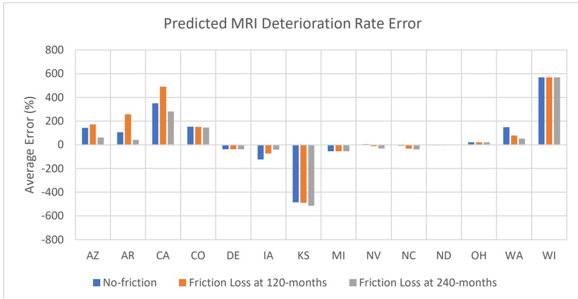
**Figure B 22. Average Error (%) Between MRI Deterioration Rates When Comparing the Predicted Values to the LTPP Measured Values.**
