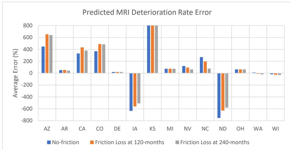
**Figure B 13. Average Error (%) Between MRI Deterioration Rates When Comparing the Predicted Values to the LTPP Measured Values.**
