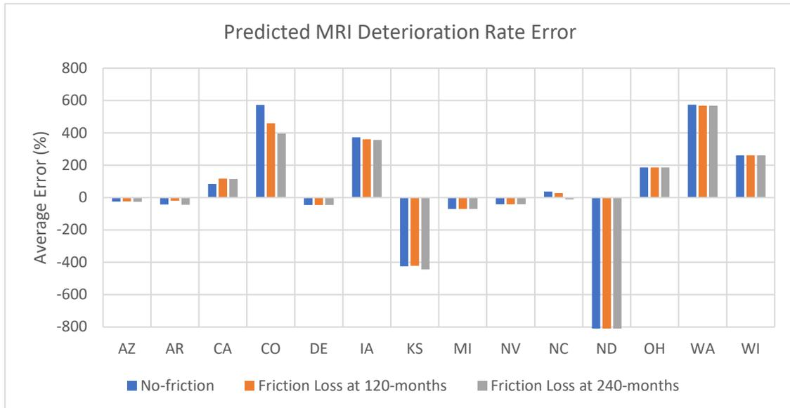
**Figure B 7. Average Error (%) Between MRI Deterioration Rates When Comparing the Predicted Values to the LTPP Measured Values.**
