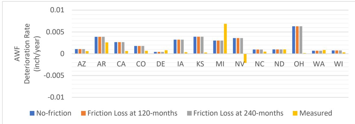
**Figure A 23. Comparison Between Measured and Predicted Deterioration Rates for AWF on Average by State.**
