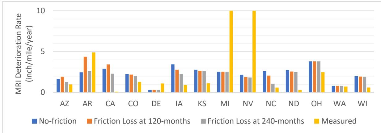
**Figure A 25. Comparison Between Measured and Predicted Deterioration Rates for MRI on Average by State.**
