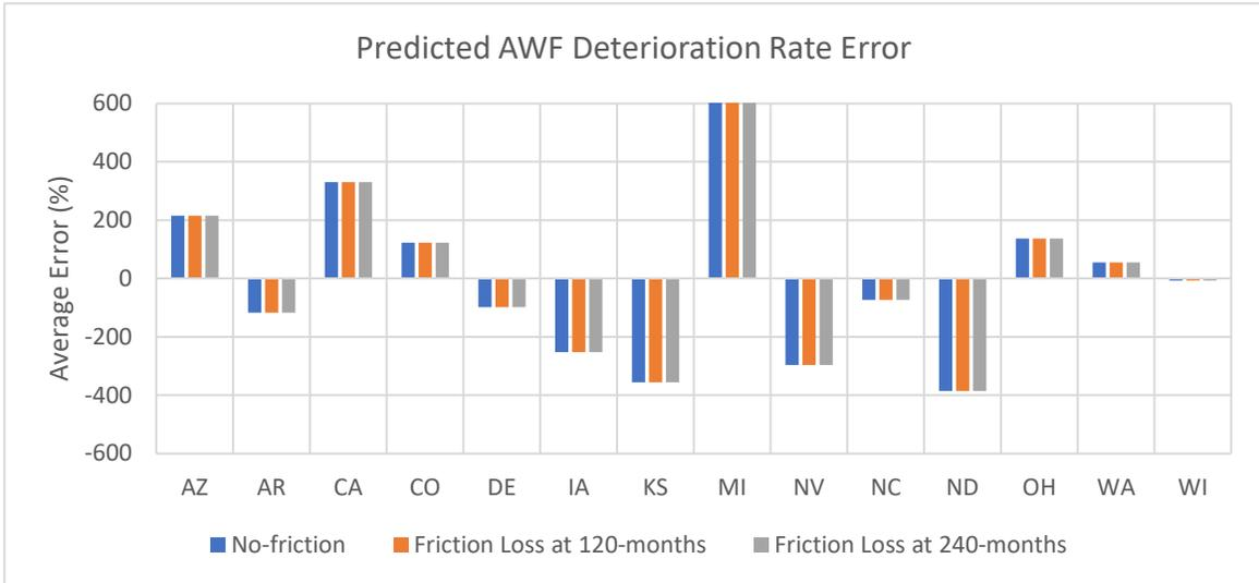
**Figure B 2. Average Error (%) Between AWF Deterioration Rates When Comparing the Predicted Values to the LTPP Measured Values.**
