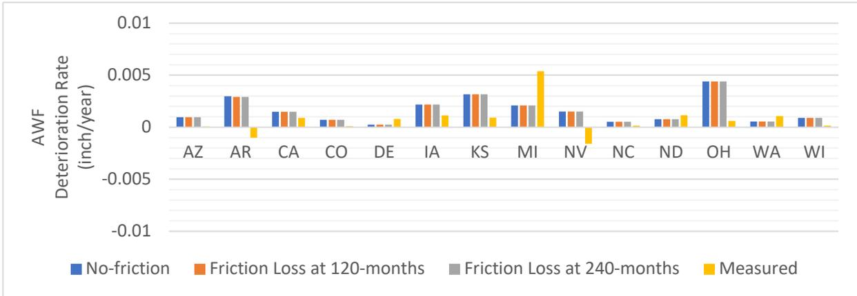
**Figure A 11. Comparison Between Measured and Predicted Deterioration Rates for AWF on Average by State.**
