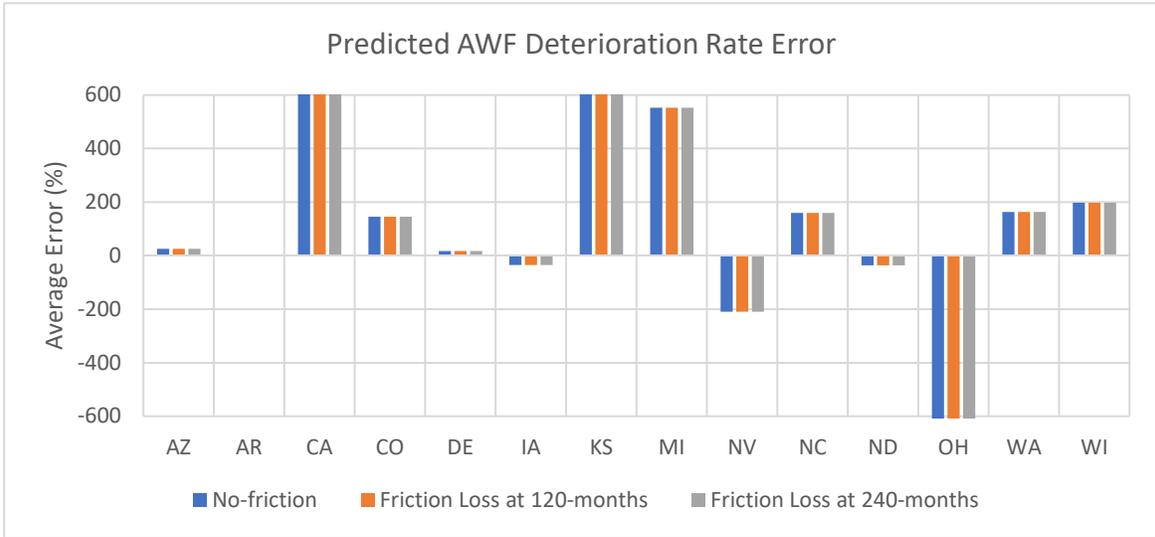
**Figure B 8. Average Error (%) Between AWF Deterioration Rates When Comparing the Predicted Values to the LTPP Measured Values.**
