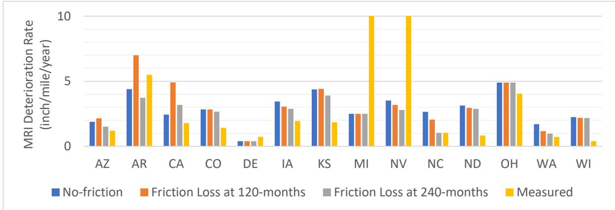
**Figure A 1. Comparison Between Measured and Predicted Deterioration Rates for MRI on Average by State.**
