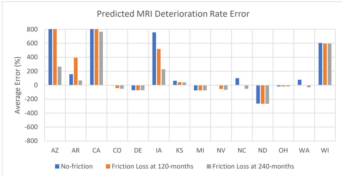
**Figure B 10. Average Error (%) Between MRI Deterioration Rates When Comparing the Predicted Values to the LTPP Measured Values.**
