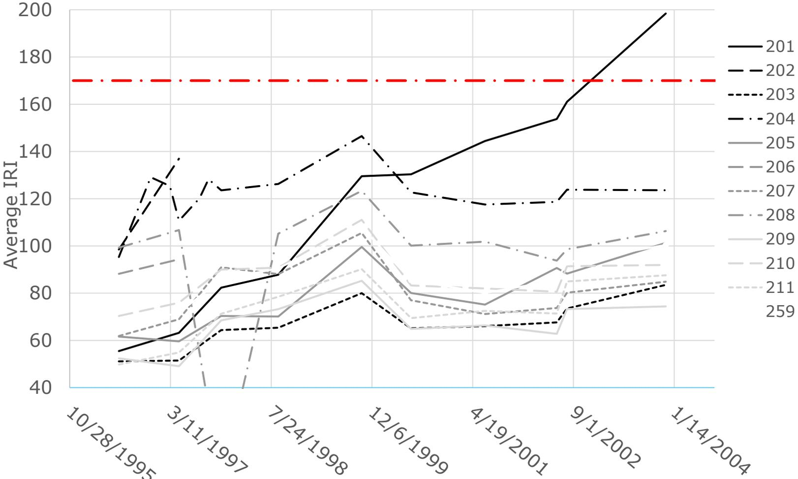
Figure 27. Average Roughness (in IRI) for Nevada SPS-2 Test Sections
