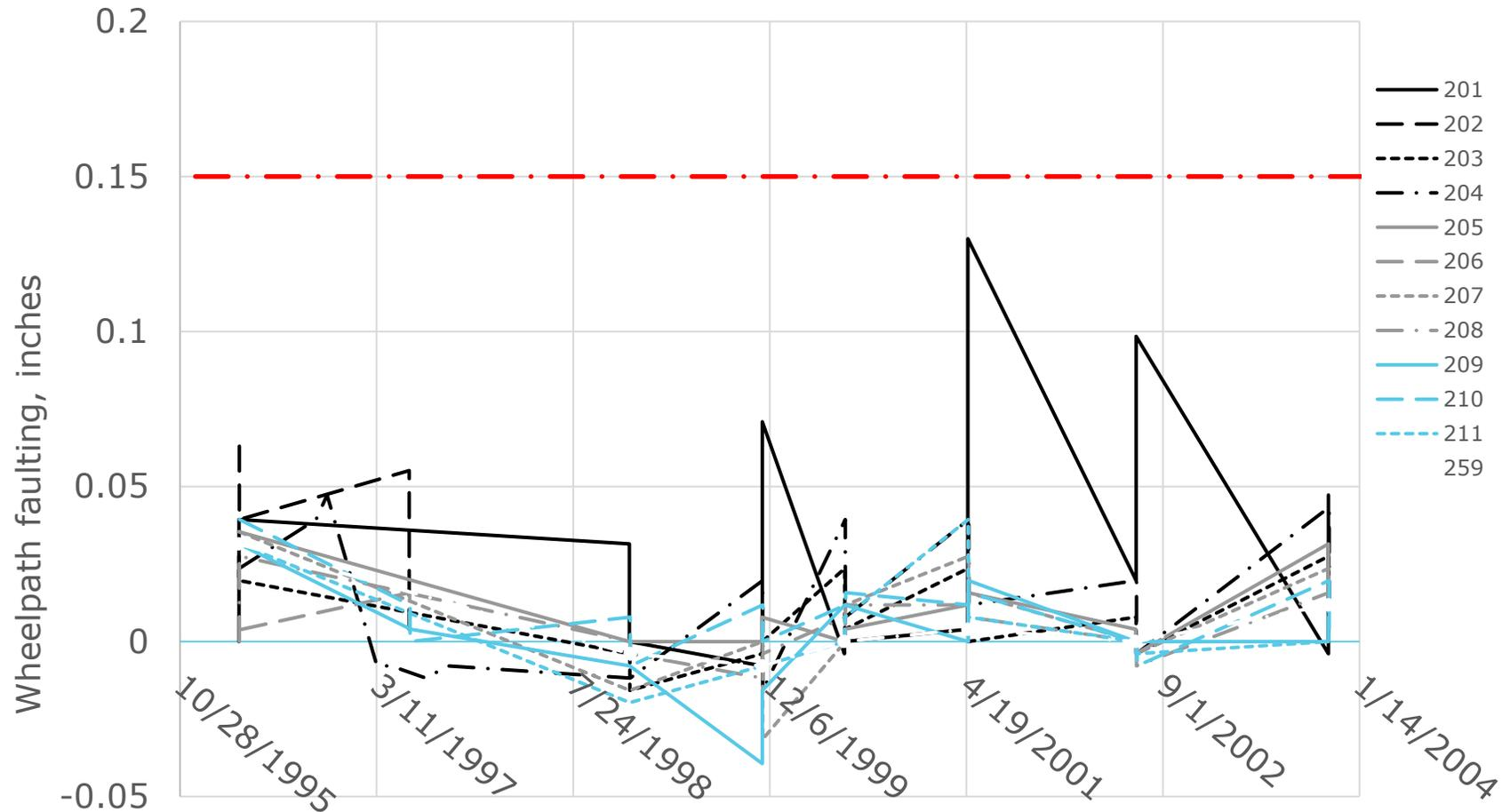
**Figure 28. Average Wheel-Path faulting (in inches) for Nevada SPS-2 Test Sections**
