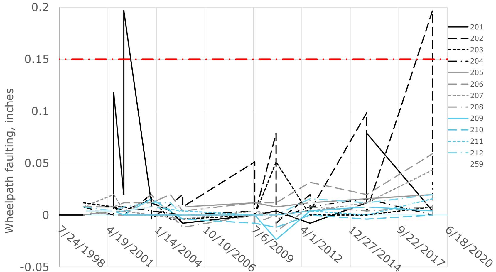
Figure 20. Average Wheel-Path faulting (in inches) of Kansas SPS-2 Test Sections
