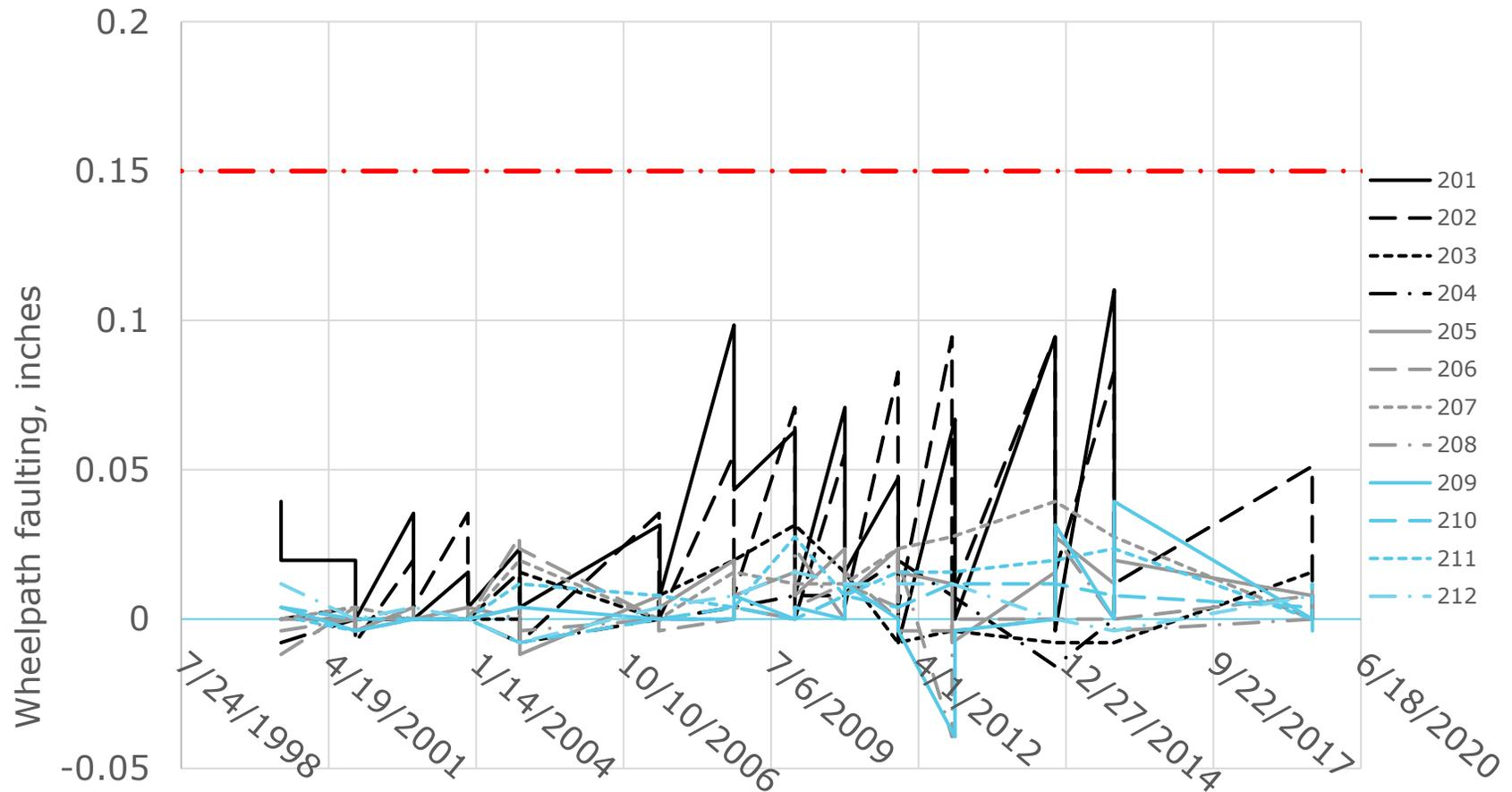
**Figure 8. Average Wheel Path Faulting (in inches) for California SPS-2 Test Sections**
