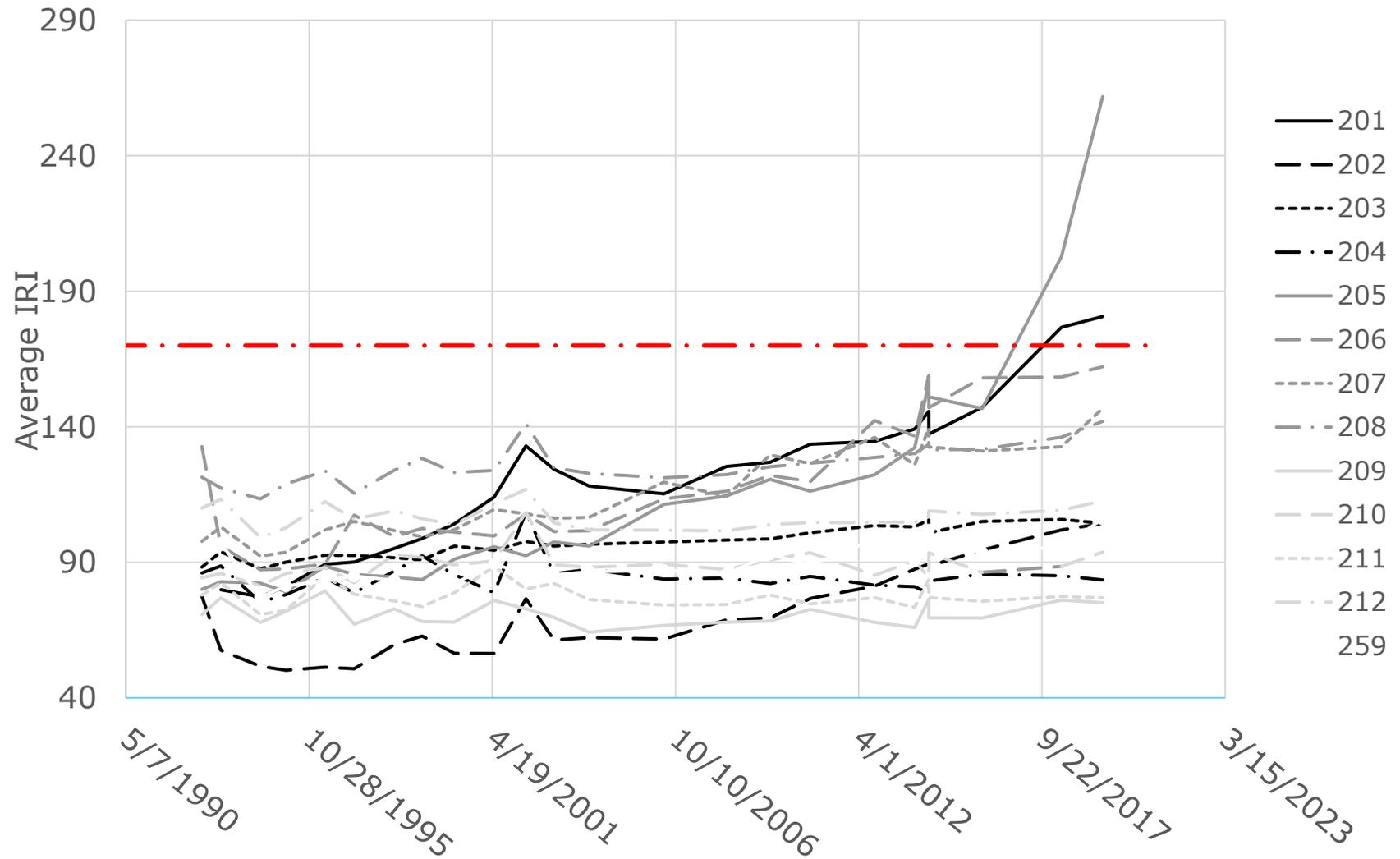
**Figure 19. Average Roughness (in IRI) of Kansas SPS-2 Test Sections**
