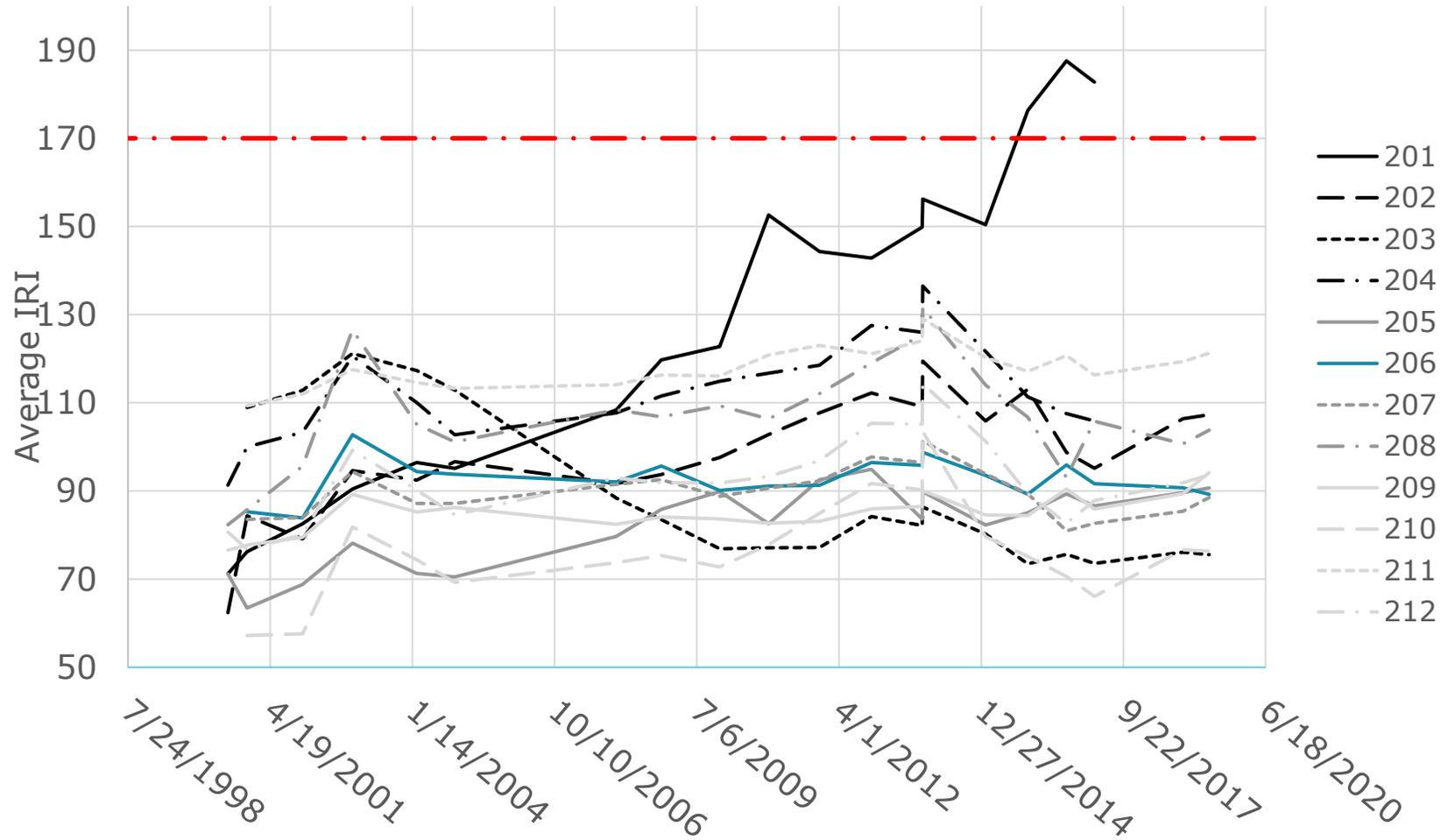
**Figure 7. Average Measured Roughness (in IRI) for California SPS-2 Test Sections**
