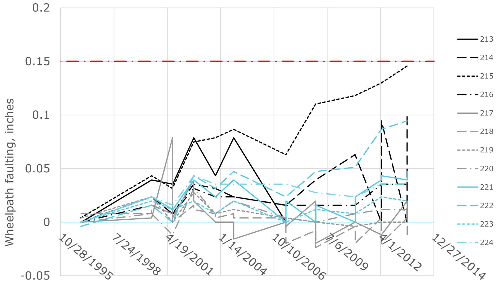
**Figure 5. Average Wheel-Path faulting (in inches) for Arkansas SPS-2 Test Sections**
