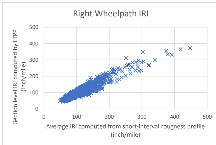
**Figure 8: Comparison of Computed IRI in the Right Wheel Path**
