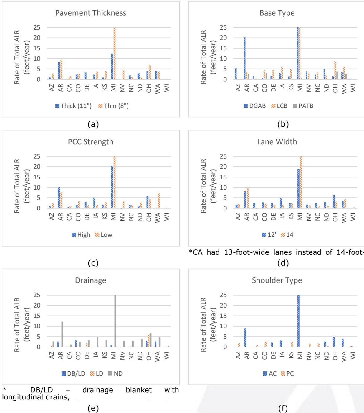
**Figure 12: Average Rate of Change in Total ALR by Design Factor and State**
