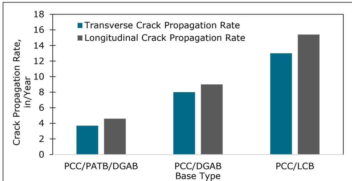
**Figure 1: Effect of Base type on Crack Propagation Rate**
