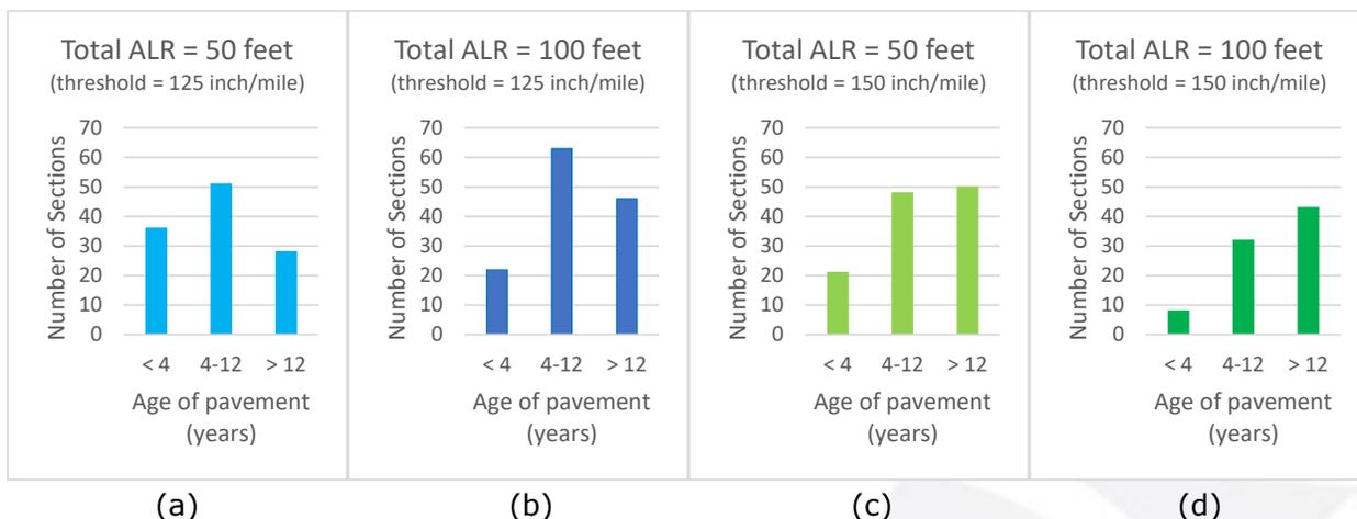
**Figure 10: Total ALR in the Right Wheel Path Versus Pavement Age**
