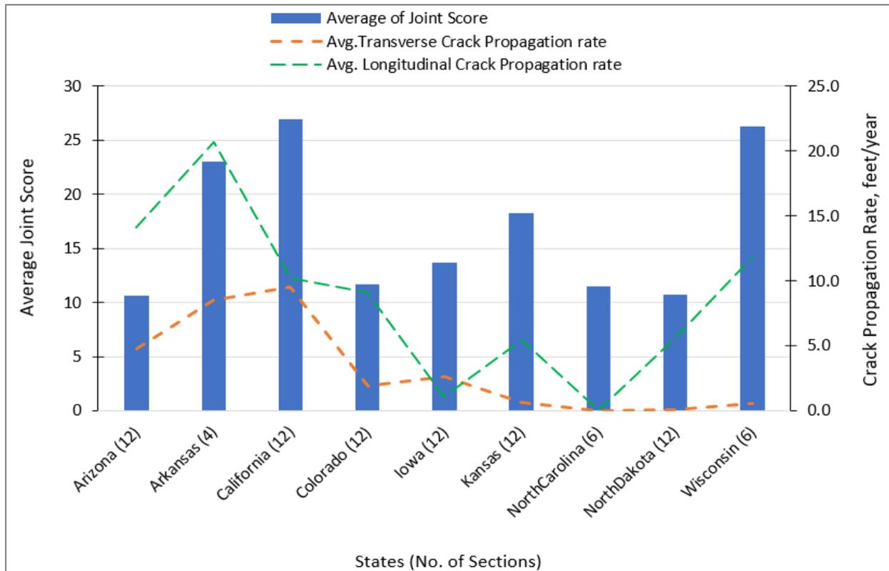
**Figure 3. Relationship between Joint Score and Crack Propagation Rate for Different States**
