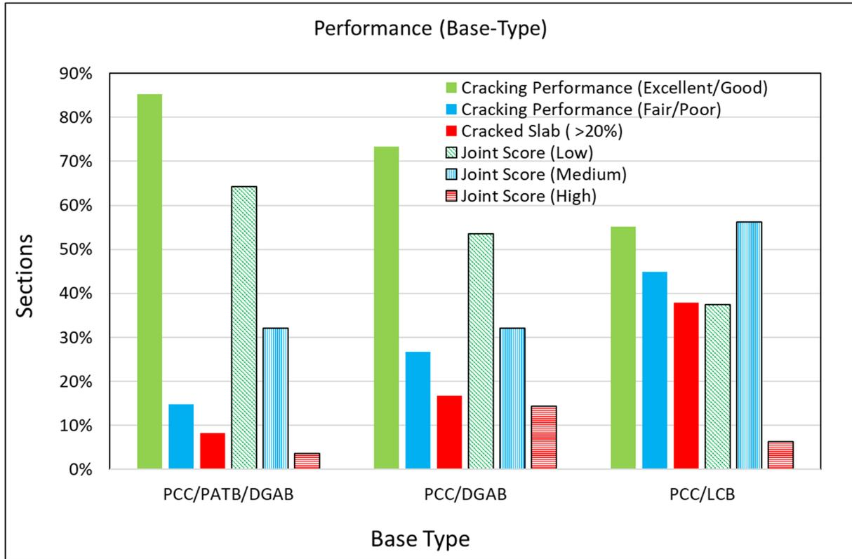
**Figure 4: Effect of Base Type on Cracking Performance**
