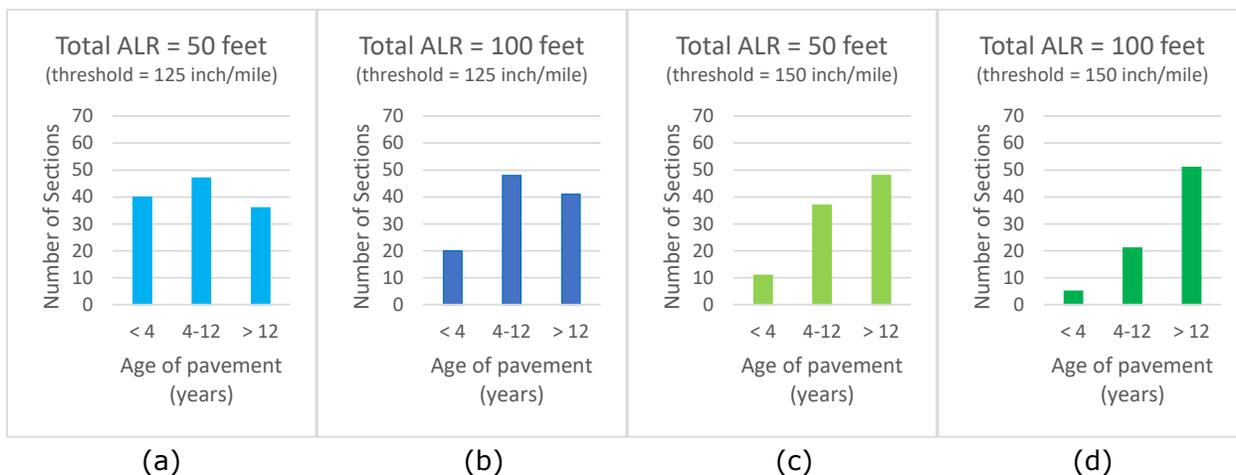
**Figure 9: Total ALR in the Left Wheel Path Versus Pavement Age**
