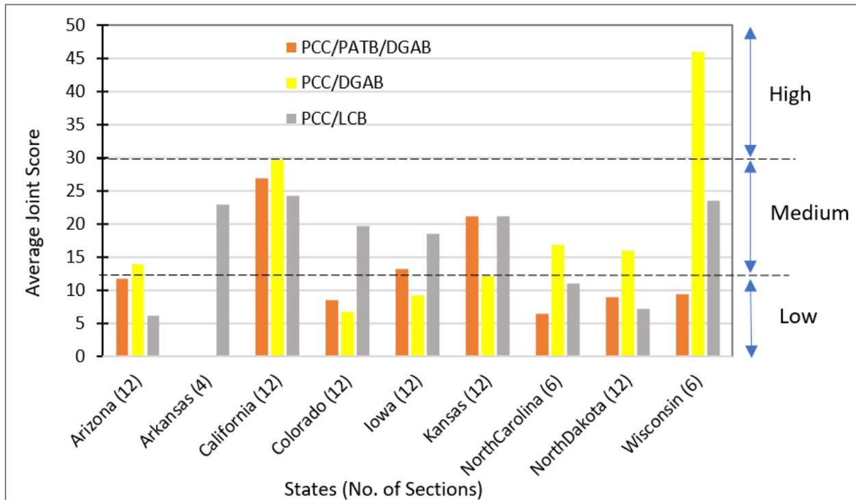
**Figure 2. Average Joint Score of Different States based on Different Base-Types**
