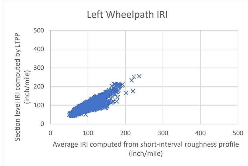
**Figure 7: Comparison of Computed IRI in the Left Wheel Path**
