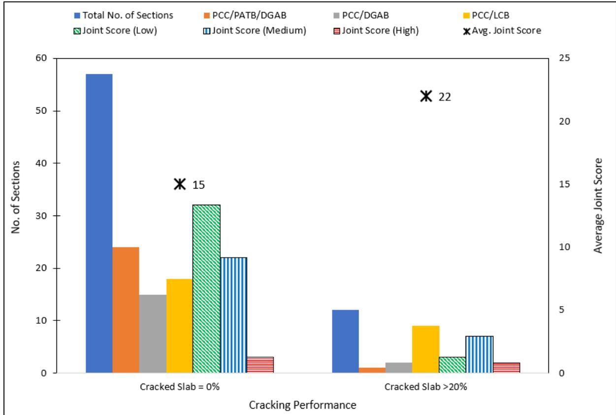
**Figure 6: Effect of Base Type and Joint Score on Cracked Slabs**
