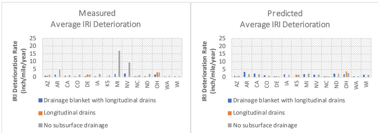
**Figure 13. Deterioration Rates for Measured and Predicted IRI by Drainage Feature**
