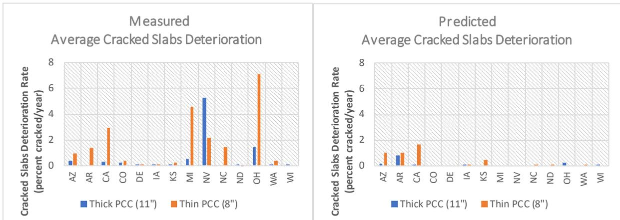
**Figure 3. Deterioration Rates for Measured and Predicted Transversely Cracked Slabs by PCC Design Thickness**
