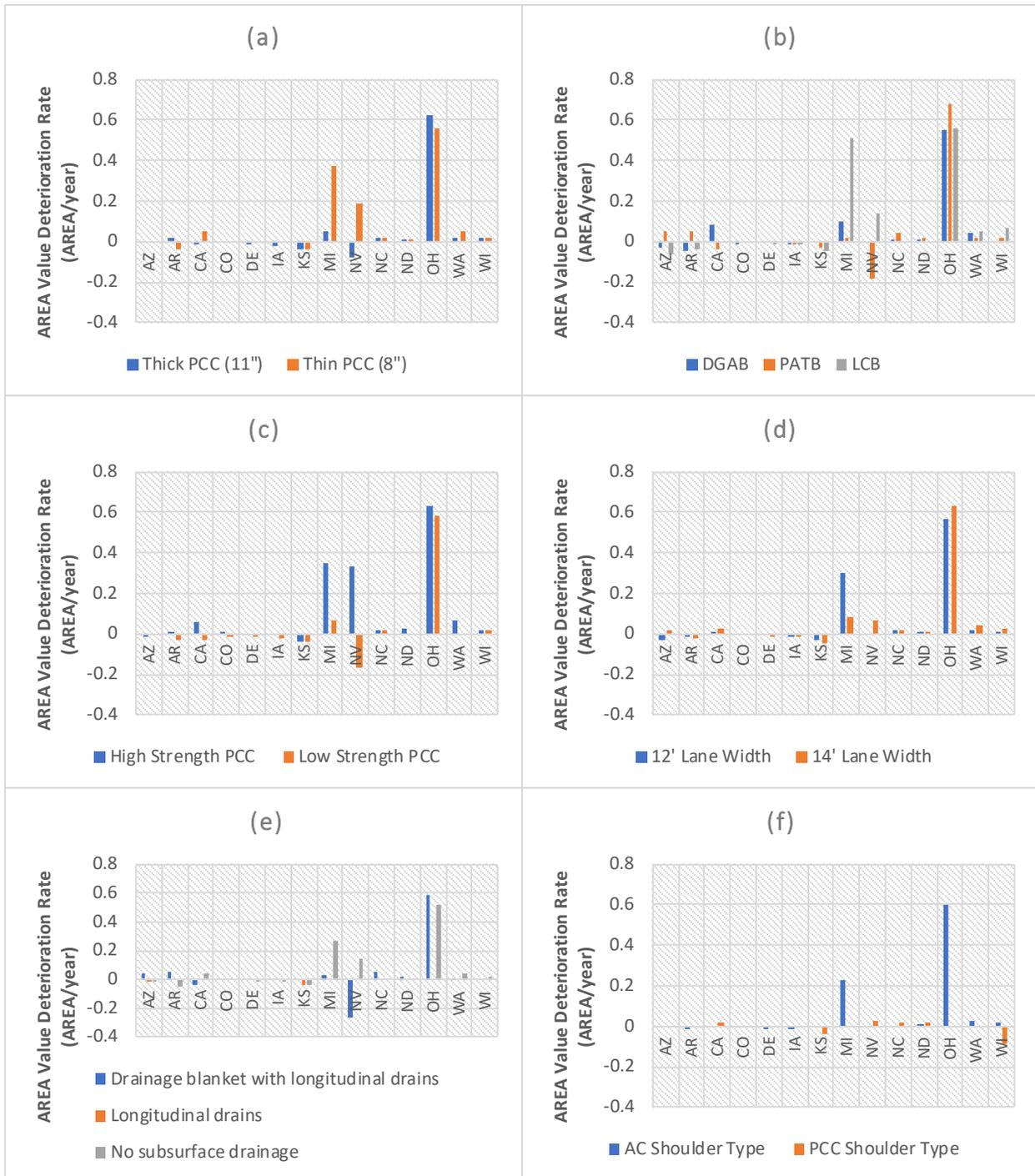
**Figure 30. Average Area Value by SPS-2 Project and Design Feature: (a) PCC thickness, (b) Base type, (c) PCC strength, (d) Lane width, (e) drainage feature, and (f) shoulder type.**
