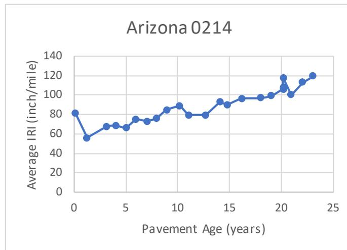
**Figure 19. Time Series of Mean IRI for Section 040214.**
