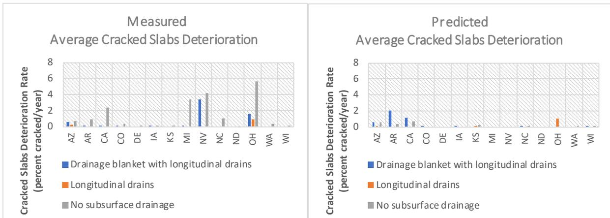
**Figure 15. Deterioration Rates for Measured and Predicted Transversely Cracked Slabs by Drainage Feature**
