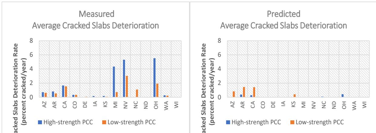
**Figure 9. Deterioration Rates for Measured and Predicted Transversely Cracked Slabs by PCC Design Strength**
