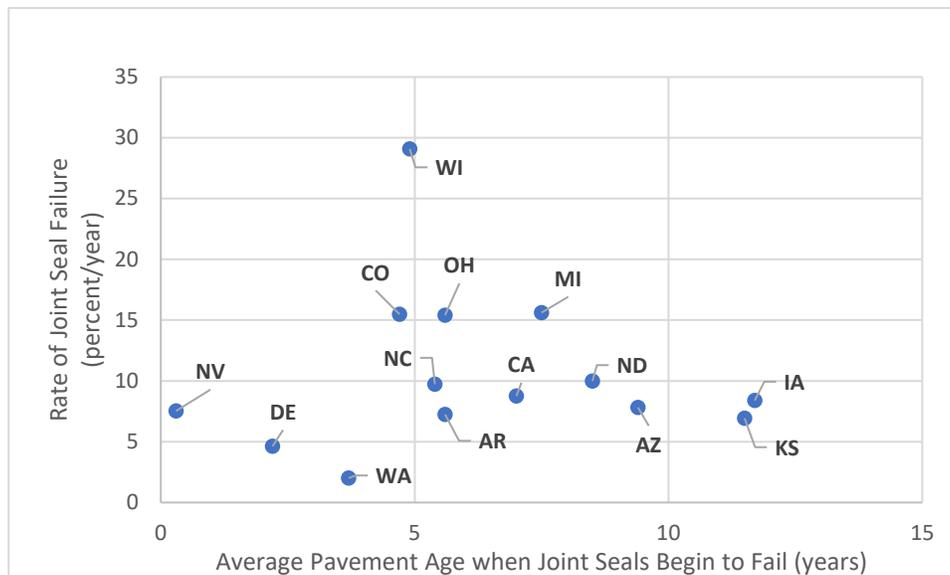
**Figure 32. Average Start and Rate Of Transverse Joint Seal Failure on SPS-2 Test Sections by State.**
