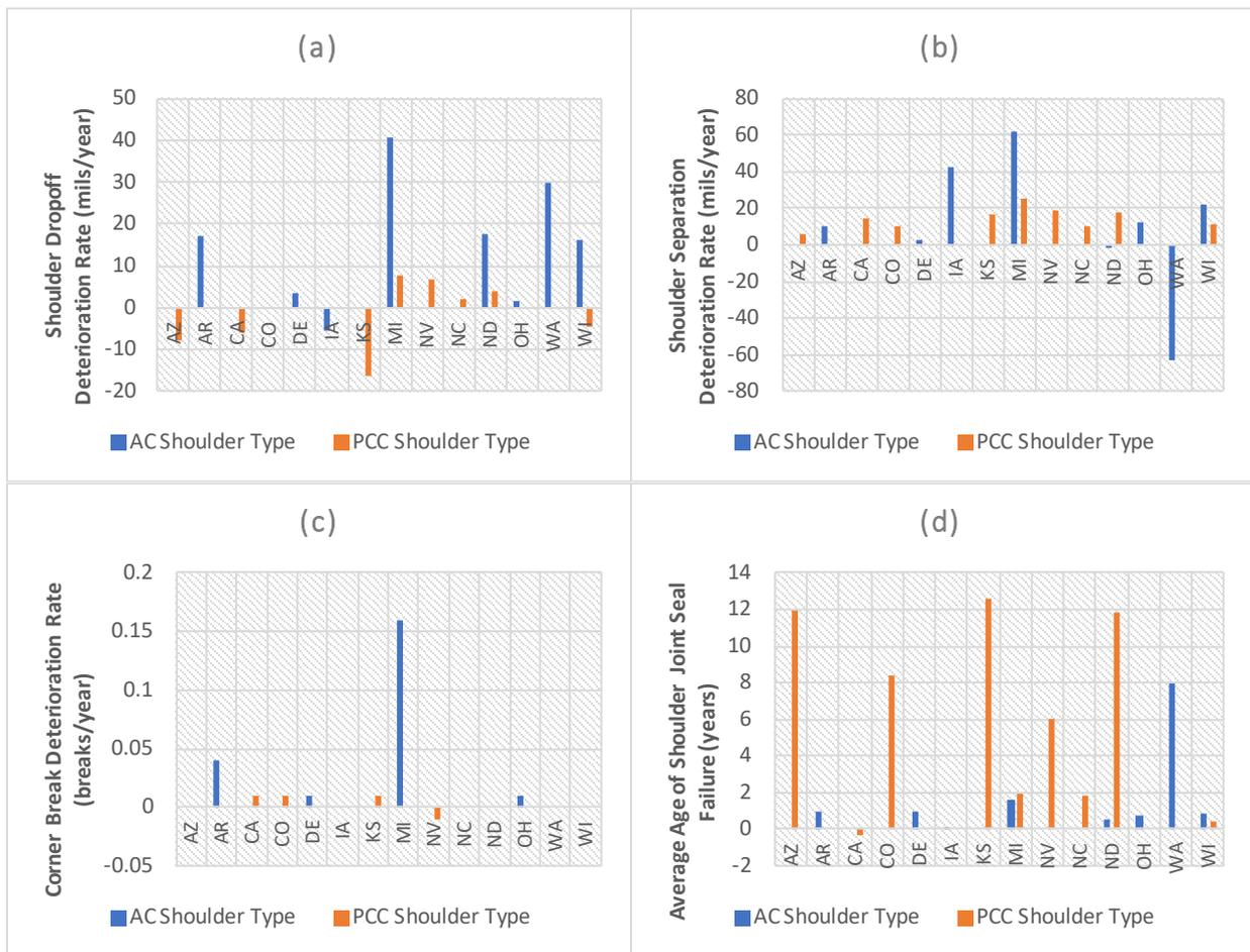
**Figure 24. Deterioration Rates for Shoulder Dropoff (a), Shoulder Separation (b), Corner Breaks (c), and the Average Age at Shoulder Joint Seal Failure (d) by Shoulder Type**
