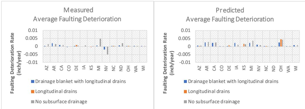
**Figure 14. Deterioration Rates for Measured and Predicted Faulting by Drainage Feature**
