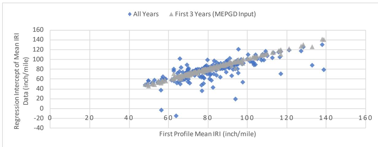
**Figure 17. Comparison of First Profile Mean IRI and the Linear Regression Intercept of Profile Data.**
