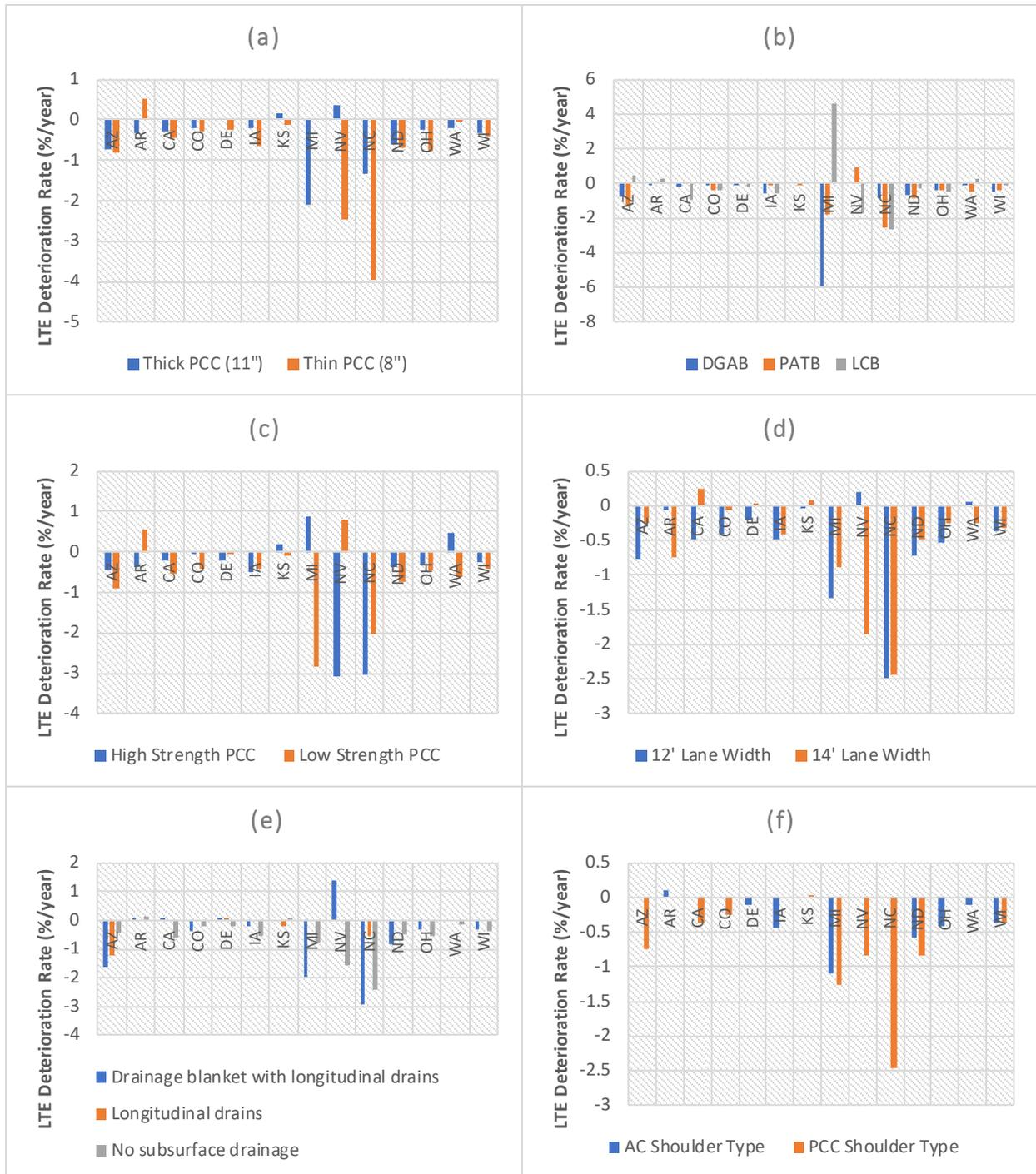
**Figure 28. Average Leave Slab LTE by SPS-2 Project and Design Feature: (a) PCC thickness, (b) Base type, (c) PCC strength, (d) Lane width, (e) drainage feature, and (f) shoulder type.**
