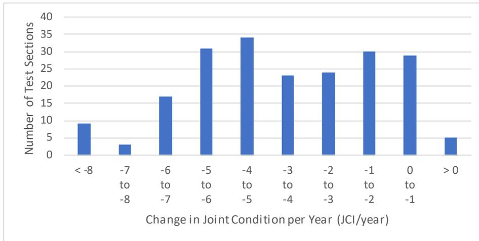
**Figure 35. Histogram of Transverse JCI Deterioration Rates**
