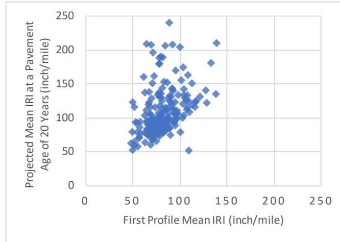
**Figure 20. Comparison of First Profile Mean IRI and the Projected IRI after 20 Years.**
