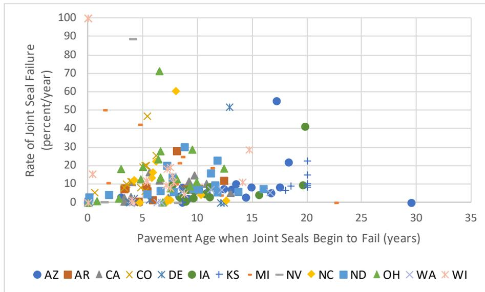
**Figure 31. Start and Rate of Joint Seal Failure on SPS-2 Core Test Sections.**
