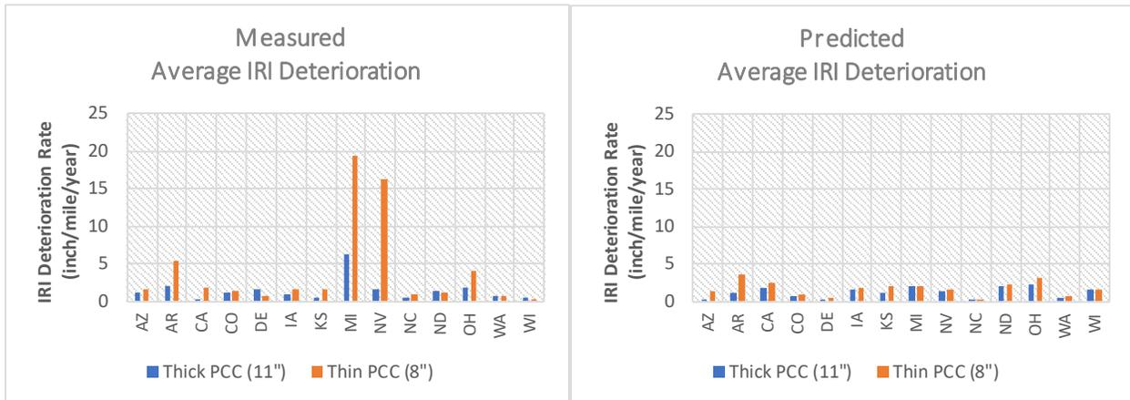
**Figure 1. Deterioration Rates for Measured and Predicted IRI by PCC Design Thickness**
