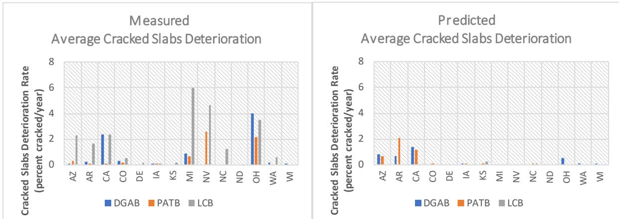
**Figure 6. Deterioration Rates for Measured and Predicted Transversely Cracked Slabs by Base Type**
