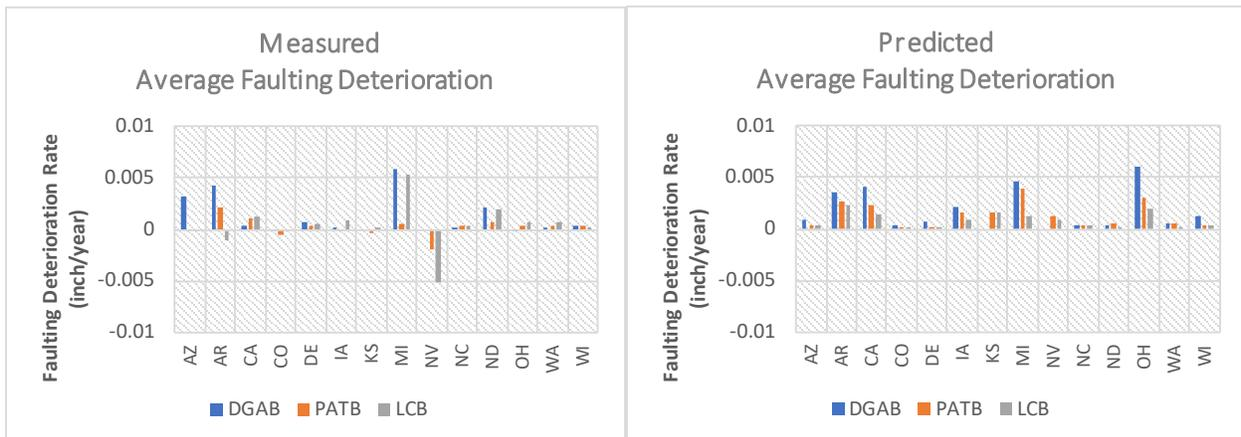
**Figure 5. Deterioration Rates for Measured and Predicted Faulting by Base Type**
