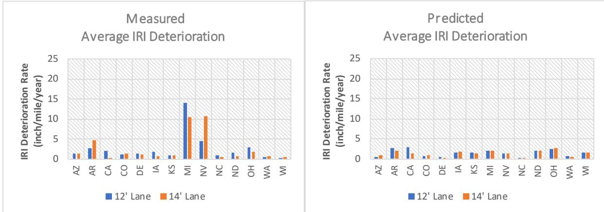
**Figure 10. Deterioration Rates for Measured and Predicted IRI by Lane Width**
