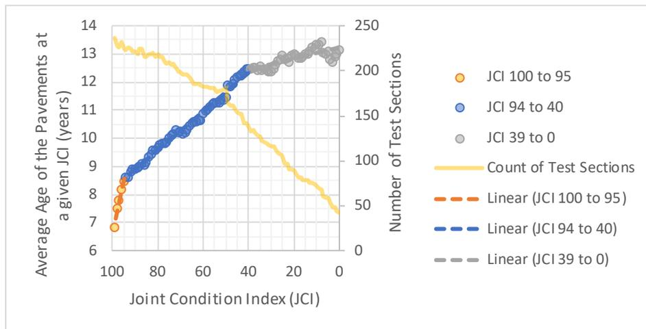
**Figure 36. Average Age of SPS-2 Test Sections by JCI**
