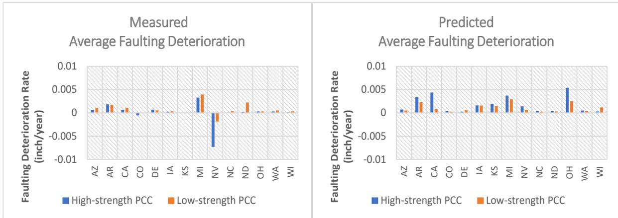
**Figure 8. Deterioration Rates for Measured and Predicted Faulting by PCC Design Strength**
