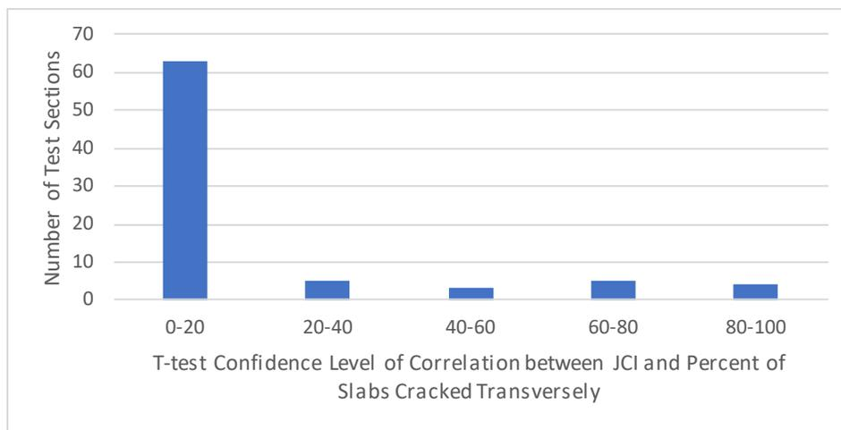
**Figure 37. Histogram of Confidence Level from T-test Between Joint Severity and Transversely Cracked Slabs**
