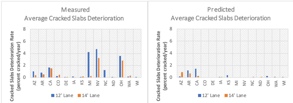
**Figure 12. Deterioration Rates for Measured and Predicted Transversely Cracked Slabs by Lane Width**
