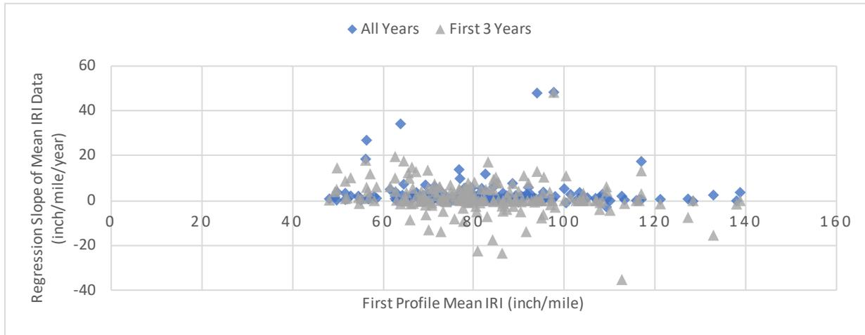
**Figure 18. Comparison of First Profile Mean IRI and the Linear Regression Slope of Profile Data (IRI Deterioration Rate).**
