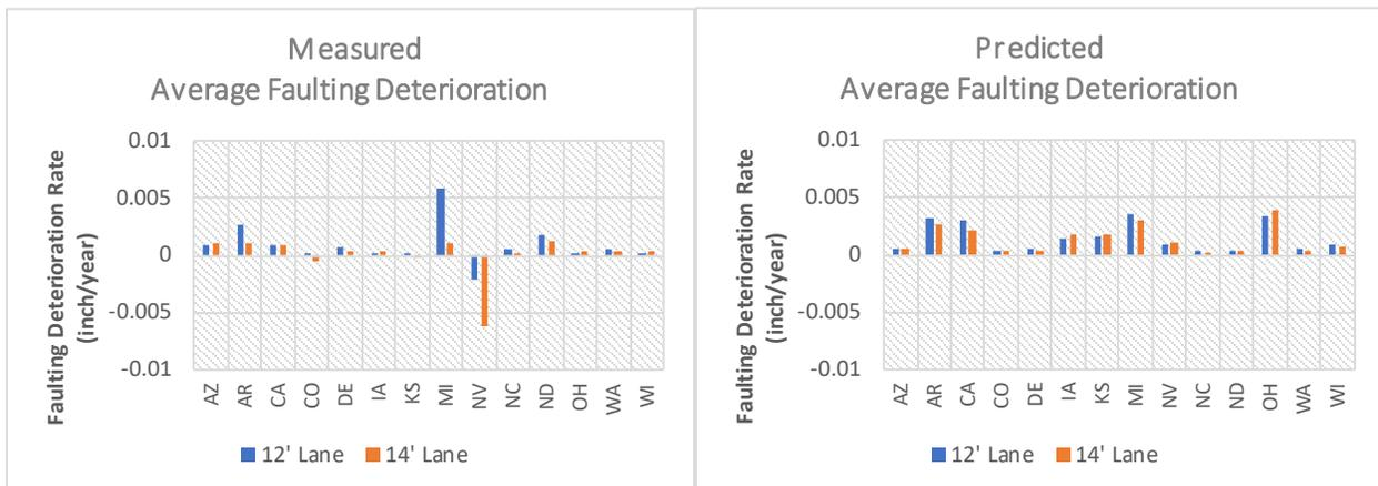
**Figure 11. Deterioration Rates for Measured and Predicted Faulting by Lane Width**
