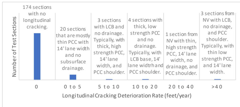
**Figure 25. Histogram of SPS-2 Test Sections by Bins Longitudinal Cracking Deterioration Rate**
