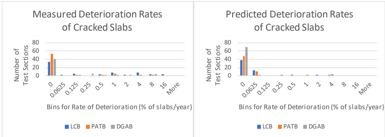
Figure 16. Histogram of Deterioration Rates for Transversely Cracked Slabs
