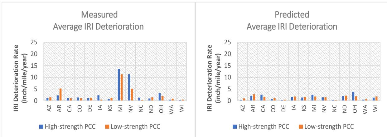
**Figure 7. Deterioration Rates for Measured and Predicted IRI by PCC Design Strength**
