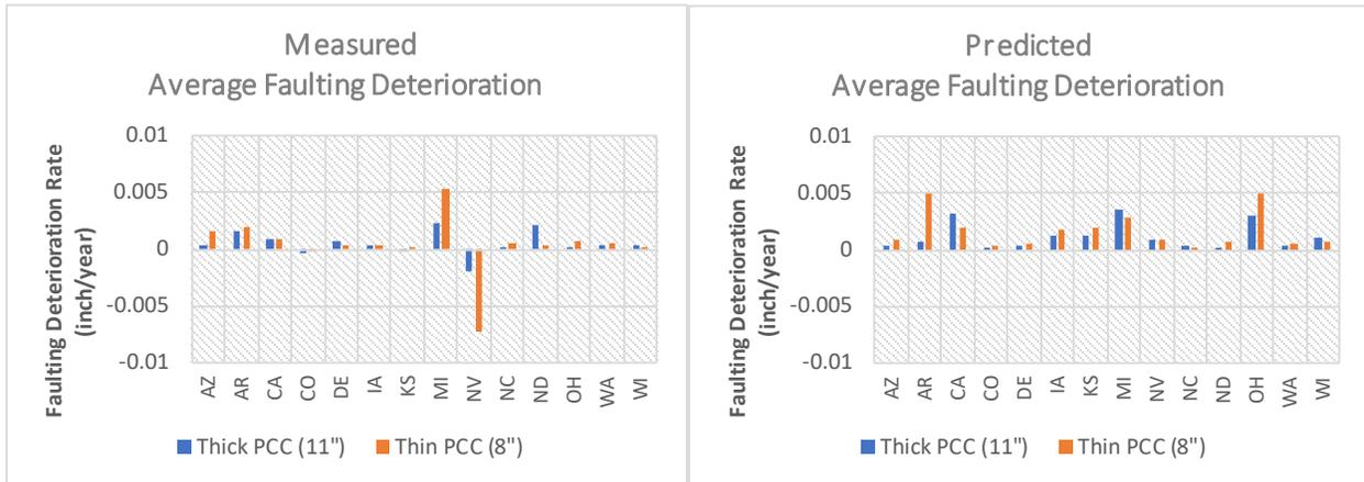
**Figure 2. Deterioration Rates for Measured and Predicted Faulting by PCC Design Thickness**
