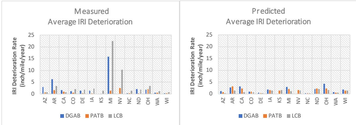
**Figure 4. Deterioration Rates for Measured and Predicted IRI by Base Type**
