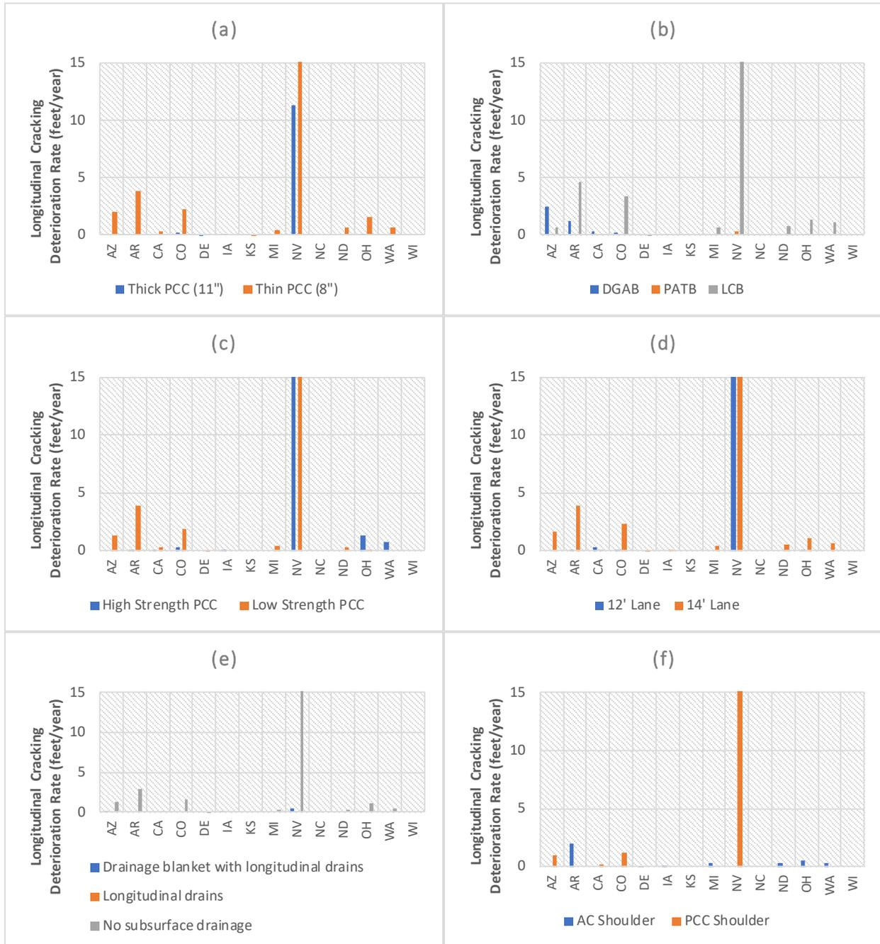
**Figure 26. Average Longitudinal Cracking by SPS-2 Project and Design Feature: (a) PCC Thickness, (b) Base Type, (c) PCC Strength, (d) Lane Width, (e) Drainage Feature, and (f) Shoulder Type.**
