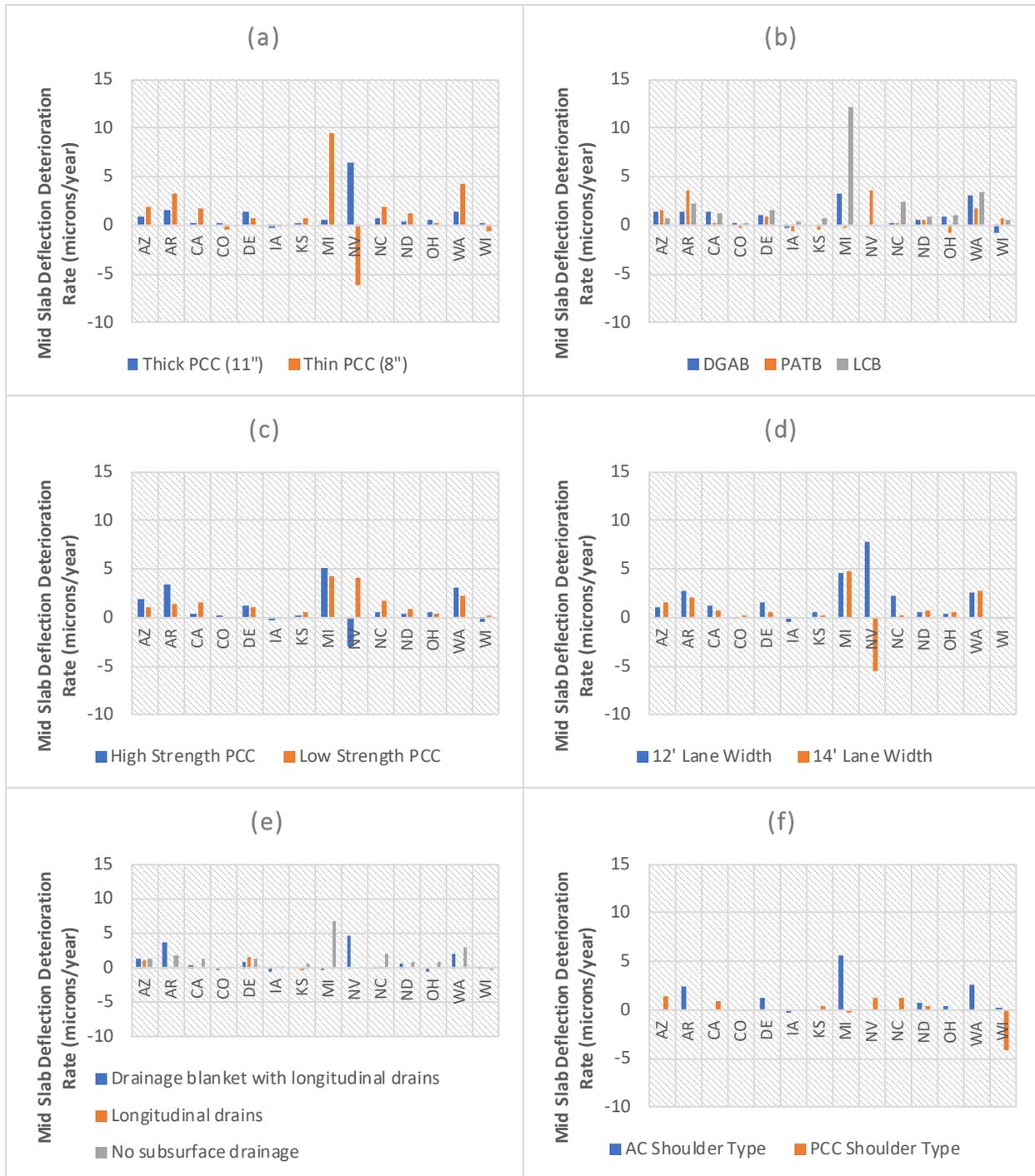
**Figure 29. Average Mid Slab Deflection by SPS-2 Project and Design Feature: (a) PCC Thickness, (b) Base Type, (c) PCC Strength, (d) Lane Width, (e) Drainage Feature, and (f) Shoulder Type.**
