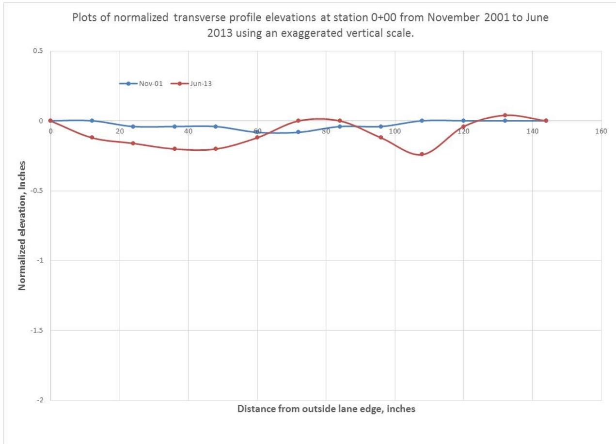
**Figure 12. Exaggerated vertical scale of the normalized transverse profile at station 0+00 after the mill and fill overlay placed in October 2001.**
