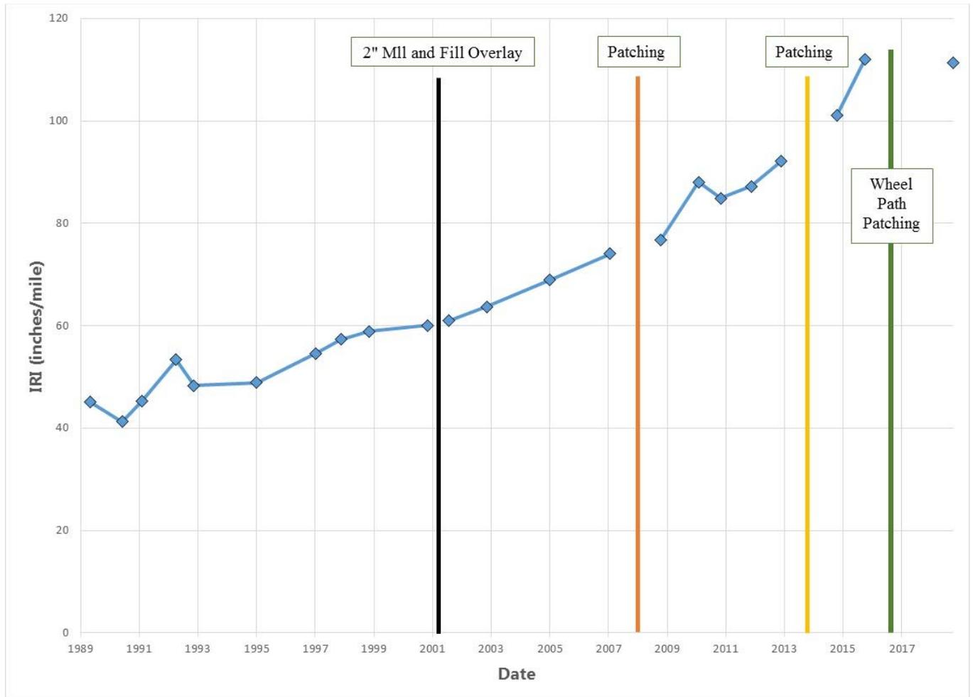
**Figure 24. Updated pavement roughness time-history adding the April 2019 LTPP measurement. The wheel path skin patches appear to arrest the further increase in roughness, within the time frame of these measurements.**
