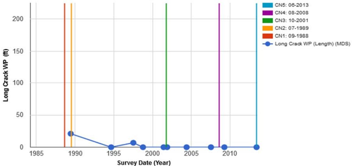
**Figure 6. Time history of longitudinal cracking in the wheel path.**
