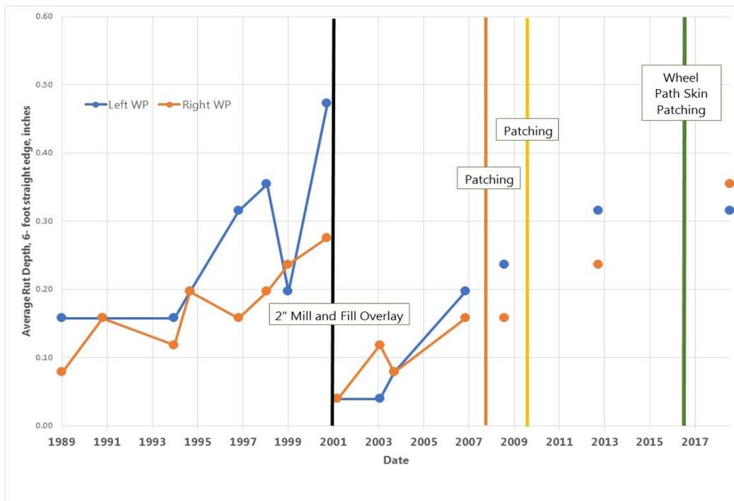
**Figure 27. Time history plot of average rut depths in left and right wheel paths based on the 6-foot straight edge measurement method.**
