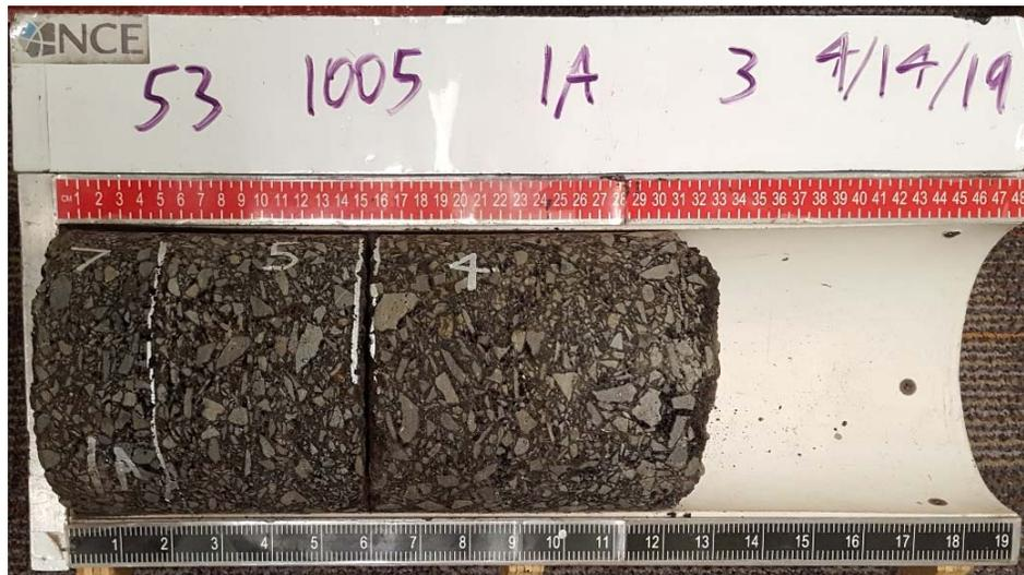
**Figure 13.** Image of core 1A obtained at station 200 at an offset of 0.8 feet from the outside lane edge.
