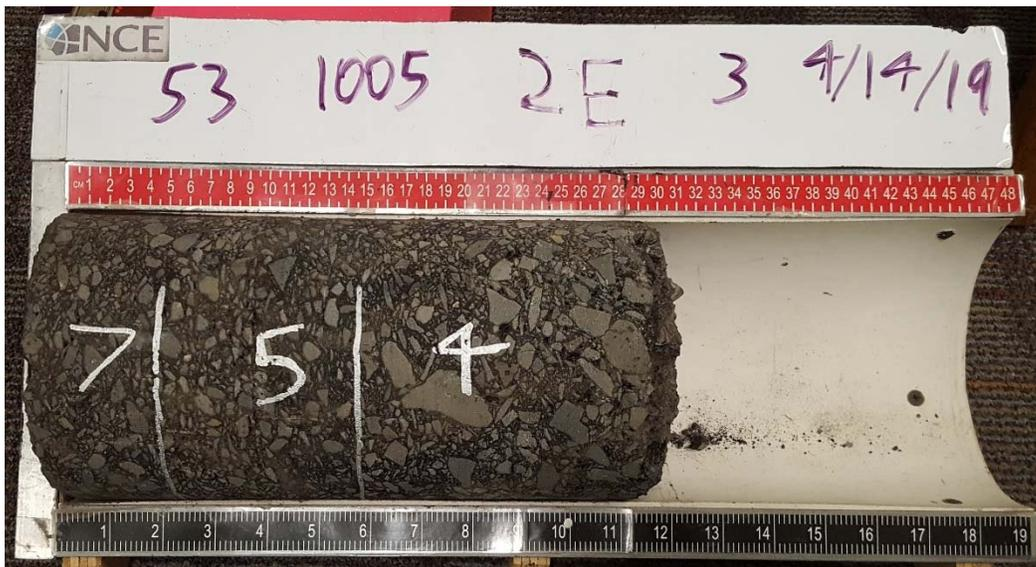
Figure 23. Image of core 2E, from station 400 with an offset of 13 feet.
