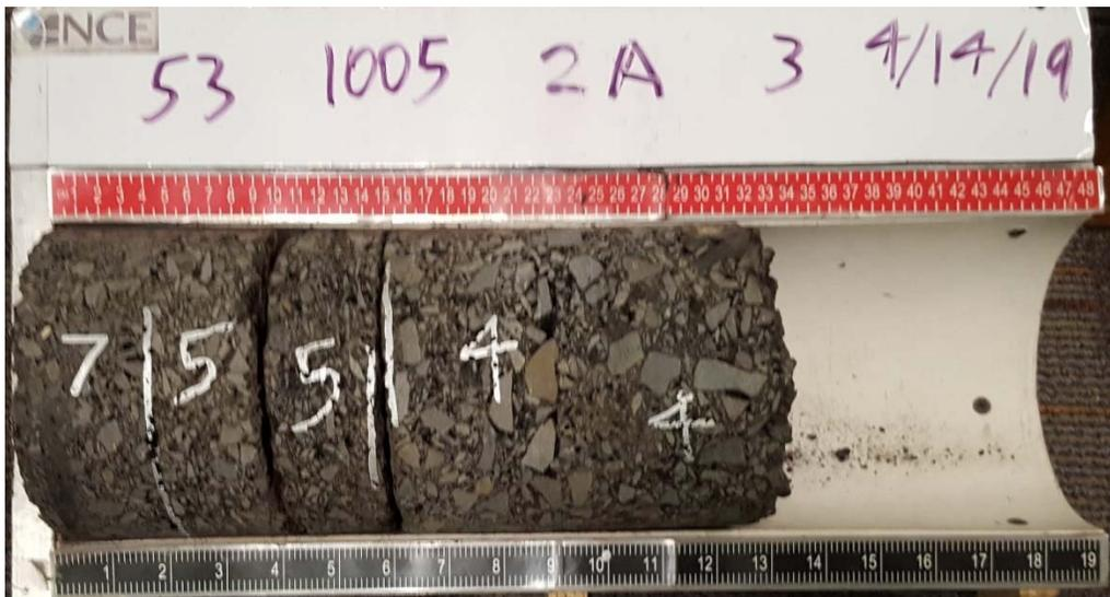
**Figure 19. Image of core 2A obtained from station 400 with an offset of 0.7 feet.**
