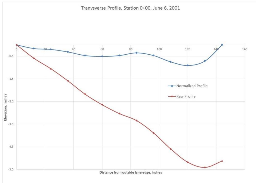
**Figure 10. Normalized and raw transverse pavement profile at station 0+00 performed on June 6, 2001 prior to the mill and fill construction event.**
