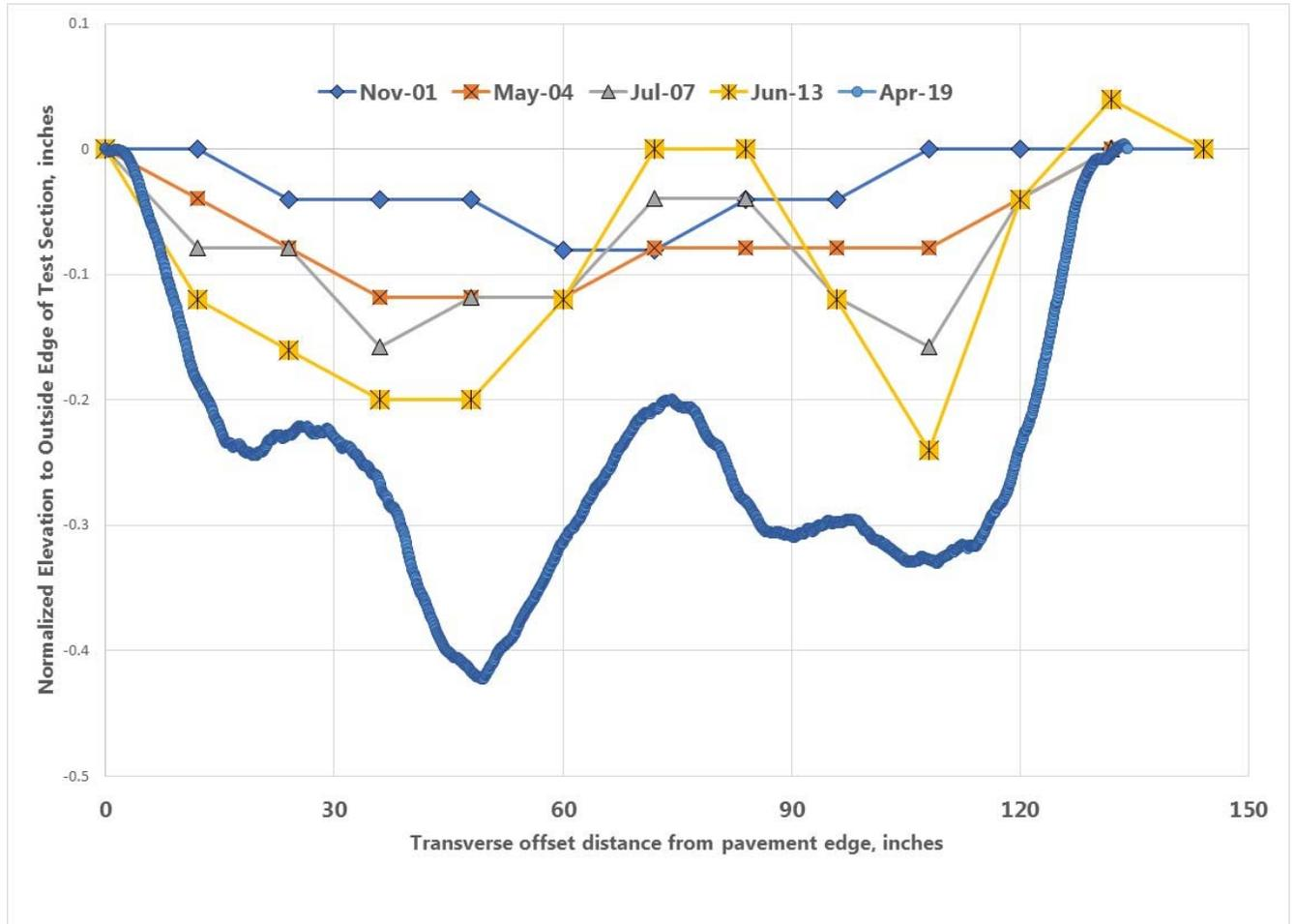
**Fig 26. Comparison of historic normalized transverse profile plots at station 0+00 on section 53\_1005.**
