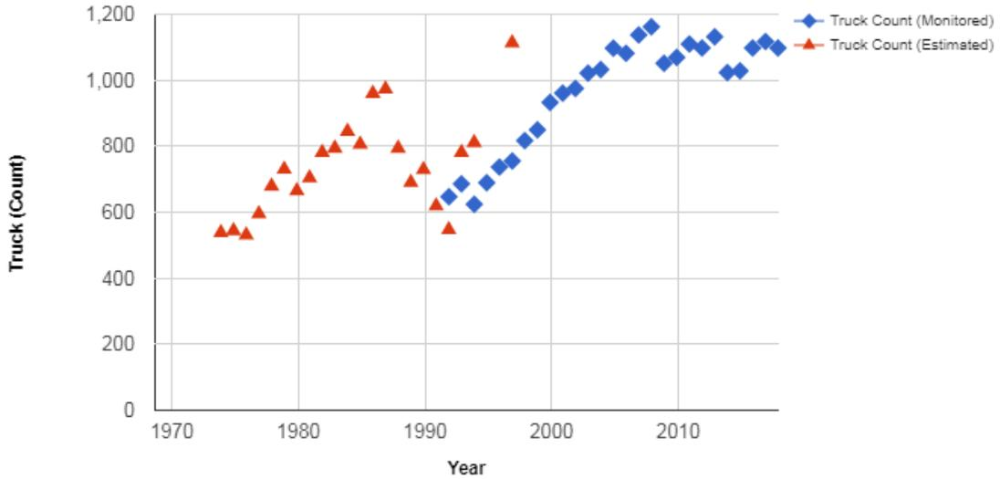
**Figure 3. Average annual daily truck traffic on test section 531005 based on state supplied estimates and monitoring measurements.**
