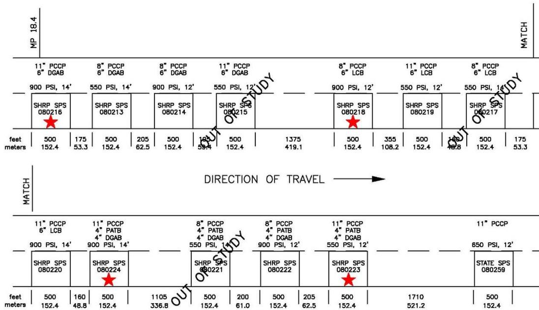
Figure 2. Location of selected test sections within the Colorado SPS-2 project.
