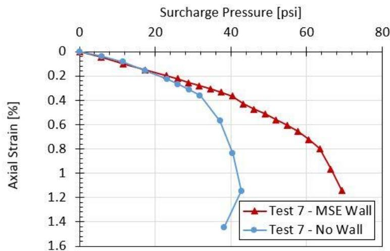
**Figure 7: Applied surcharge pressure versus axial strain in the LCC for tests with and without MSE wall.**
