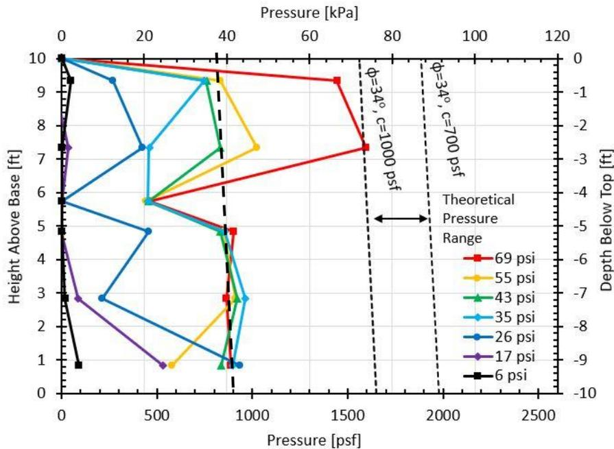
**Figure 11: Horizontal pressure on the welded-wire MSE wall versus depth curves for selected applied surcharge pressure values near the wall during test 7 as measured by Geokon pressure plates.**
