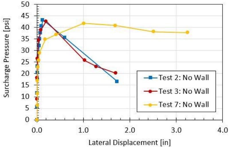
**Figure 10: Applied surcharge pressure vs. lateral wall displacement with no retaining wall (free face) for unreinforced LCC tests 2, 3, and 7.**
