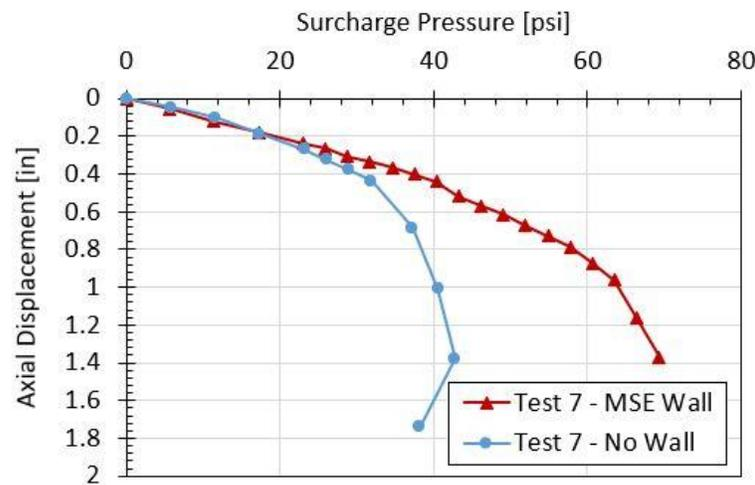
**Figure 6: Applied surcharge pressure versus axial displacement in the LCC for tests with and without MSE wall.**
