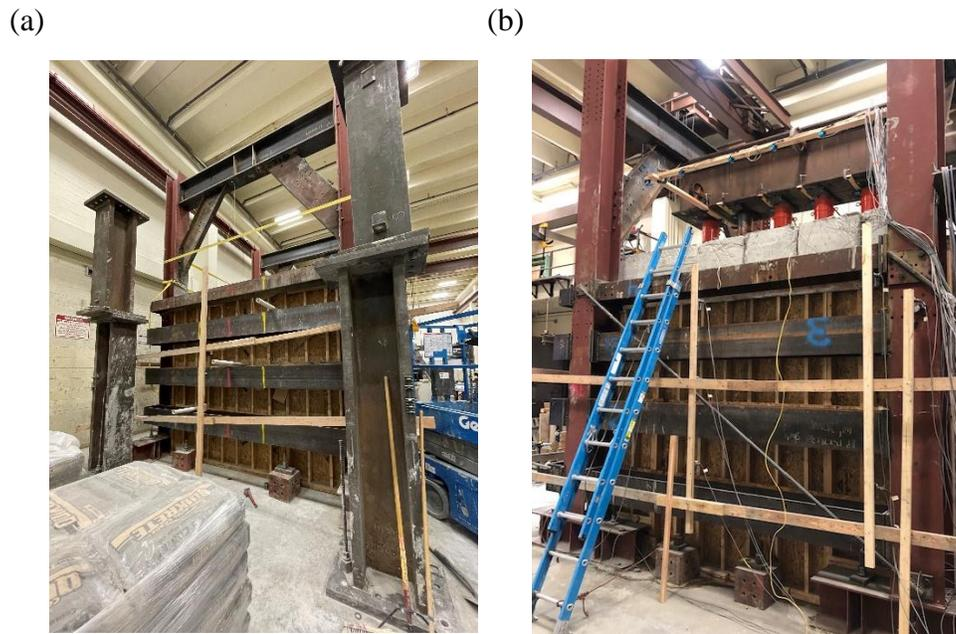
**Figure 4: Photographs showing: (a) the test box from the short side opposite from the retaining wall and (b) the test box from the long side with the concrete surcharge blocks and hydraulic jacks reacting against a longitudinal beam consisting of two deep beams.**
