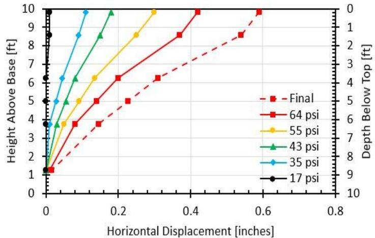
**Figure 12: (a) photograph of MSE wall panel deflection at failure, and (b) measured horizontal deflection of the wall versus height above the base of the wall for selected surcharge pressures.**
