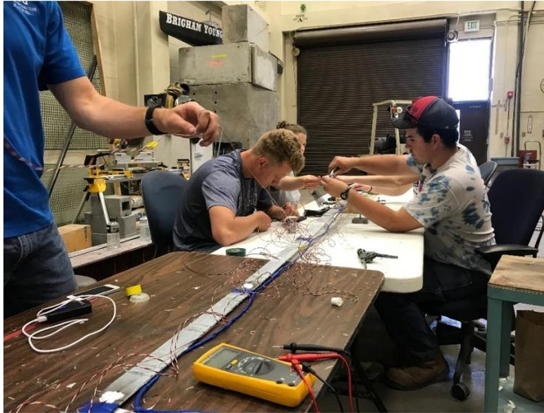
**Figure 2-4. Instrumentation of a ribbed strip reinforcement**
