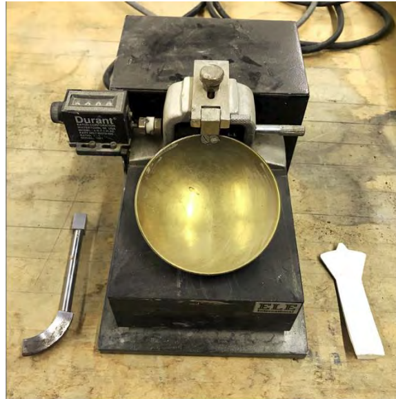
Figure 3. Liquid limit test device used in this study
