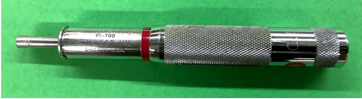
Figure 6. Pocket penetrometer device for this study
