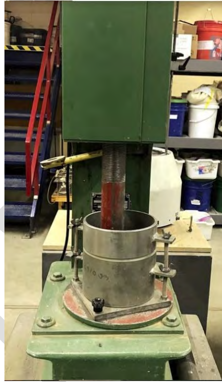
Figure 4. (a) Hobart mixer and (b) automated mechanical rammer used in this study
