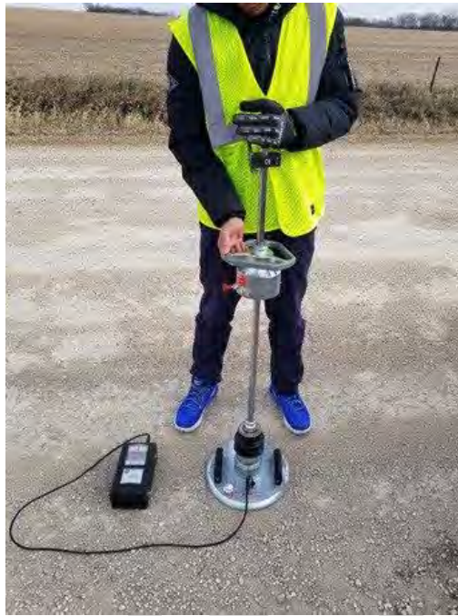
Figure 12. Light Weight Deflectometer device for this study
