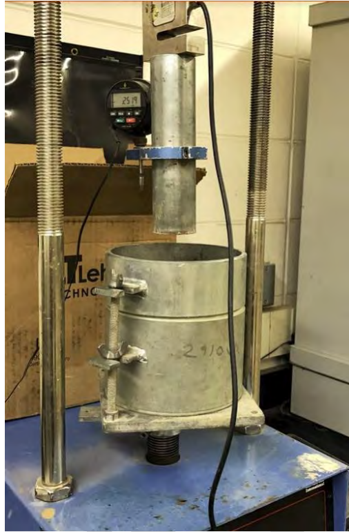
Figure 5. California Bearing Ratio device for this study
