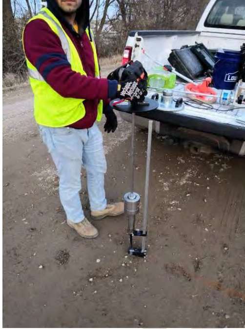
Figure 13. Dynamic Cone Penetrometer device for this study
