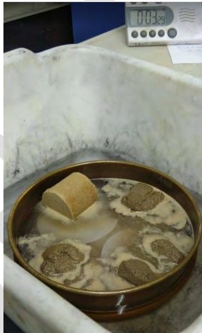
Figure 23. Slaking test for 2-by-2 specimens of Boone County existing surface aggregate, and mixing with 2% Clay Slurry
