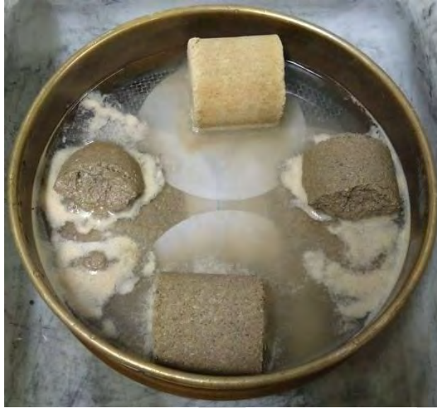
Figure 9. Slaking test for 2-by-2 specimens of Jones County existing surface aggregate mixing with 2% clay slurry, 2, 6, and 10% Moscow
