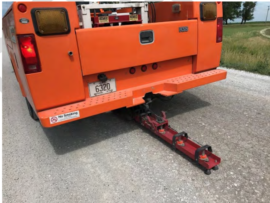
Figure 11. FWD device for this study
