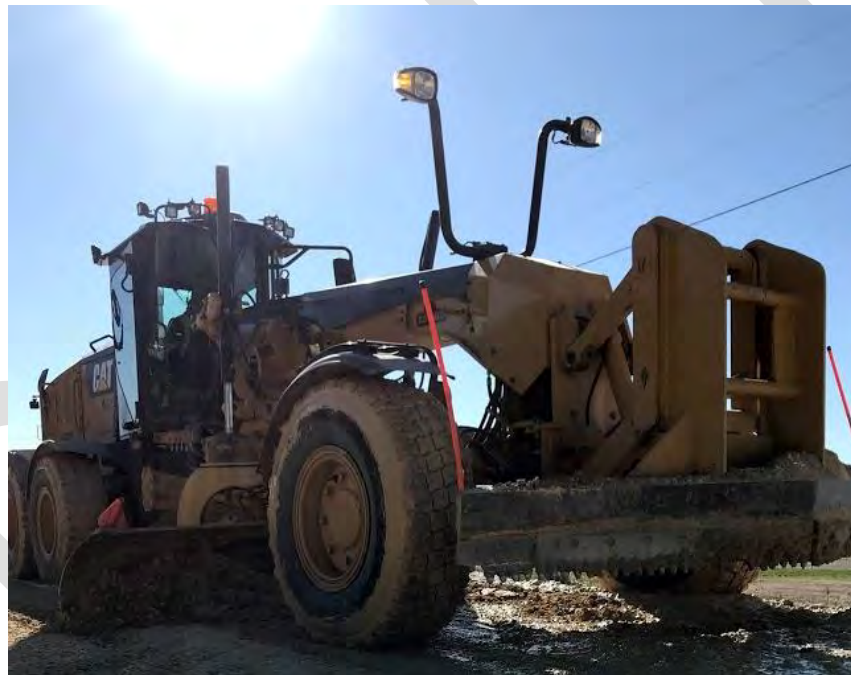
Figure 33. Motor grader for blading and removing the distresses
