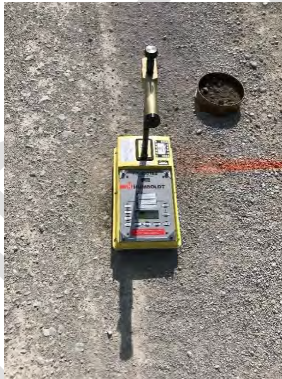
Figure 16. Nuclear Density Gauge test device (Cetin et al. 2019)
