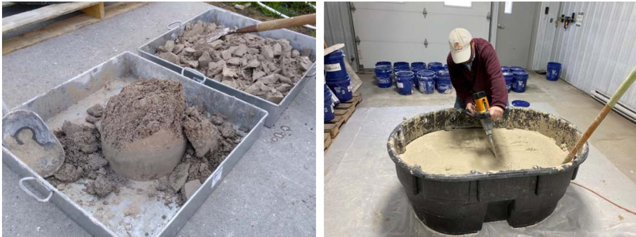
Figure 4: Typical CGR Cakes and CGR Slurry Mixing Process
