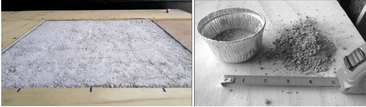
Figure 40: Soil Loss Due to Wind Erosion from Compacted Soil Form
