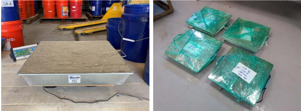
Figure 38: : Weighing and Curing of (Sealed) Compaction Soil Forms
