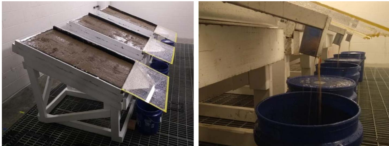
Figure 21: Typical Rainfall Simulation and Captured Sediment-Laden Water Runoff
