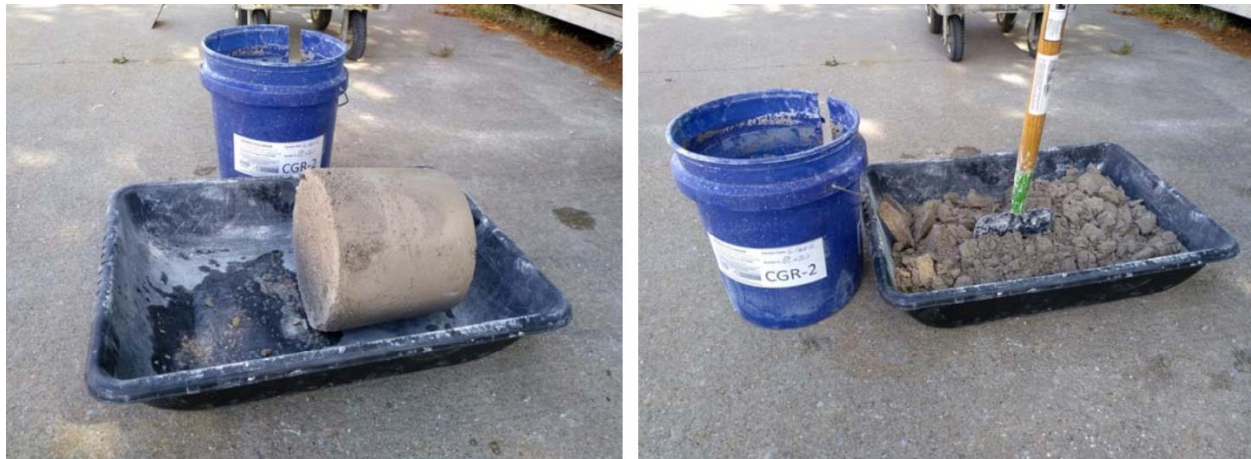
Figure 30: Consolidation of CGR Slurry After Storage for Extended Period of Time
