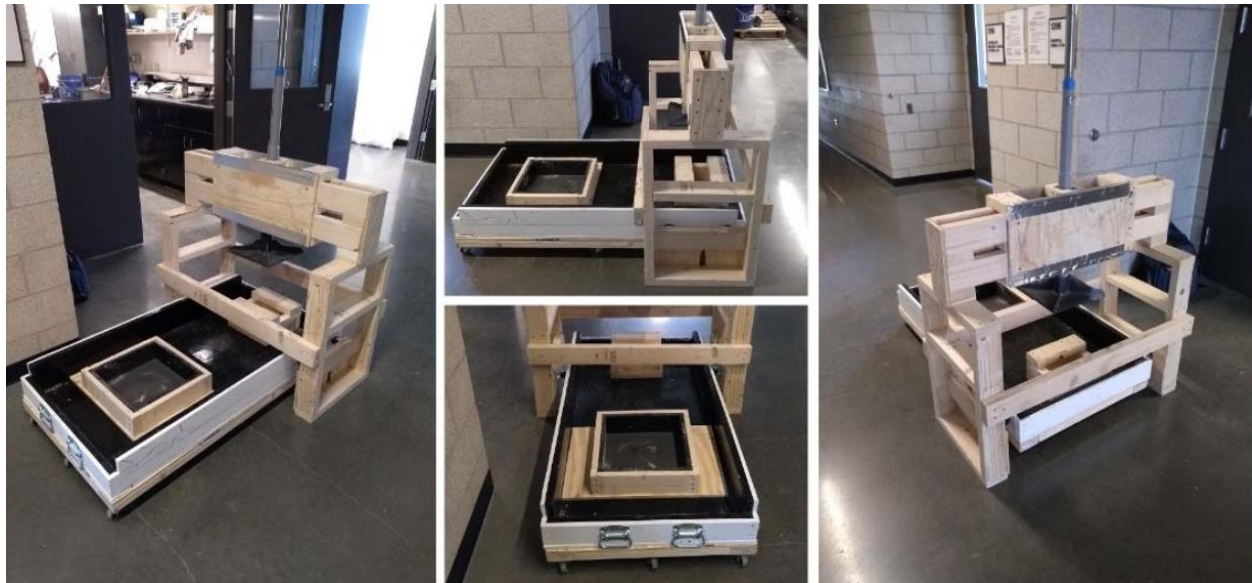
Figure 12: Wooden Uniform Tamping Apparatus (UTA)
