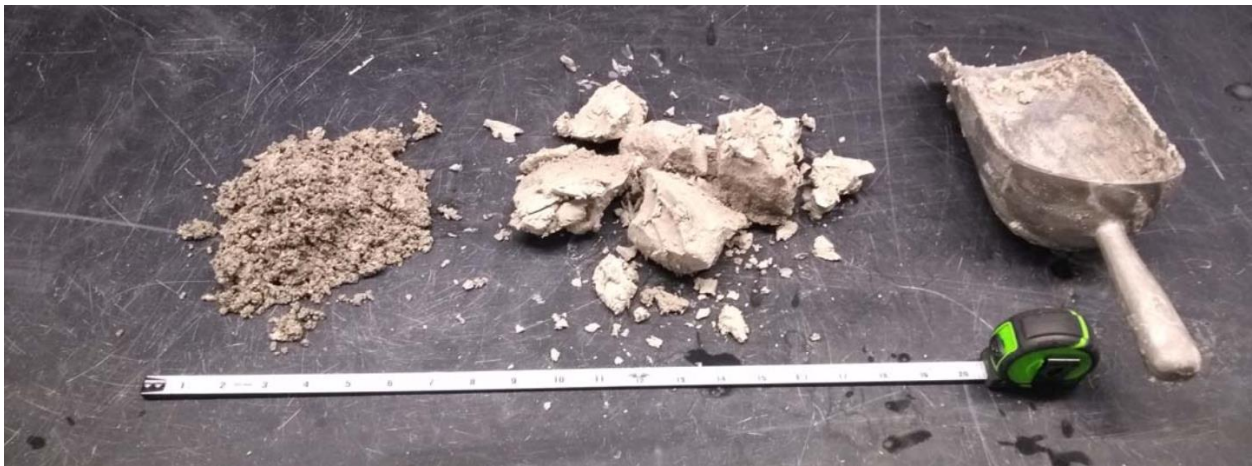
Figure 3: Consistency of Typical Settled CGR Solids (After Decanting)
