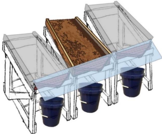
Figure 10: Concept Design Sketch and Completed (Built) Version of Rainfall Test Apparatus
