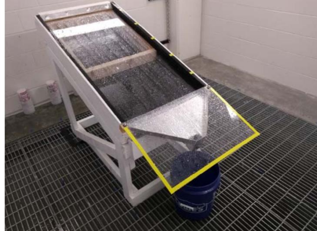
Figure 10: Concept Design Sketch and Completed (Built) Version of Rainfall Test Apparatus
