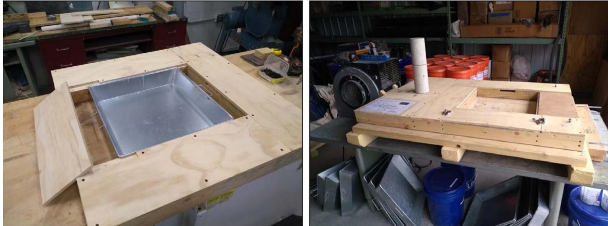
Figure 34: Wind Erosion Test Apparatus (WETA) During Fabrication and Final Construction
