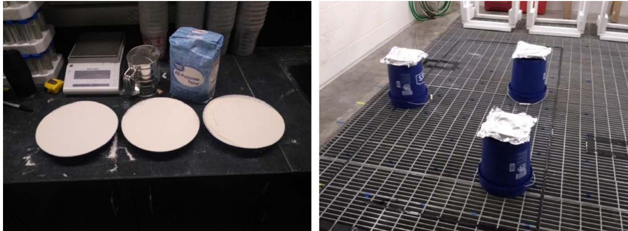
Figure 19: Raindrop Particle Size Distribution Test (Flour Test)
