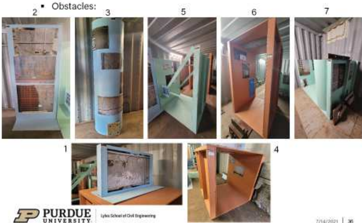
Figure 1 - Photographs showing interior UAV Evaluation Chamber
