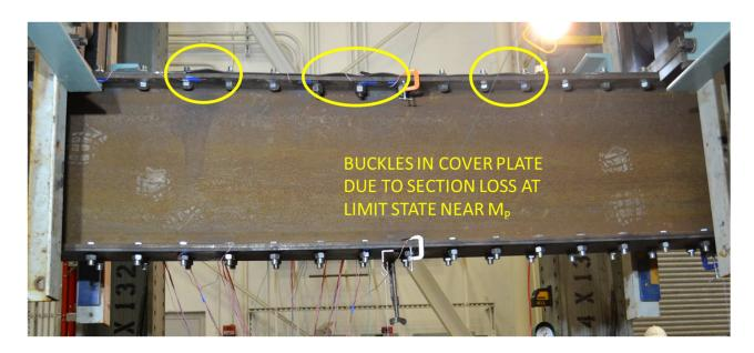
Figure 1 – Photograph of Specimens 2. Coverplate included simulated section loss but no simulated pack-out. Buckles in the coverplate were due to applied flexural compressive stress in the top flange.
