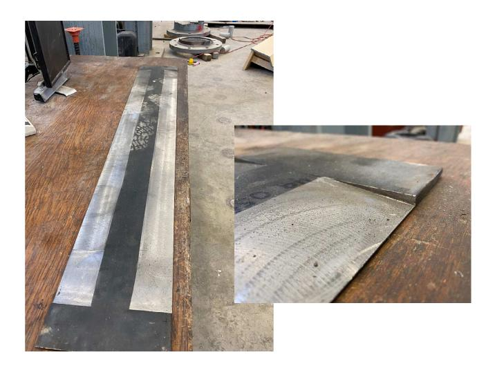
Figure 3 – Photograph of portion of coverplate in which edges are machined away to simulate section loss. The plate was originally 3/8 inches thick and is machined down to 1/8 inch at tips. Middle third is full thickness of 3/8 inch. Extension plates are then CJP welded onto each end so that the plate will run full length of the specimens.
