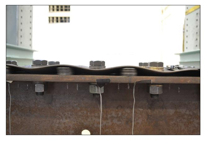
Figure 2 – Photographs of Specimen 3 showing simulated pack-out distortion and section loss. There was no load applied when this photograph was taken.
