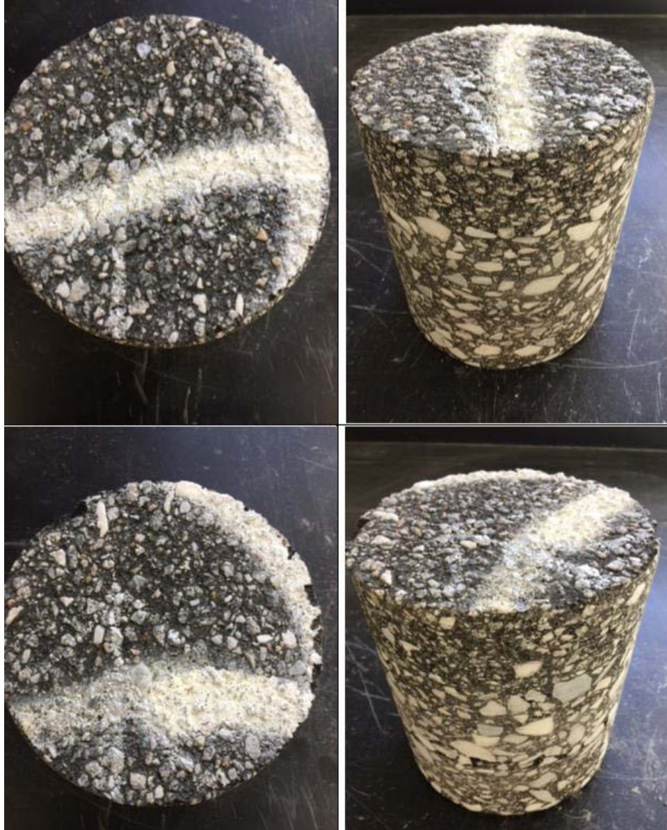
Figure 5 Cores Taken from Section N5 (Control, Low Density, Low AC)
