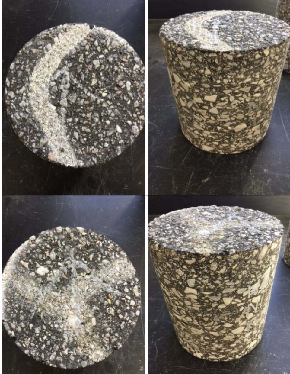
Figure 3 Cores Taken from Section N1 (Control, 20% RAP)
