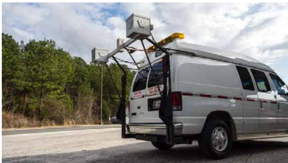
Figure 9 Inertial Profiler Used to Assess Ride Quality and Rutting Measurement
