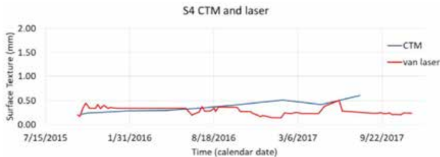
Figure 7 Field Surface Macrotexture Measurements
