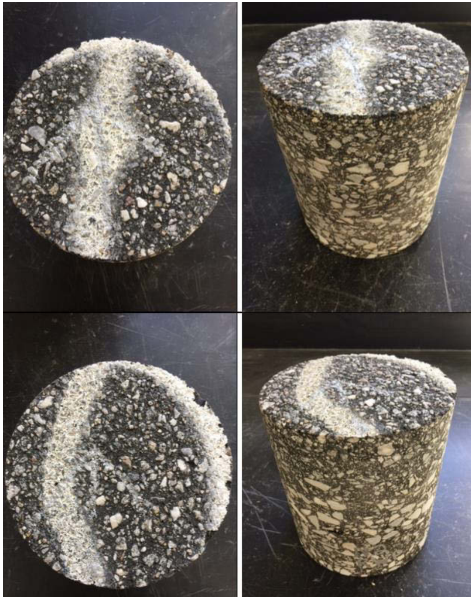
Figure 4 Cores Taken from Section N2 (Control, Higher Density)
