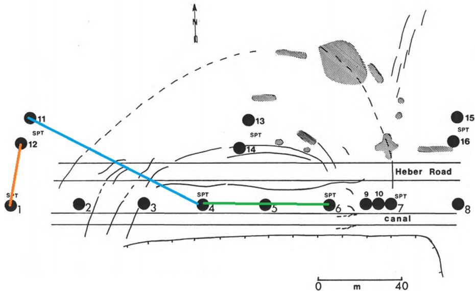
Figure 1 SPT boreholes and lateral spread in Heber road at 1979 Imperial Valley case history
