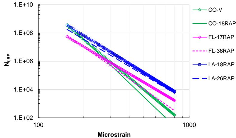
Given the unparallel failure lines and the need for a parameter for indicating the fatigue resistance, the fatigue life corresponding to 340 microstrain was interpolated for each mixture and was denoted as  $N_{f,BF}$ . This strain level was the average of the strains at the bottom of the ALF lanes obtained using the finite element analysis; see Table 6 in a later
