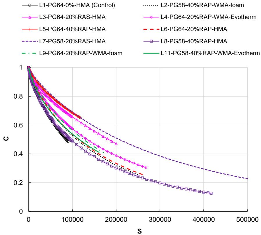
**Figure 9. Damage characteristic curves of the CO, FL, and LA mixtures**
