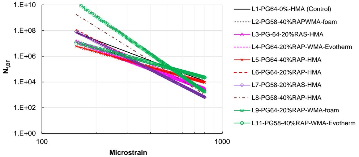
**Figure 15. Relationship of fatigue life  $N_{f,BF}$  versus strain level for the CO, FL, and LA mixtures**
