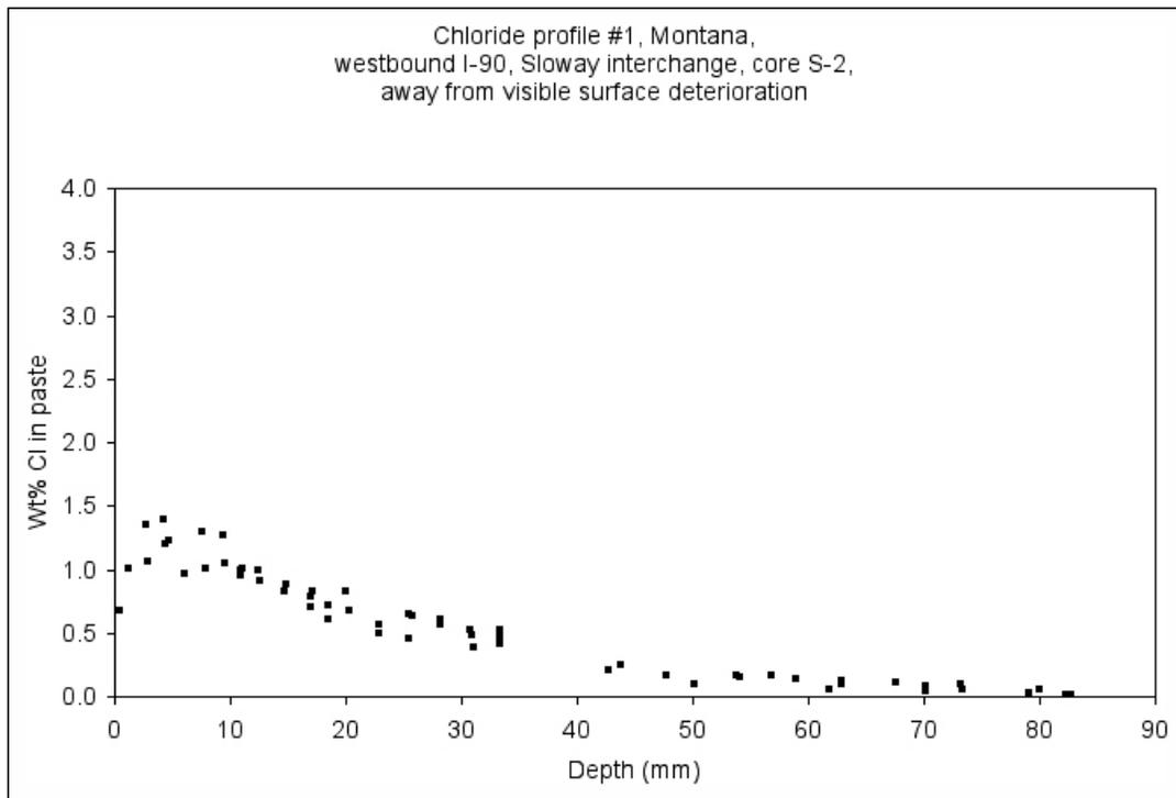
Figure S-10: Chloride profile through cement paste, from billet prepared from core S-2.
