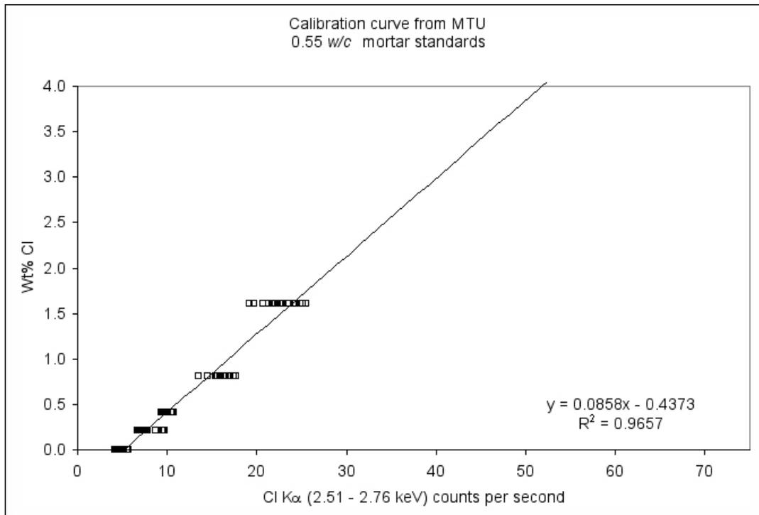
Figure B-1: Calibration curve plotting CI Ka counts per second versus wt% Cl from cement paste of 0.55 w/c mortar standards.
