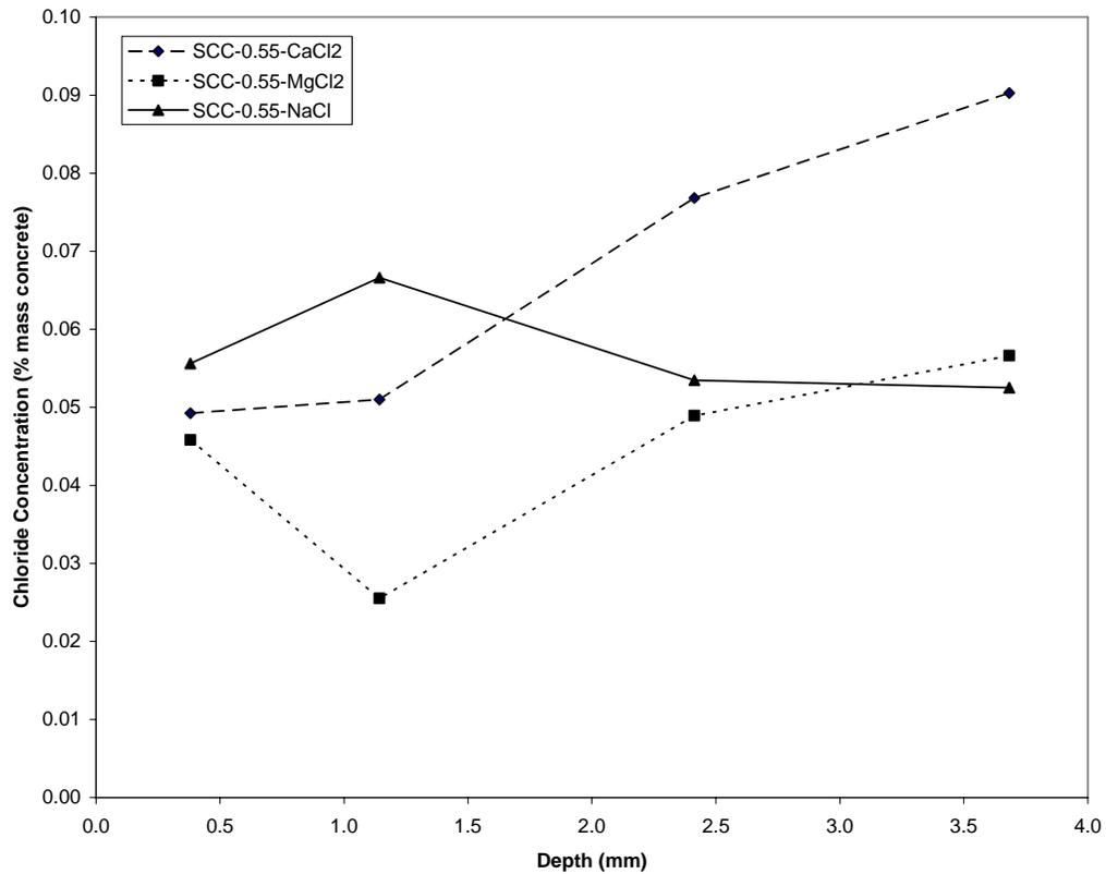
Figure 9. GGBFS blended cement concrete samples (sealer 1) - chloride profile
