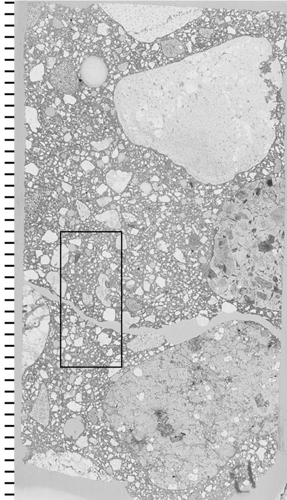
Figure T-14: Transmitted light scanned image of thin section to show location of elemental map. The large crack, sub-parallel to the pavement surface, is at a depth of about 40 mm, (tic marks every mm).
