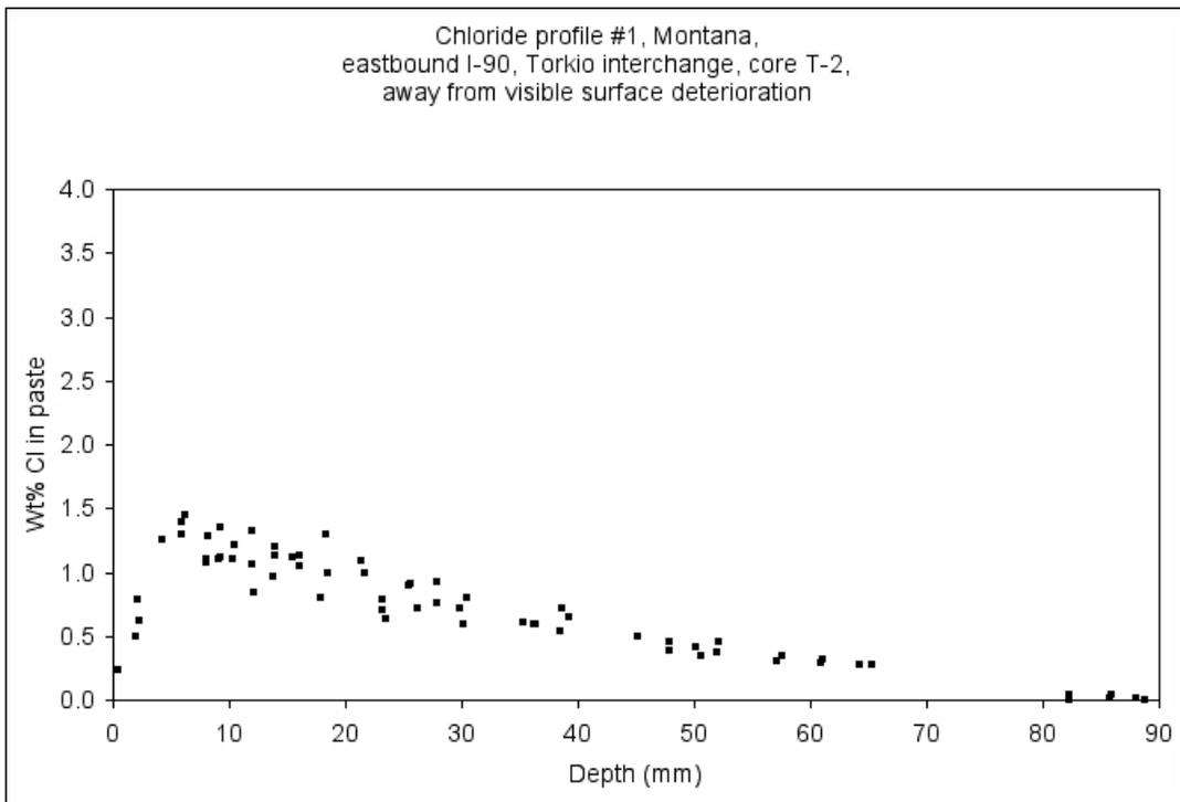
Figure T-10: Chloride profile through cement paste, from billet prepared from core T-2.
