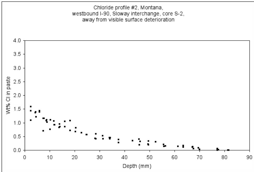
Figure S-11: Chloride profile through cement paste, from billet prepared from core S-2.
