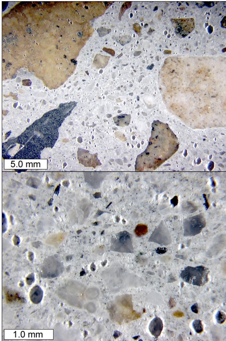
Figure CO-9: Stereo microscope images to show air void structure on polished slab from core CO-1.
