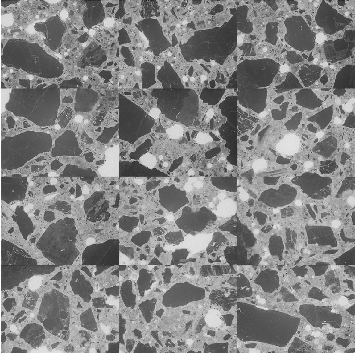
Figure CO-11: Mosaic of 12 frames collected from thin section prepared from billet cut from top portion of core CO-6 (each individual frame measures 2.612 x 1.959 mm).
