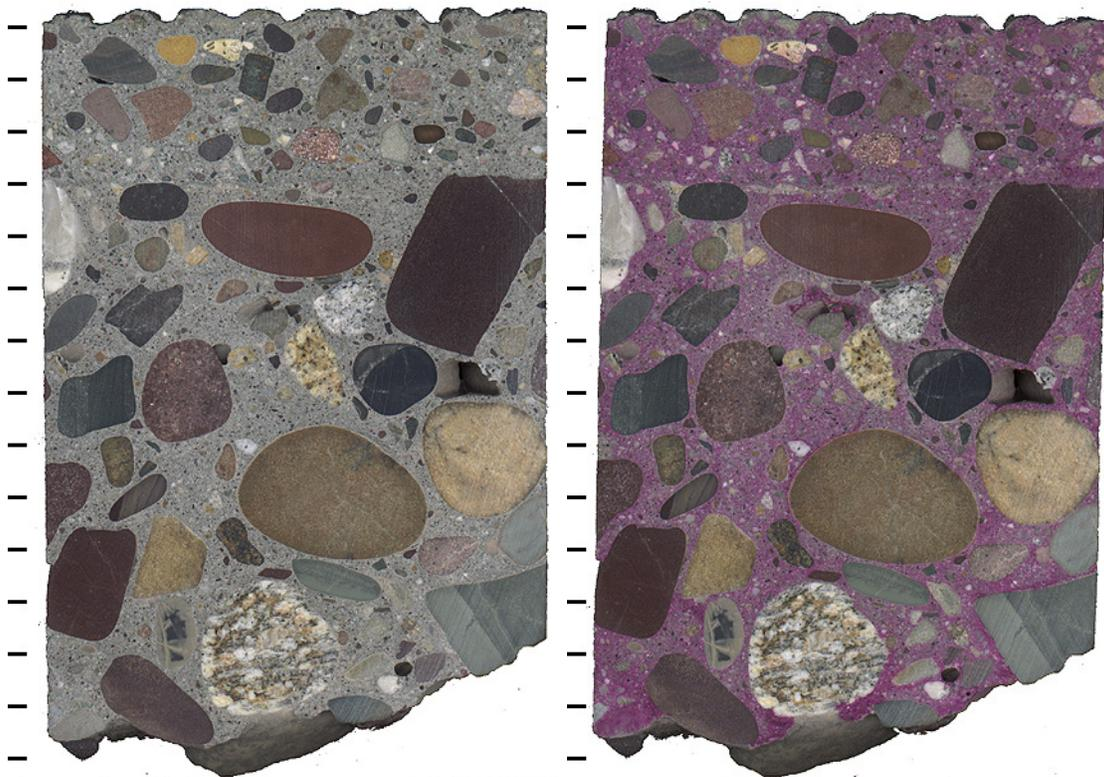
Figure MT-4: Polished slabs to show complete cross-section through core MT-2 both before (left) and after application of phenolphthalein stain (right) tic marks every cm.
