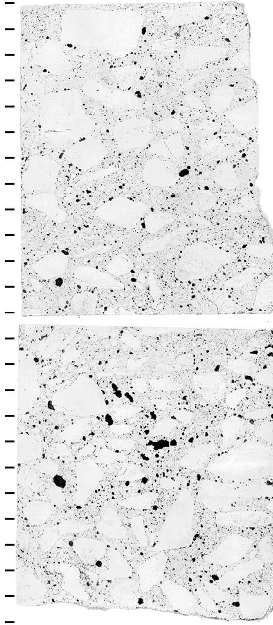
Figure CO-6: Polished slabs to show complete cross-section through core CO-1 after treatment to enhance appearance of air voids and cracks, tic marks every cm.
