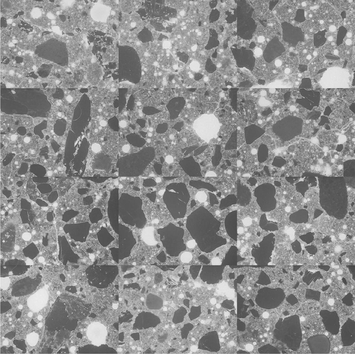
Figure SD-13: Mosaic of 12 frames collected from thin section prepared from a second billet cut from top portion of core SD-1 (each individual frame measures 2.612 x 1.959 mm). These frames were not masked and used for w/c determination, but recorded as visual check against the first section prepared from core SD-1.
