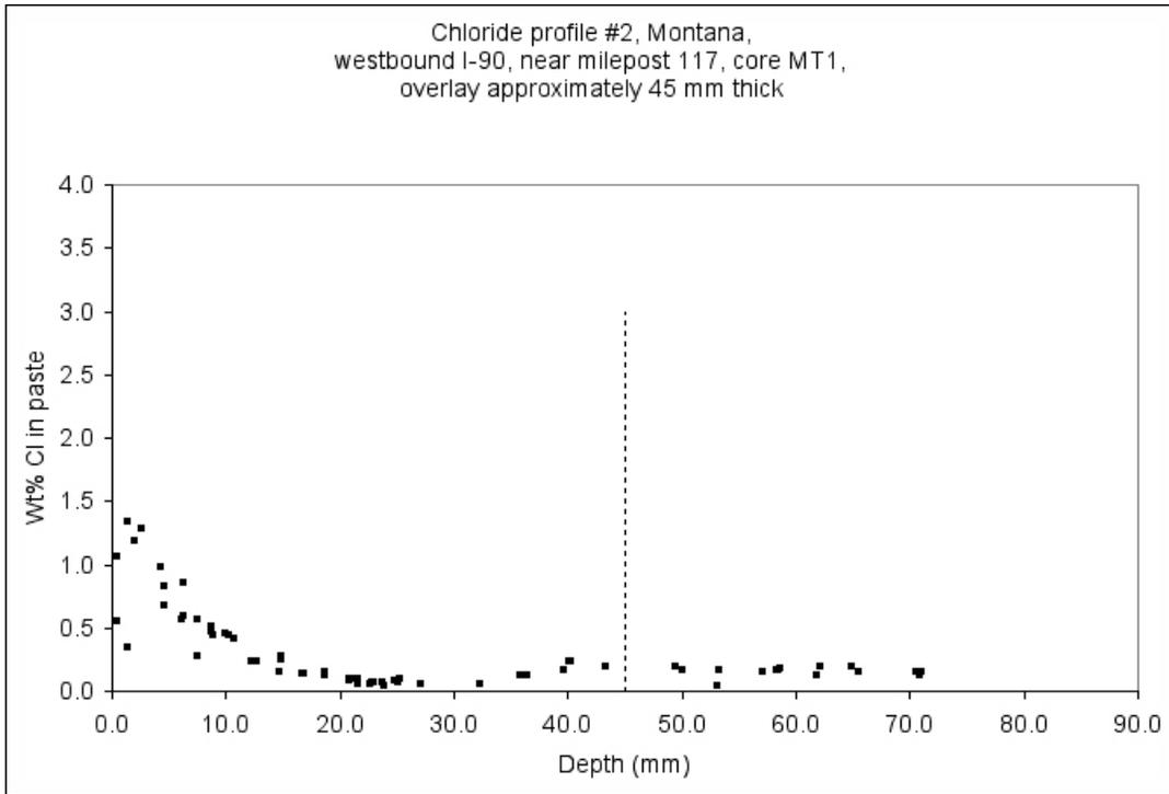
Figure MT-13: Chloride profile through cement paste from billet prepared from core MT-1, dashed line marks the transition between the overlay and the original concrete below.
