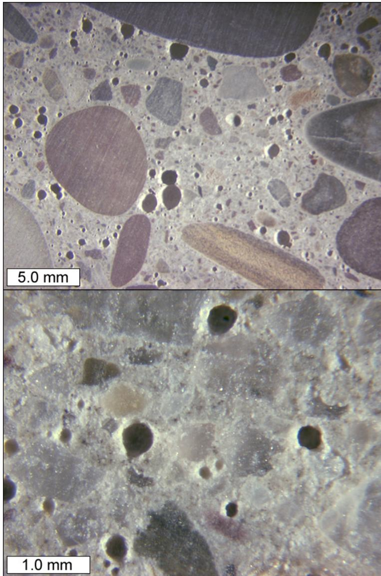
Figure S-7: Stereo microscope images to show air void structure on polished slab from core S-2.
