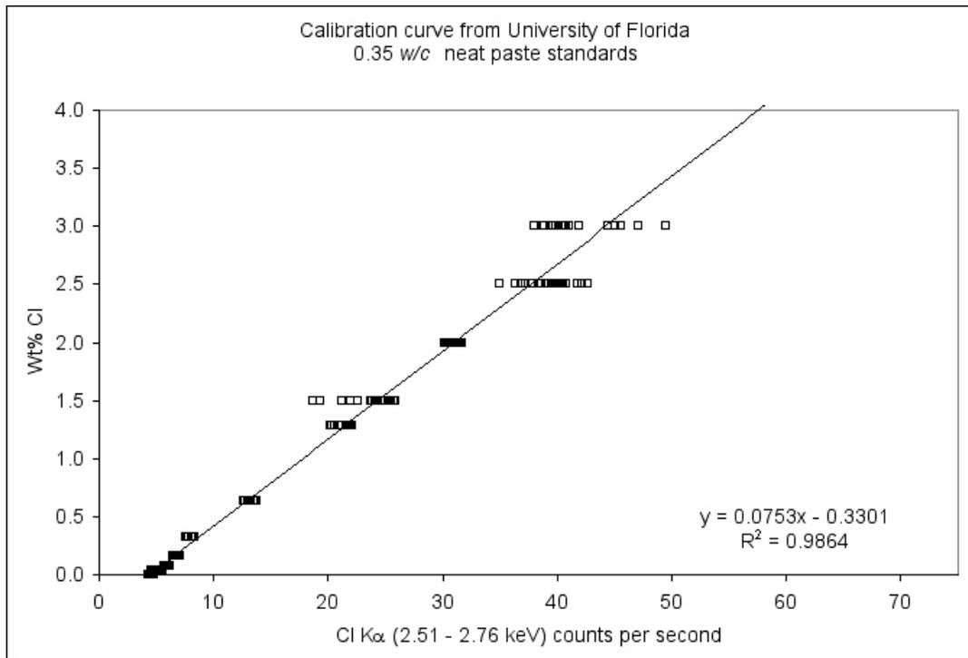
Figure B-3: Calibration curve plotting CI Ka counts per second versus wt% Cl from cement paste of 0.35 w/c neat cement standards.
