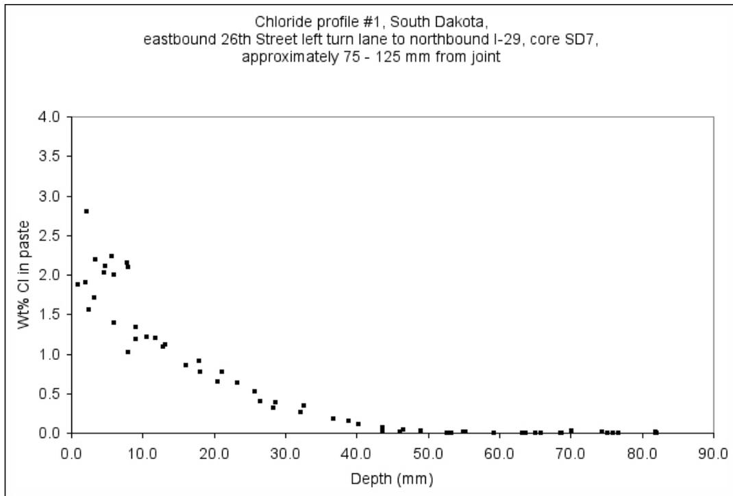
Figure SD-24: Chloride profile through cement paste, from billet prepared from core SD-7.
