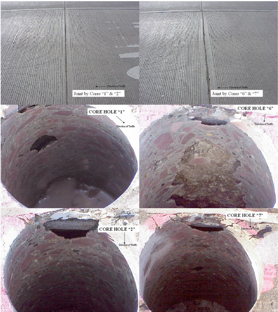
Figure SD-3: Photographs of the joints sampled, and of the holes after the coring operation.
