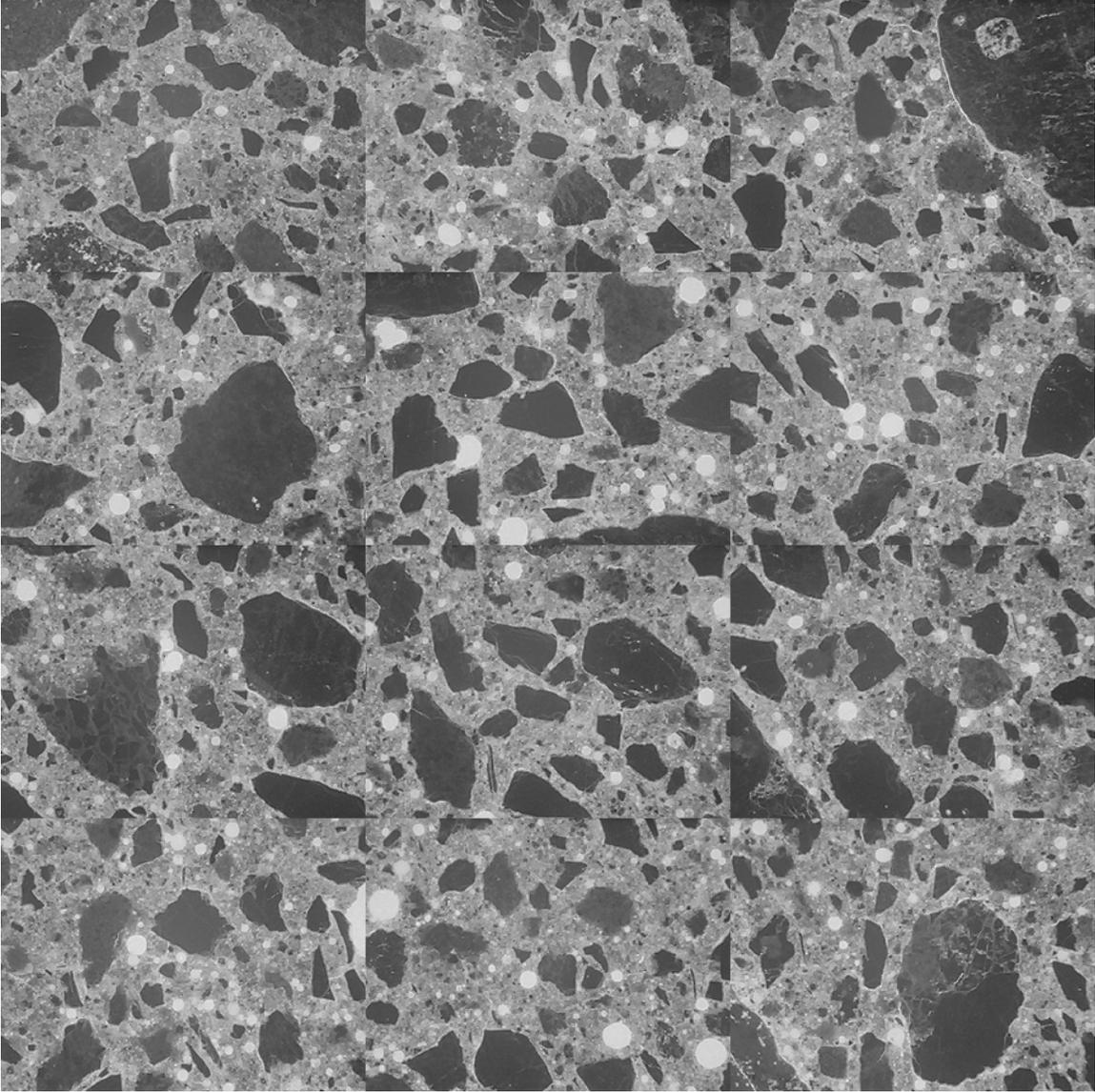
Figure MT-10: Mosaic of 12 frames collected from area of thin section representing the original concrete below the concrete overlay, core MT-3 (each individual frame measures 2.612 x 1.959 mm).
