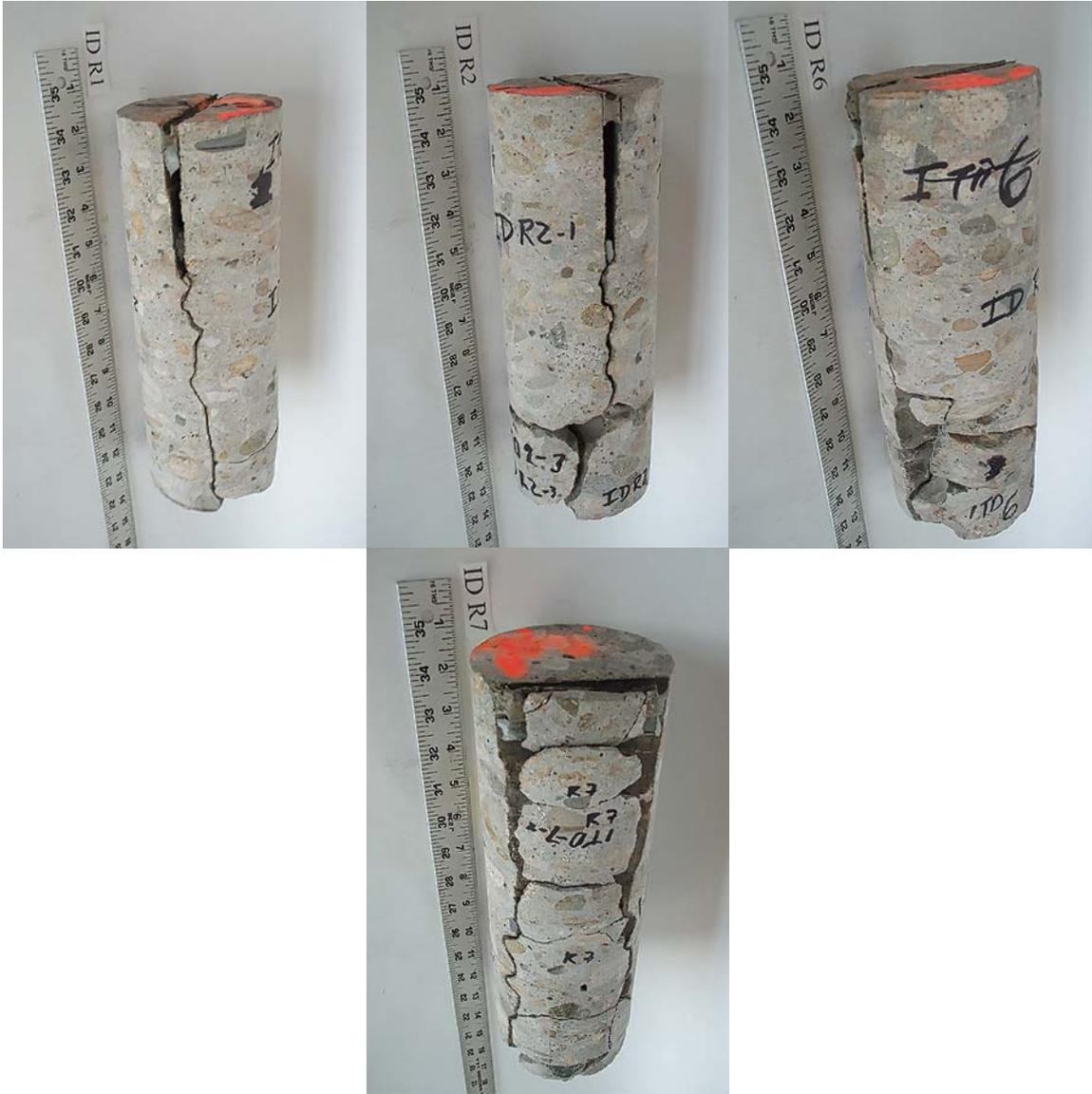
Figure ID-4: Cores from right lane taken near pavement joints.
