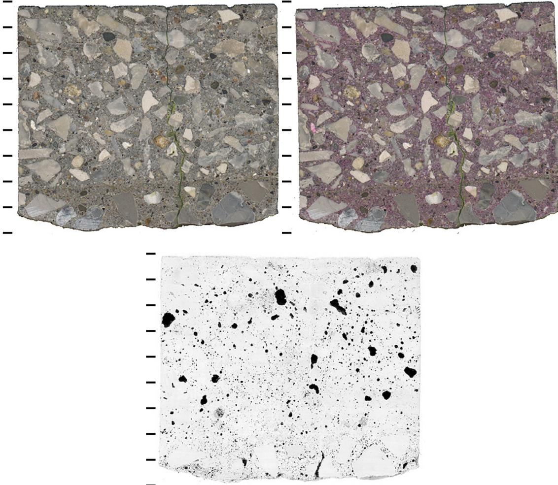
Figure IA-6: Polished slabs to show complete cross-section through core IA-7, before (upper left) and after application of phenolphthalein stain (upper right) and after treatment to enhance appearance of air voids and cracks (bottom) tic marks every cm. The slab was stabilized with epoxy prior to polishing due to the large crack running the down the middle of the core. Since the crack was filled with epoxy, it does not appear in the black and white enhanced image.
