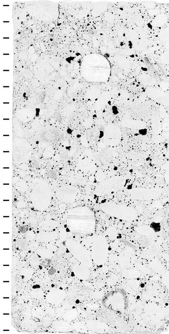
Figure S-6: Polished slabs to show complete cross-section through core S-2 after treatment to enhance appearance of air voids and cracks, tic marks every cm.
