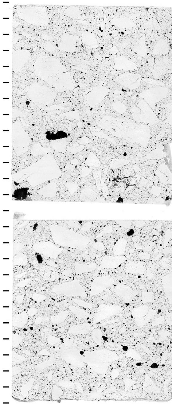
Figure CO-8: Polished slabs to show complete cross-section through core CO-5 after treatment to enhance appearance of air voids and cracks, tic marks every cm.
