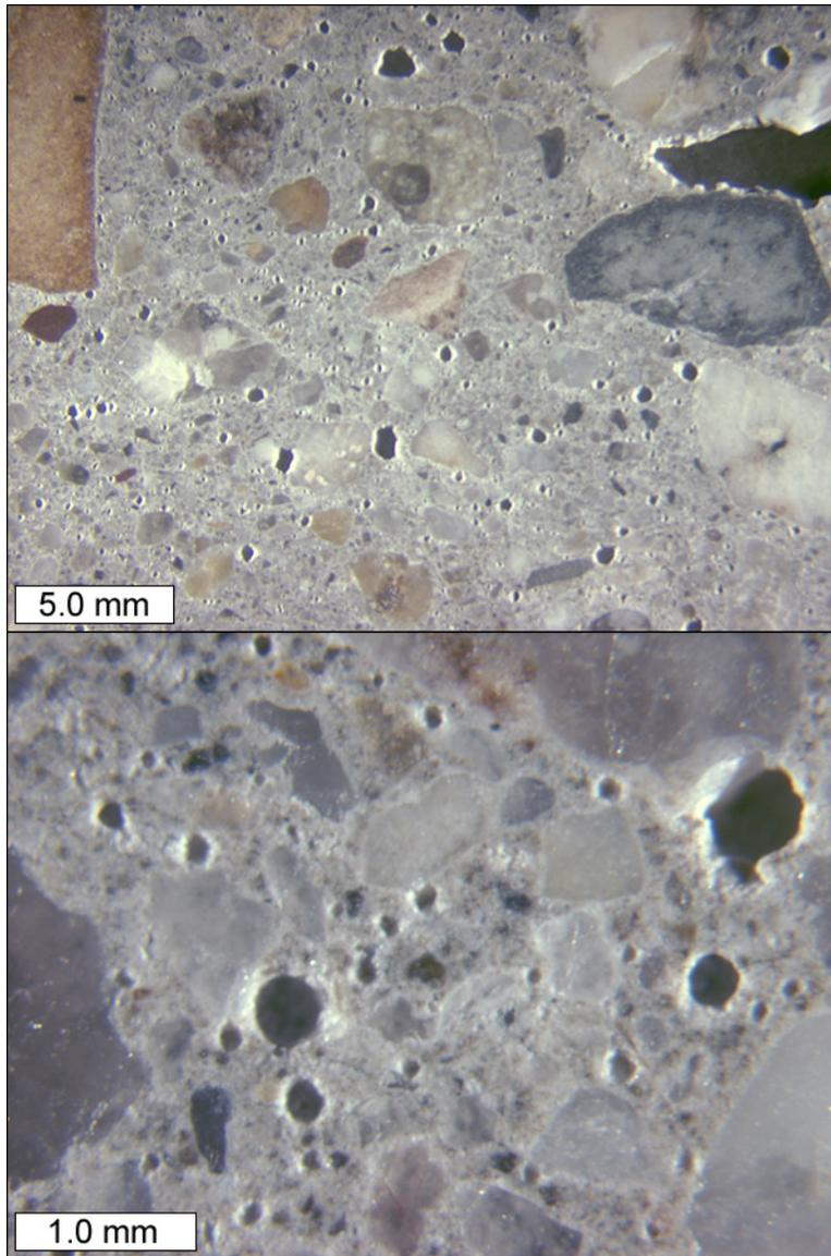
Figure T-7: Stereo microscope images to show air void structure on polished slab from core T-2.
