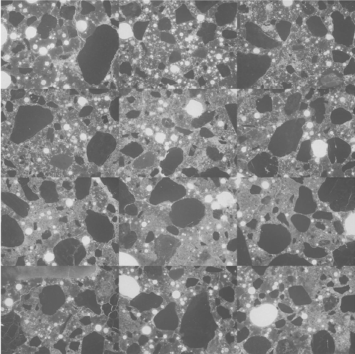
Figure SD-16: Mosaic of 12 frames collected from thin section prepared from billet cut from top portion of core SD-4 (each individual frame measures 2.612 x 1.959 mm).
