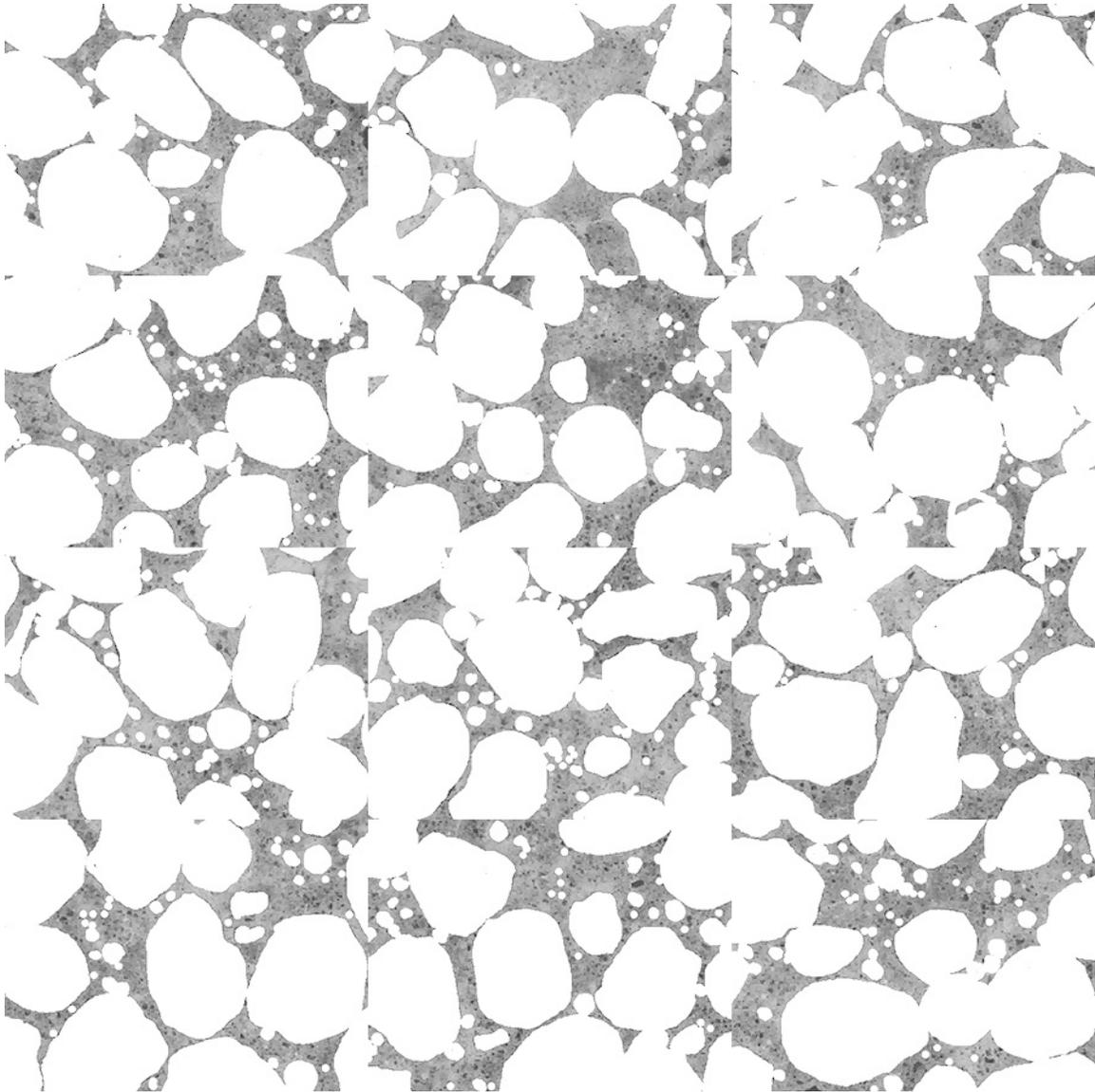
Figure A-4: Mosaic of 12 frames collected from 0.50 w/c 28 day moist cured mortar standards after masking out air voids and fine aggregate to isolate cement paste (each individual frame measures 2.612 x 1.959 mm).
