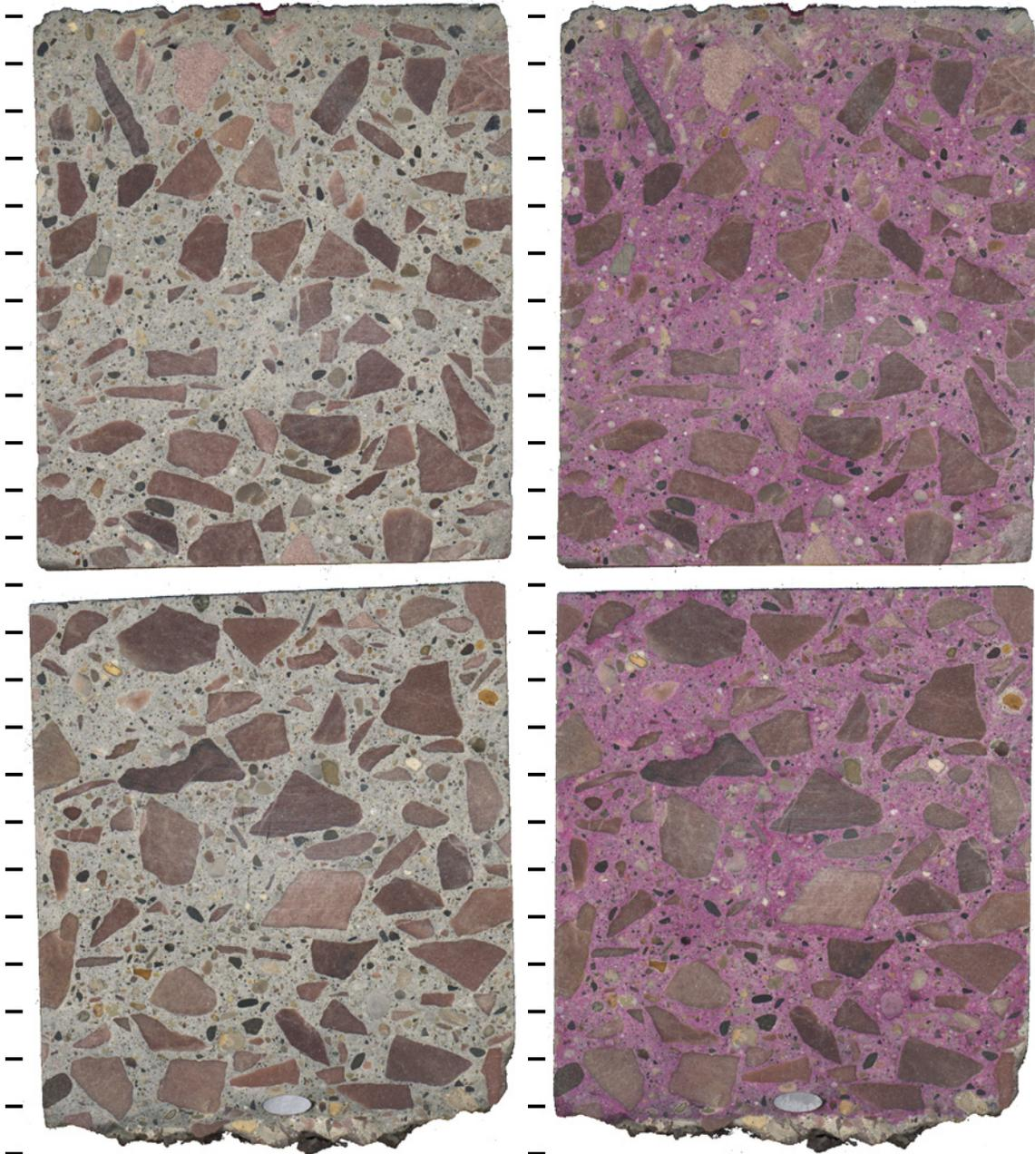
Figure SD-6: Polished slabs to show complete cross-section through core SD-1 both before (left) and after application of phenolphthalein stain (right) tic marks every cm.
