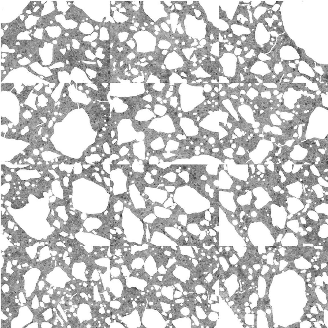
Figure MT-11: Mosaic of 12 frames collected area of thin section representing the original concrete below the concrete overlay, core MT-3, after masking out air voids, fine aggregate, and micro-cracks to isolate cement paste (each individual frame measures 2.612 x 1.959 mm).
