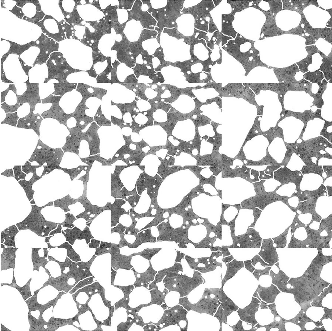
Figure IA-10: Mosaic of 12 frames collected from thin section prepared from billet cut from top portion of concrete overlay, core IA-3, after masking out air voids, fine aggregate, and micro-cracks to isolate cement paste (each individual frame measures 2.612 x 1.959 mm).
