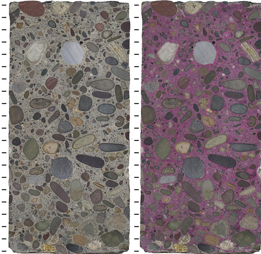
Figure S-5: Polished slabs to show complete cross-section through core S-2 both before (left) and after application of phenolphthalein stain (right) tic marks every cm.
