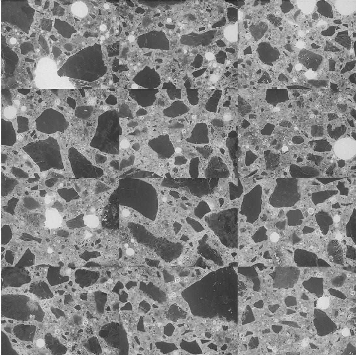
Figure ID-15: Mosaic of 12 frames collected from thin section prepared from billet cut from top portion of core IDL-1 (each individual frame measures 2.612 x 1.959 mm).
