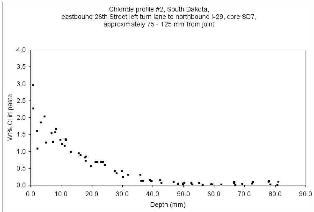
Figure SD-16: Chloride profile through cement paste, from billet prepared from core SD-7.
