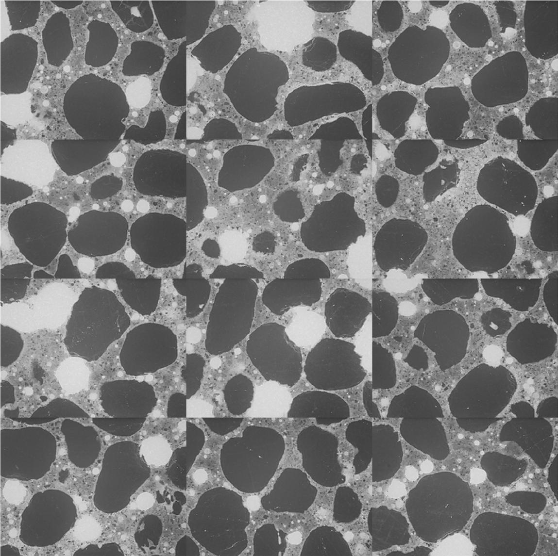
Figure A-1: Mosaic of 12 frames collected from 0.40 w/c 28 day moist cured mortar standards (each individual frame measures 2.612 x 1.959 mm).
