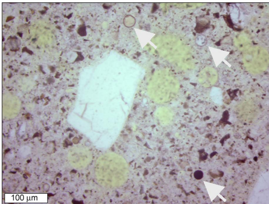
Figure CO-17: Transmitted light image, with arrows indicating some of the fly ash particles.
