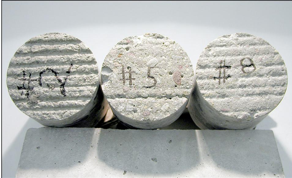
Figure MT-3: Photograph to show variation in surface wear from core to core.
