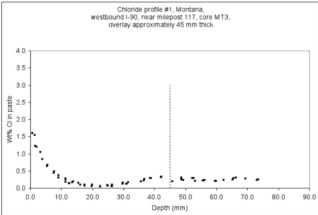
Figure MT-14: Chloride profile through cement paste from billet prepared from core MT-3, dashed line marks the transition between the overlay and the original concrete below.
