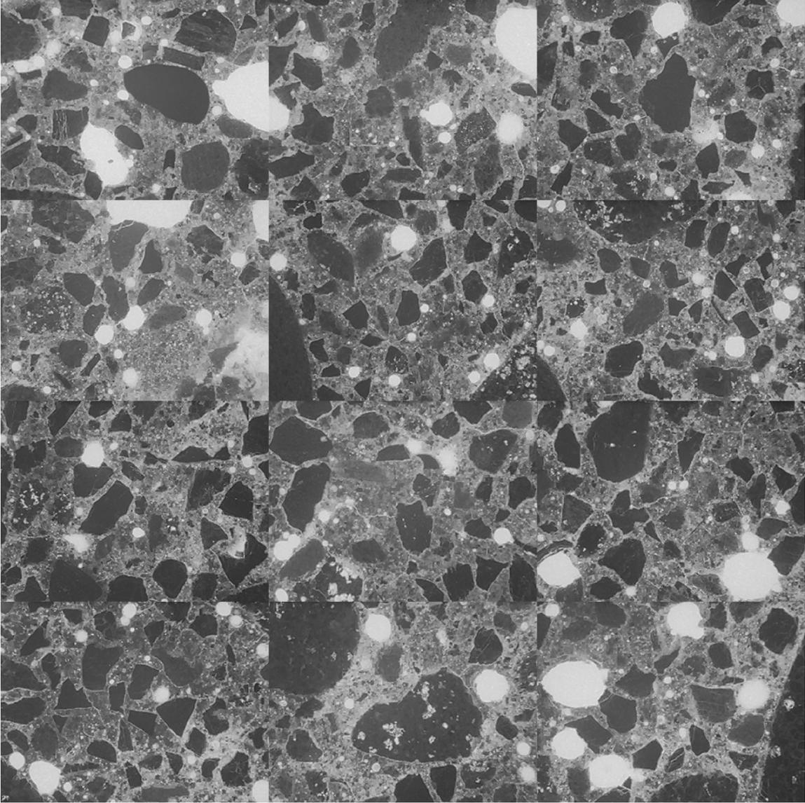
Figure S-8: Mosaic of 12 frames collected from thin section prepared from billet cut from top portion of core S-2 (each individual frame measures 2.612 x 1.959 mm).
