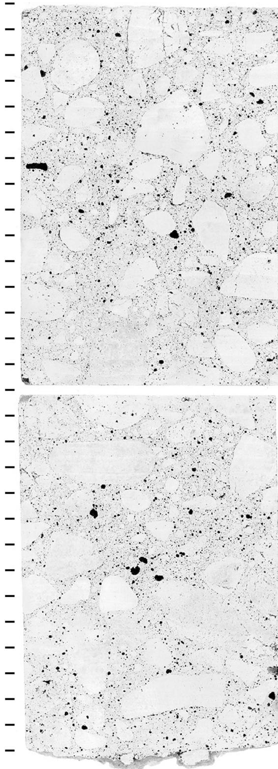
Figure ID-13: Polished slabs to show complete cross-section through core IDR-3 after treatment to enhance appearance of air voids and cracks, tic marks every cm.
