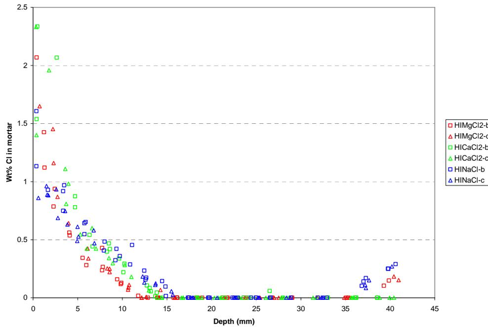
Figure 5. Chloride profiles of 0.45w/c PC mortar billets in three high concentration deicer solutions.
