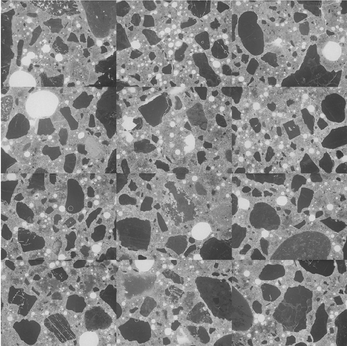
Figure SD-14: Mosaic of 12 frames collected from thin section prepared from billet cut from top portion of core SD-7 (each individual frame measures 2.612 x 1.959 mm).
