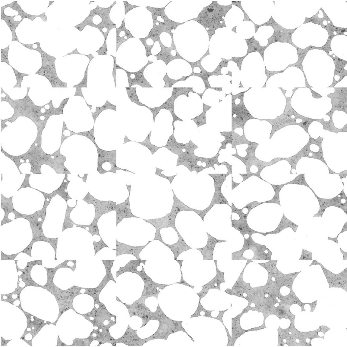
Figure A-6: Mosaic of 12 frames collected from 0.60 w/c 28 day moist cured mortar standards after masking out air voids and fine aggregate to isolate cement paste (each individual frame measures 2.612 x 1.959 mm).
