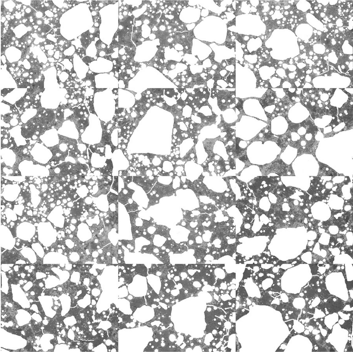
Figure SD-20: Mosaic of 12 frames collected from thin section prepared from billet cut from top portion of core SD-5 after masking out air voids, fine aggregate, and micro-cracks to isolate cement paste (each individual frame measures 2.612 x 1.959 mm).
