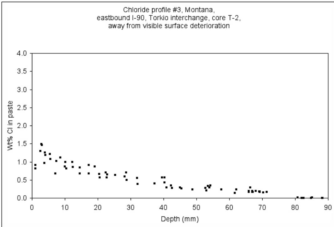
Figure T-12: Chloride profile through cement paste, from billet prepared from core T-2.
