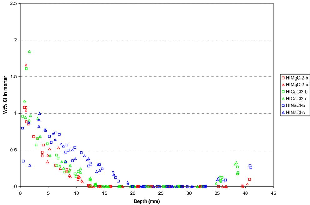
Figure 6. Chloride profiles of 0.55w/c PC mortar billets in three high concentration deicer solutions.
