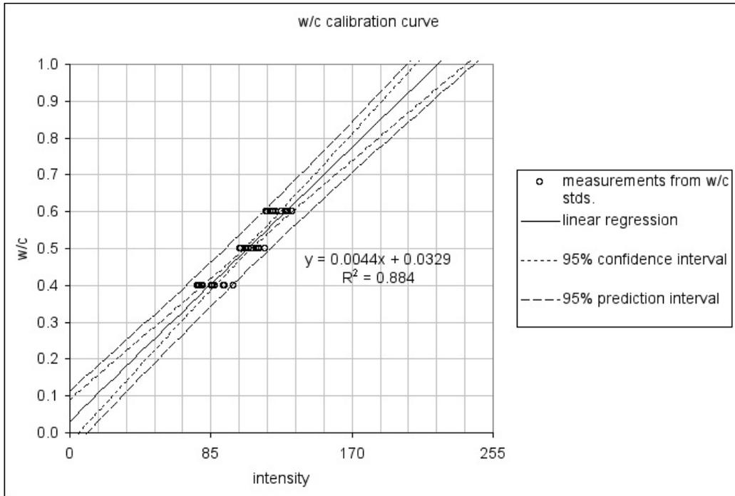
Figure A-8: Calibration curve plotting average cement paste pixel fluorescence intensity per frame versus w/c.
