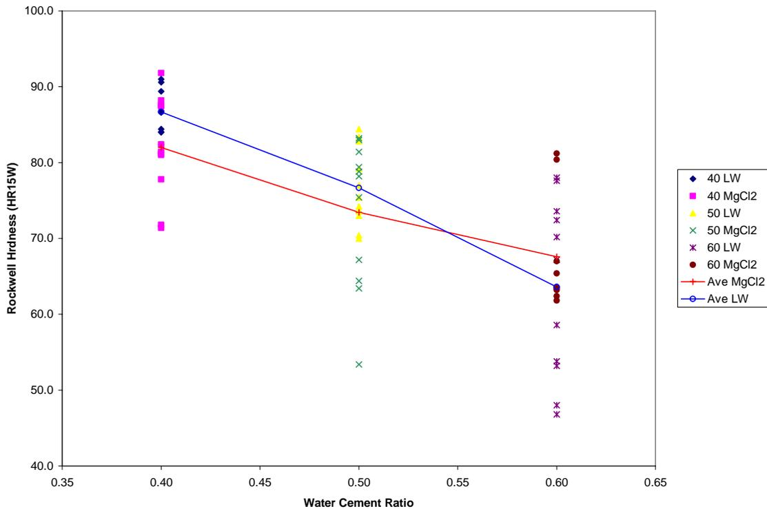
Figure 1. Rockwell Hardness of various Portland cement mortar samples.
