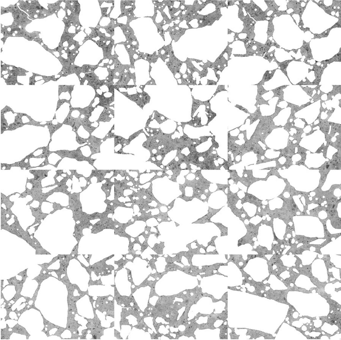
Figure CO-12: Mosaic of 12 frames collected from thin section prepared from billet cut from top portion of core CO-6 after masking out air voids and fine aggregate to isolate cement paste (each individual frame measures 2.612 x 1.959 mm).
