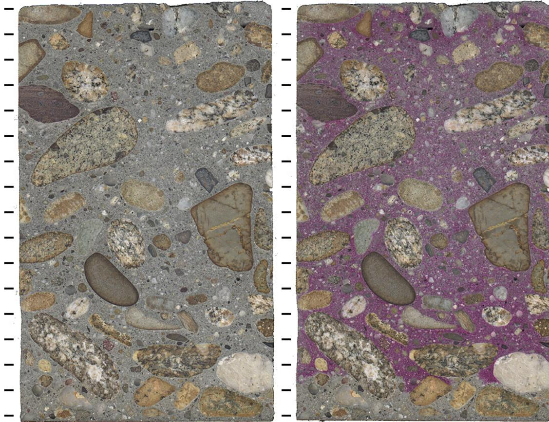
Figure T-5: Polished slabs to show complete cross-section through core T-2 both before (left) and after application of phenolphthalein stain (right) tic marks every cm.
