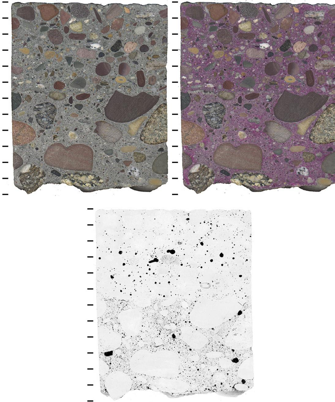
Figure MT-6: Polished slabs to show complete cross-section through core MT-8, before (upper left) and after application of phenolphthalein stain (upper right) and after treatment to enhance appearance of air voids and cracks (bottom) tic marks every cm.
