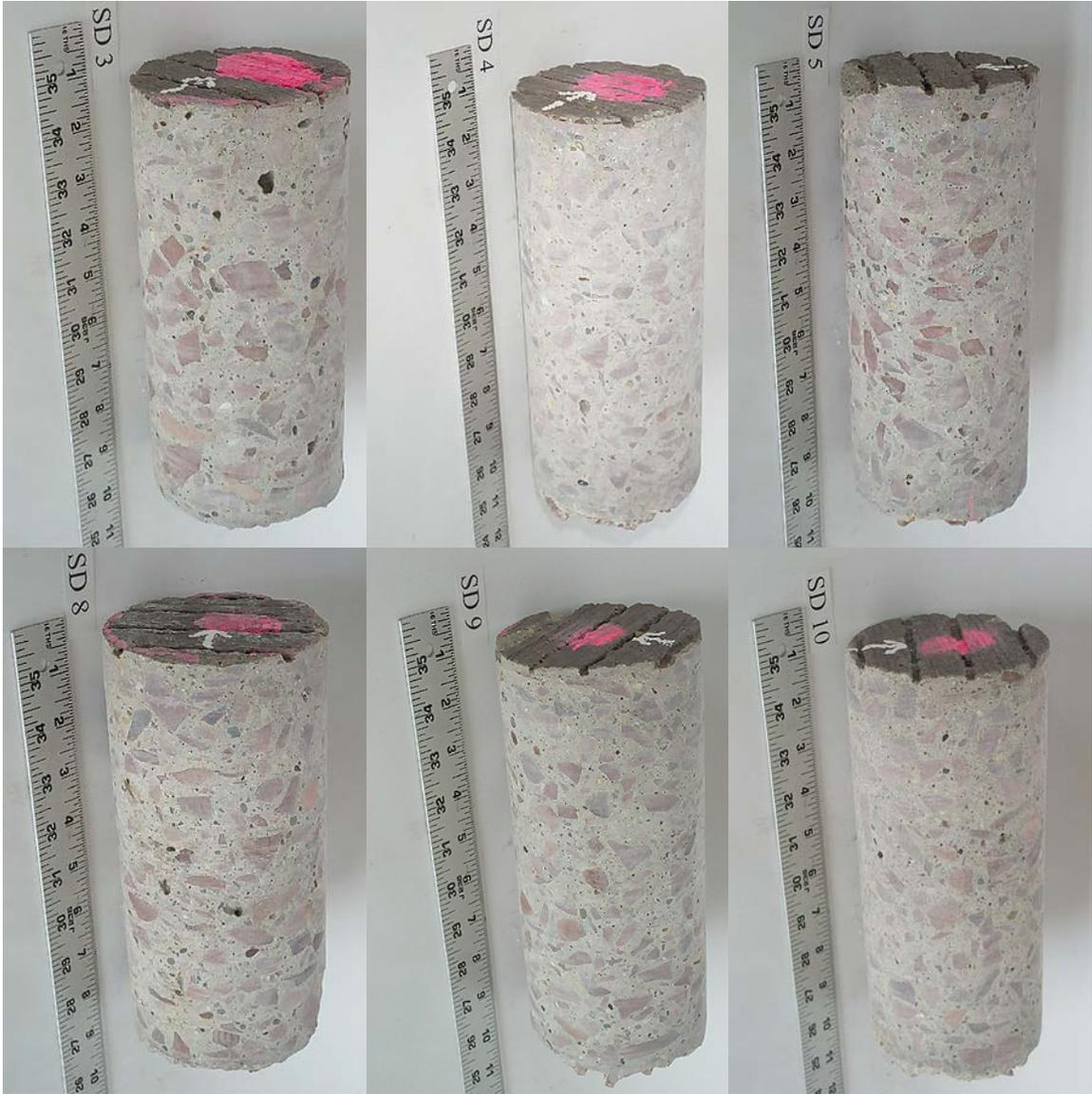
Figure SD-5: Cores taken away from joint.
