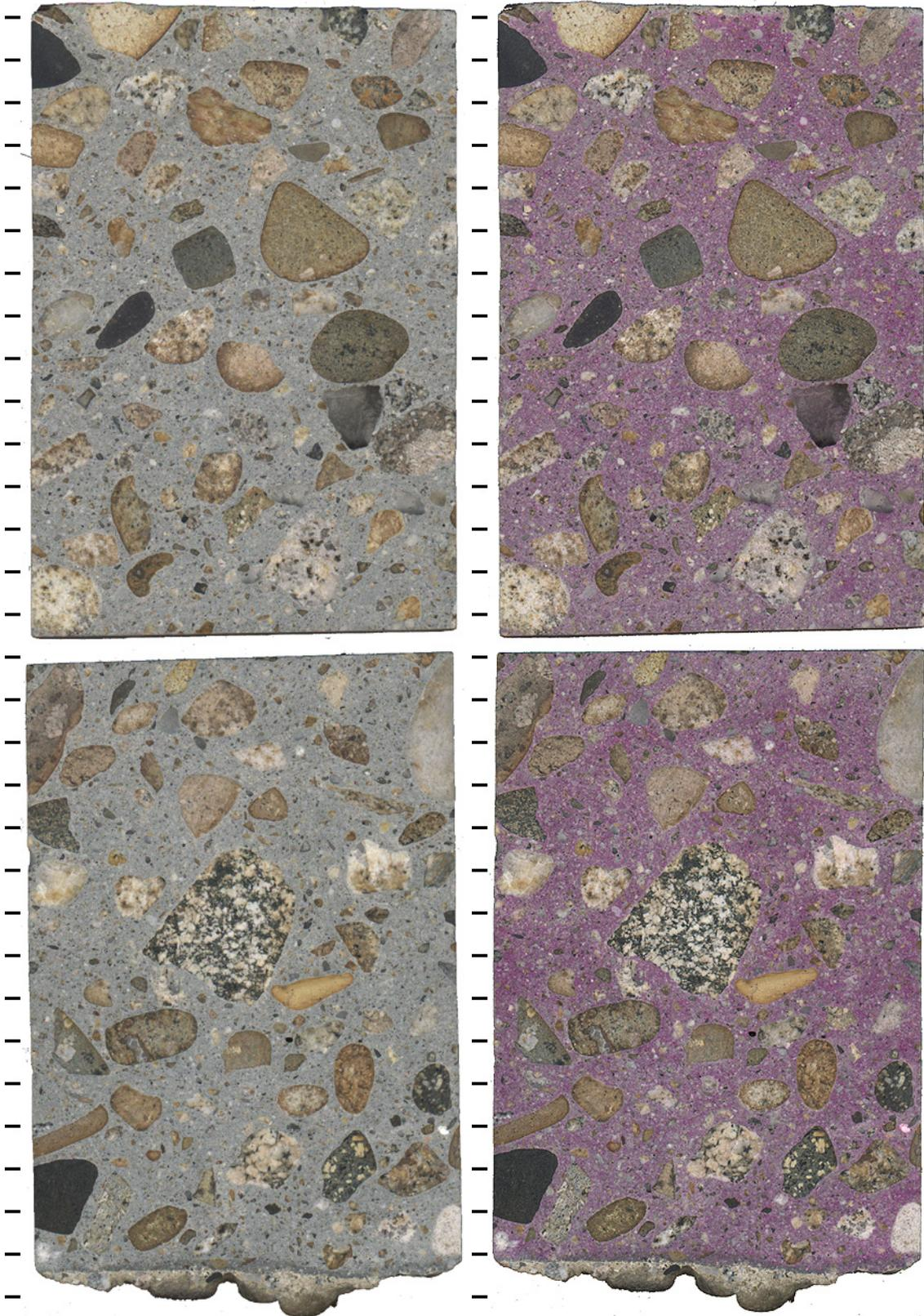
Figure ID-8: Polished slabs to show complete cross-section through core IDL-4 both before (left) and after application of phenolphthalein stain (right) tic marks every cm.
