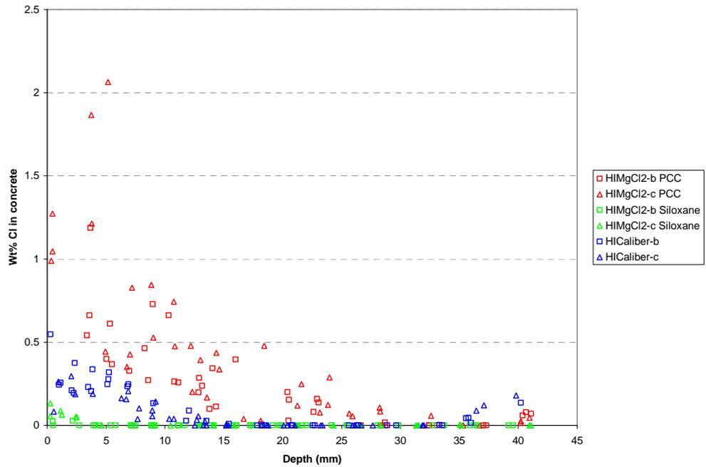
Figure 9. Chloride profiles of 0.55w/c PCC and PCC-siloxane sealed in high concentration  $MgCl_2$  solution with PCC in high concentration Caliber solution.
