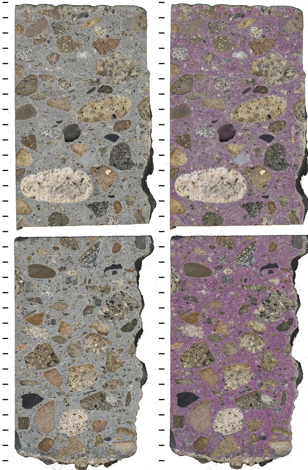
Figure ID-6: Polished slabs to show complete cross-section through core IDL-6 both before (left) and after application of phenolphthalein stain (right) tic marks every cm.
