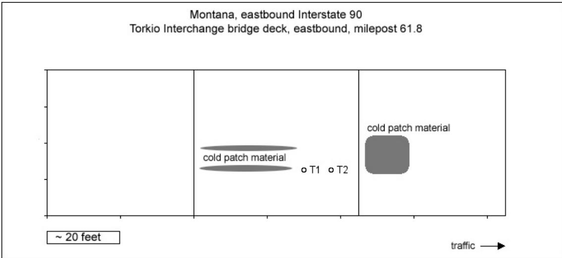
Figure T-1: Diagram to show location of cores according to field notes.
