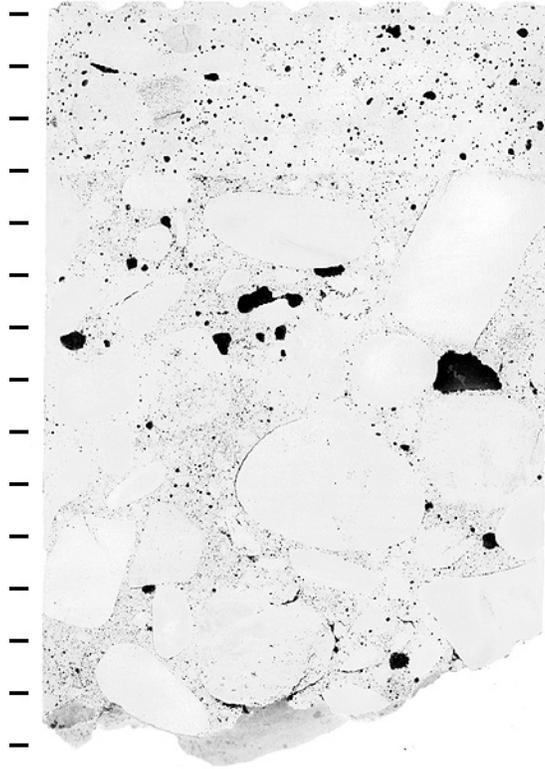
Figure MT-5: Polished slabs to show complete cross-section through core MT-2 after treatment to enhance appearance of air voids and cracks, tic marks every cm.
