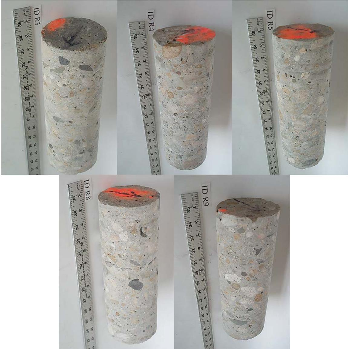
Figure ID-5: Cores from right lane taken away from pavement joints.
