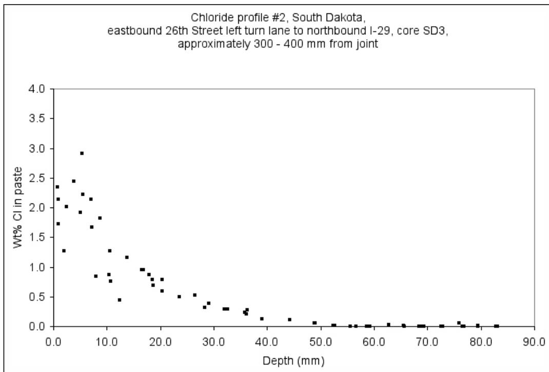
Figure SD-23: Chloride profile through cement paste, from billet prepared from core SD-3.
