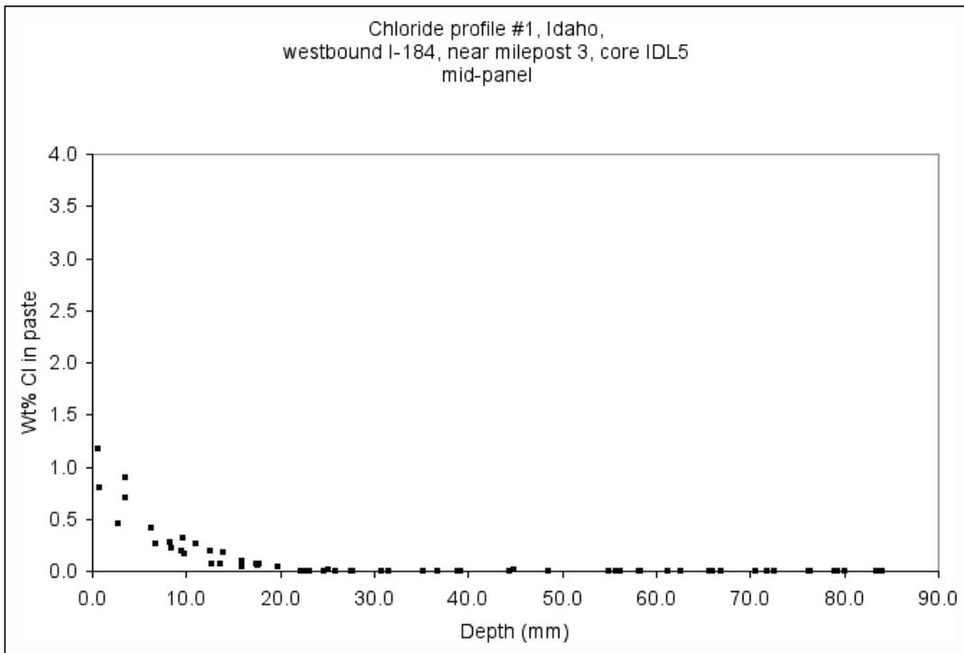
Figure ID-19: Chloride profile through cement paste at mid-panel, from billet prepared from core IDL-5.
