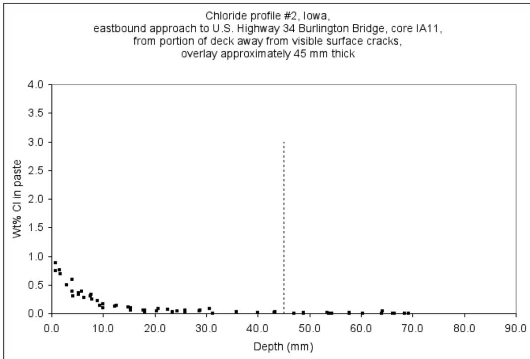
Figure IA-16: Chloride profile through cement paste, from billet prepared from core IA-11, dashed line marks the transition point between concrete overlay and the original concrete below the overlay.
