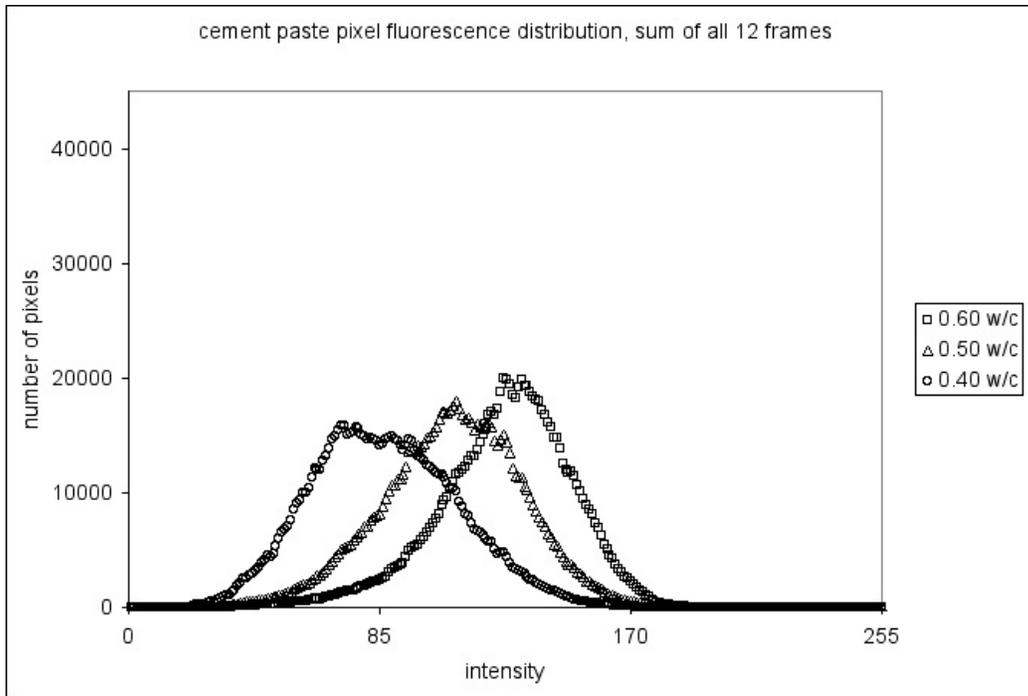
Figure A-7: Histogram plotting cement paste pixel intensities using all 12 frames collected from each of the 28 day moist cured mortar standards.
