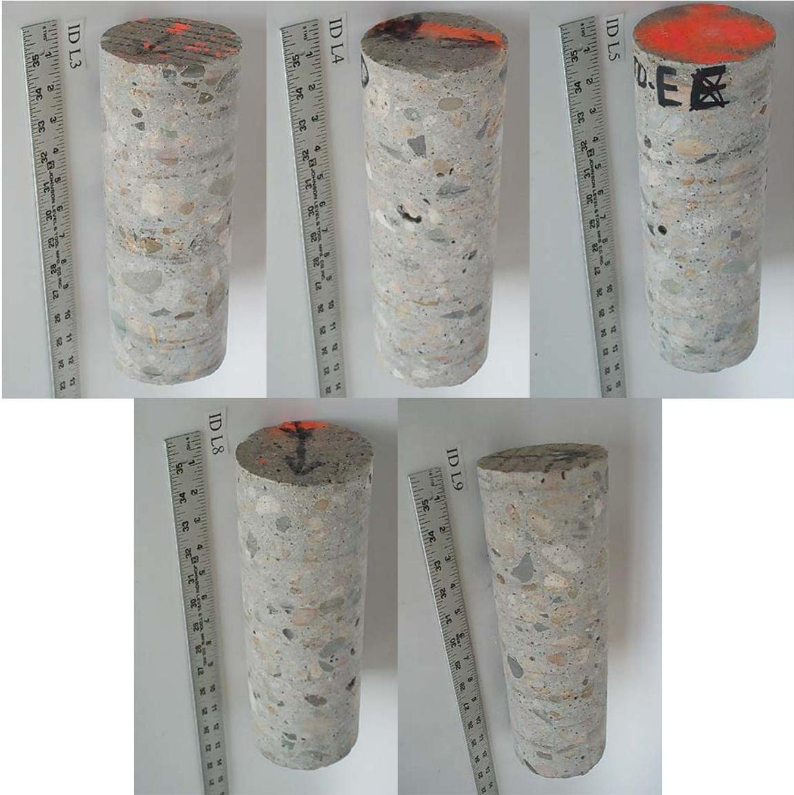
Figure ID-3: Cores from left lane taken away from pavement joints.
