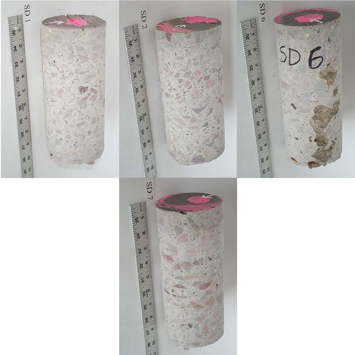
Figure SD-4: Cores taken at joint.
