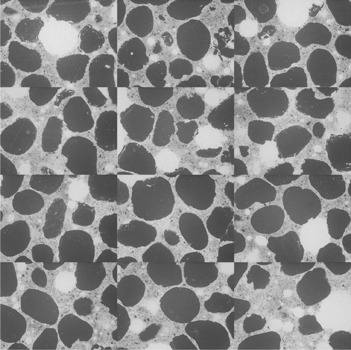
Figure A-5: Mosaic of 12 frames collected from 0.60 w/c 28 day moist cured mortar standards (each individual frame measures 2.612 x 1.959 mm).
