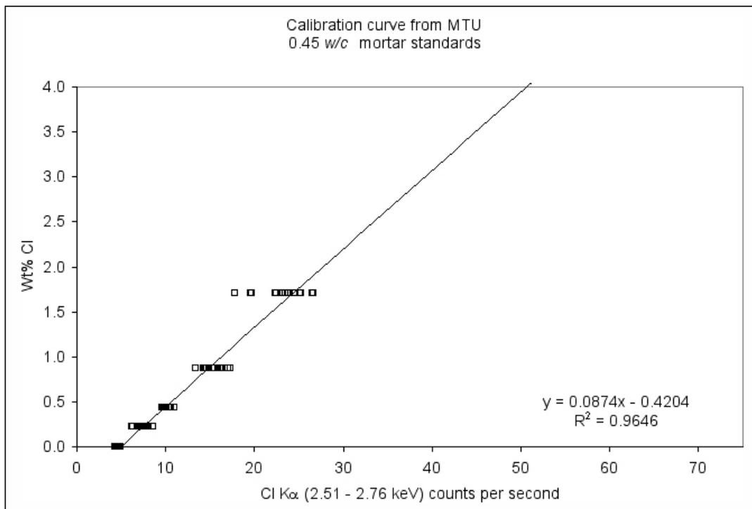
Figure B-2: Calibration curve plotting CI Ka counts per second versus wt% Cl from cement paste of 0.45 w/c mortar standards.
