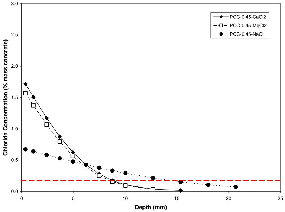
Figure 1. Portland cement concrete samples (w/c=0.45) - chloride profiles for different salts
