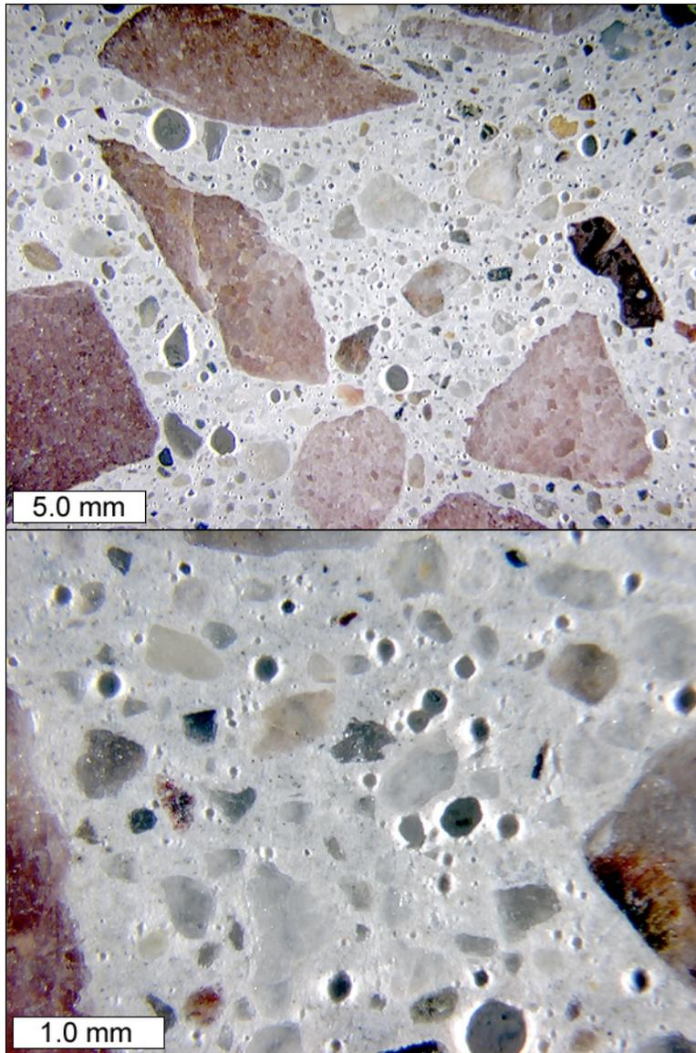
Figure SD-10: Stereo microscope images to show air void structure on polished slab from core SD-4.
