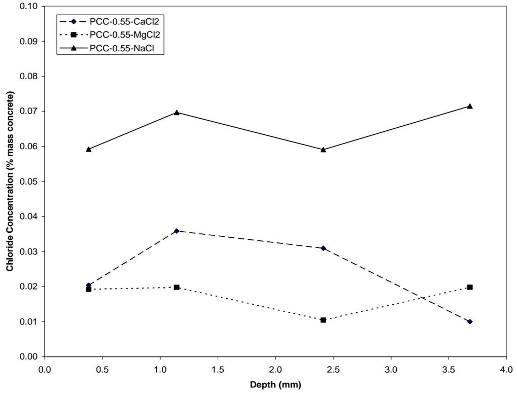
Figure 7. Portland cement concrete samples (sealer 1) - chloride profiles
