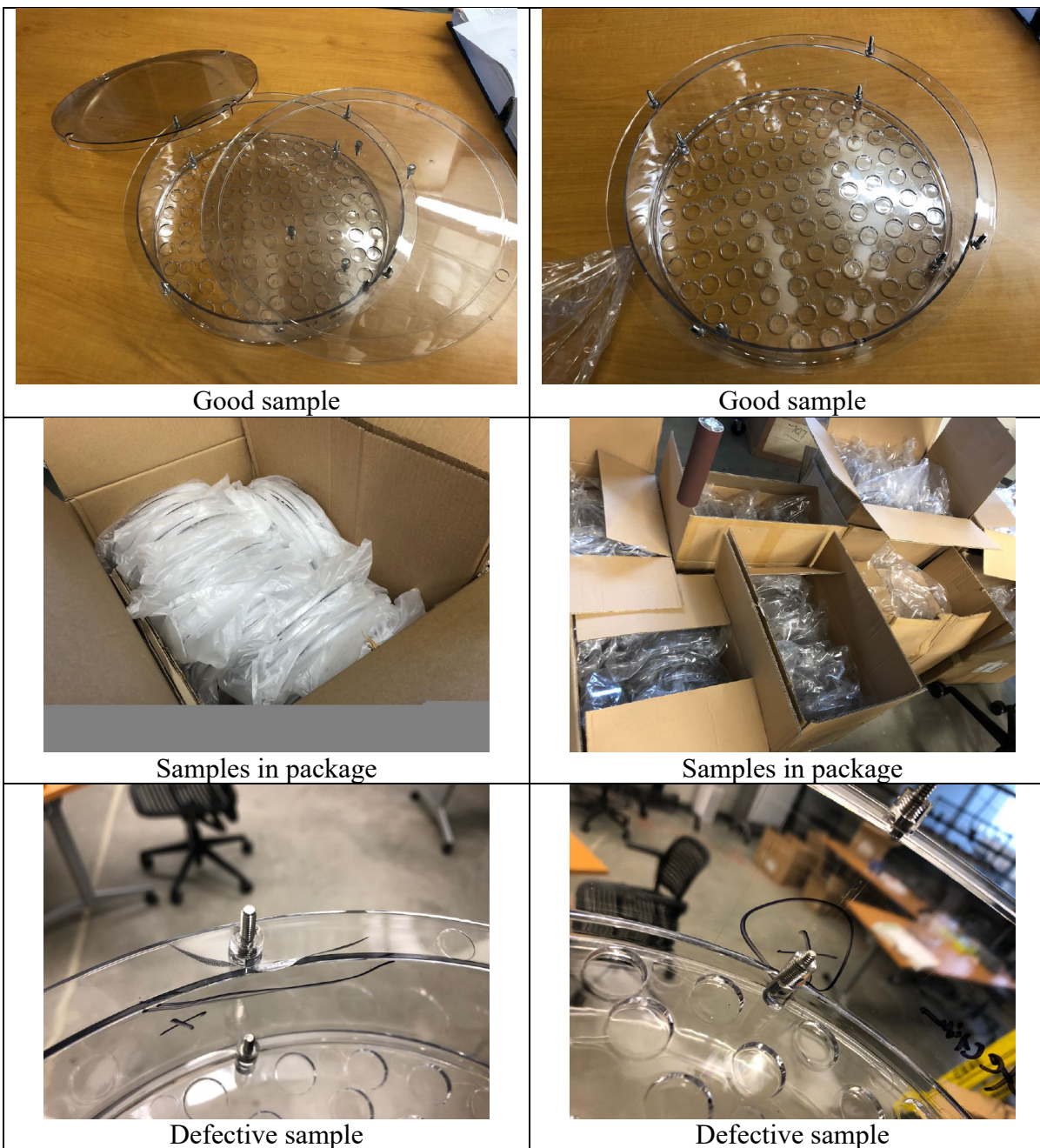
Figure 1 New samples of the finalized new self-de-icing signal housing, made of PC material Markrolon 2807 for UL certificate using revised mass production technology to correct the defective concaved lens surface of the plastic housing in mass production, with a maximum tolerance of 1.5 mm.
