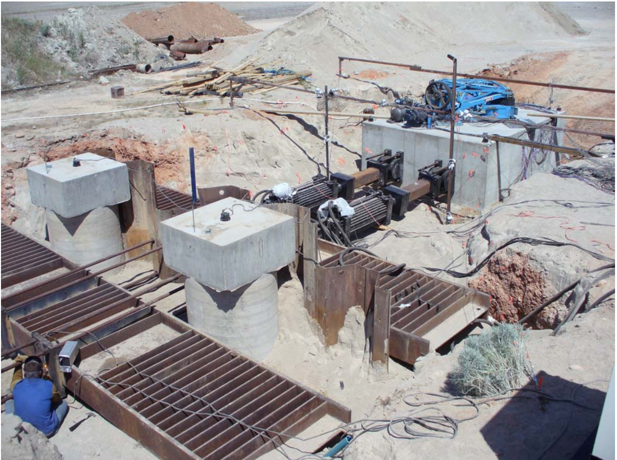
Fig. 1. Looking northwest at test site with reaction foundation (foreground), two 600 kip hydraulic actuators, and eccentric-mass shaker (blue device in background) mounted to test pile cap
