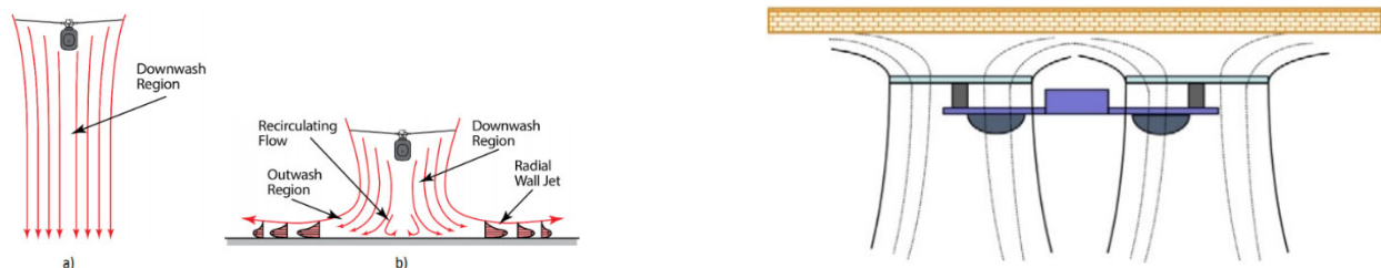
Figure 2 Ground effects (left) and Ceiling effects (right) in UAVs
