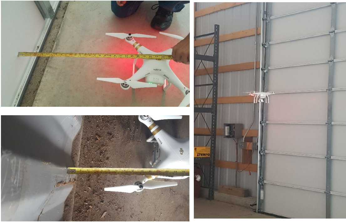
Figure 4 Trials to determine a safe clearance distance
