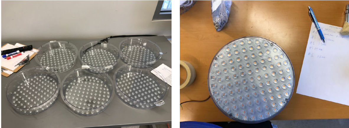
Figure 1 New trial samples of the improved technology for our new housing by increasing the runner size from 4 mm to 6 mm in the injection molding using a bigger machine for trial. We have received and tested 6 samples of the new housing made with the improved technology in two options.
