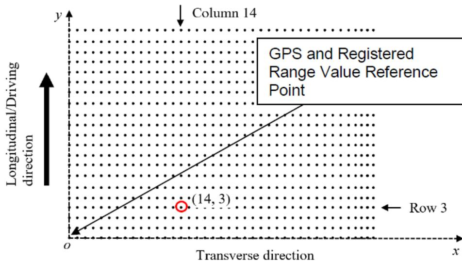
**Figure 4. Graph. Recommended coordinate system for a 2D/3D image.**
