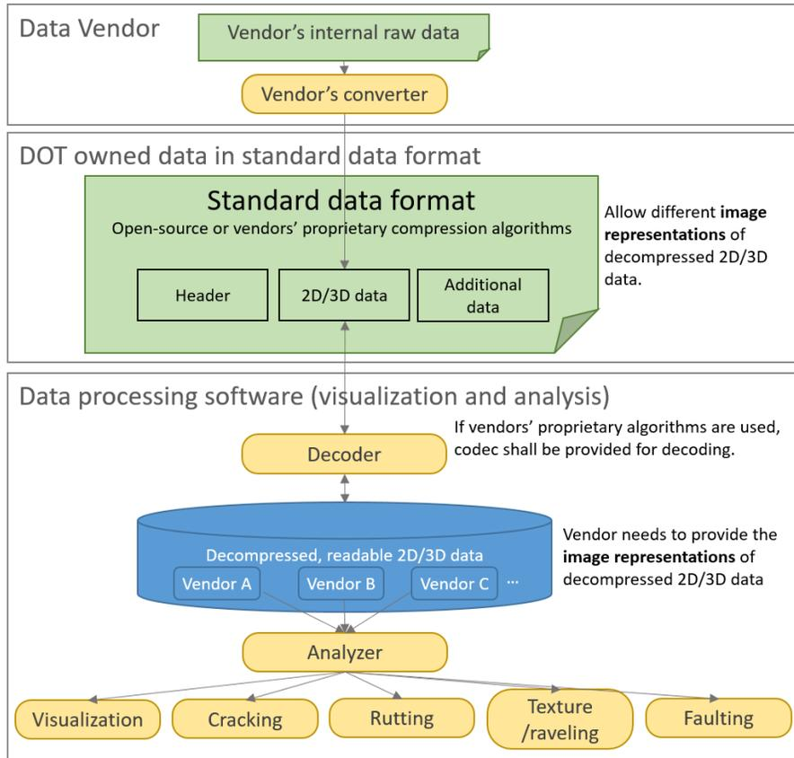
**Figure 1. Chart. Original standard 2D/3D data format and possible usage.**
