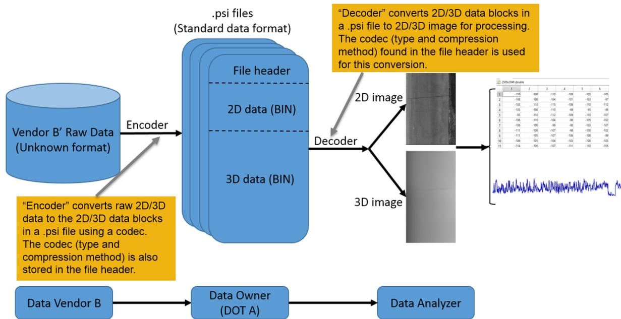
**Figure 7. Chart. Preliminary testing of using standard data format.**
