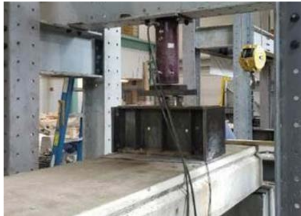
Figure 1: full-scale arch beam test setup
