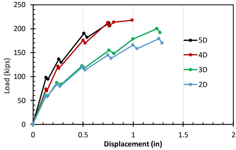
Fig. 2 Measured lateral pile head load versus deflection curves for 24-inch diameter free-head test piles located at 2, 3, 4, and 5 pile diameters (D) behind the wall. (Results are preliminary based on measurements during field testing.)
