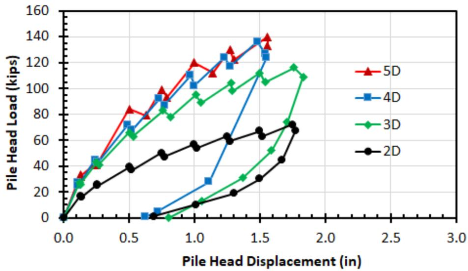
Fig. 1 Measured lateral pile head load versus deflection curves for fixed head test piles located at 2, 3, 4, and 5 pile widths (D) behind the wall. (Preliminary results based on measurements during field testing.)
