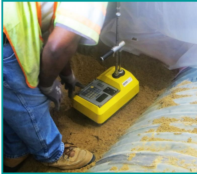
Figure A3: Nuclear Density Measurement to Check the Compaction Rate.
