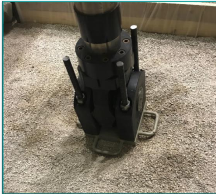
Figure A15: Load Pad Penetration into the Soil due to the Soil Failure at the Ultimate Load.
