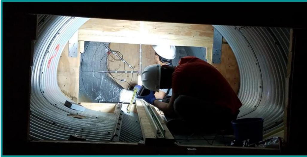
Figure A33: Initial Measurement and Instrumentation Installation for the invert-cut 47 in. × 71 in. Arch CMP.
