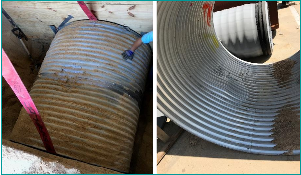
Figure A32: Pipe Exhumation and Storage – Intact 60 in. Circular CMP.
