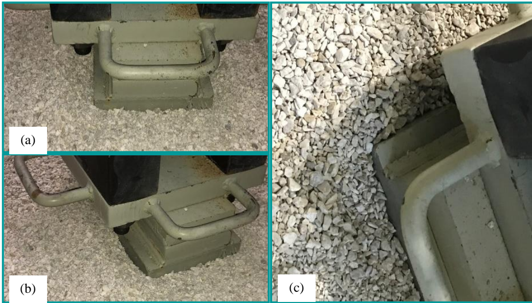
Figure A14: Load Pad (10 in. \times 20 in.) Configuration on the soil at: (a) 16,650 lb. Service Load, (b) and (c) both at the Soil Failure Initiation.
