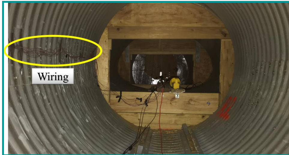
Figure A9: Partition Walls Opening and Wiring inside the CMPs.
