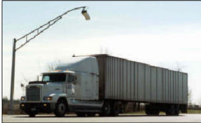
Figure 1: Electronic Screening of a Commercial Vehicle (6)
