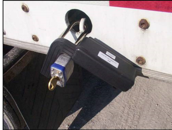
Figure 5: E-Seal Attached to Freight Trailer (5)
