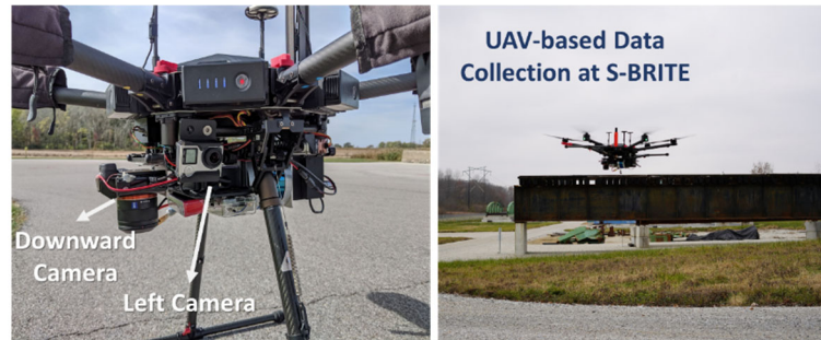
Figure 3: Illustration of the UAV system flown over S-BRITE for Geometric Resolution investigation
