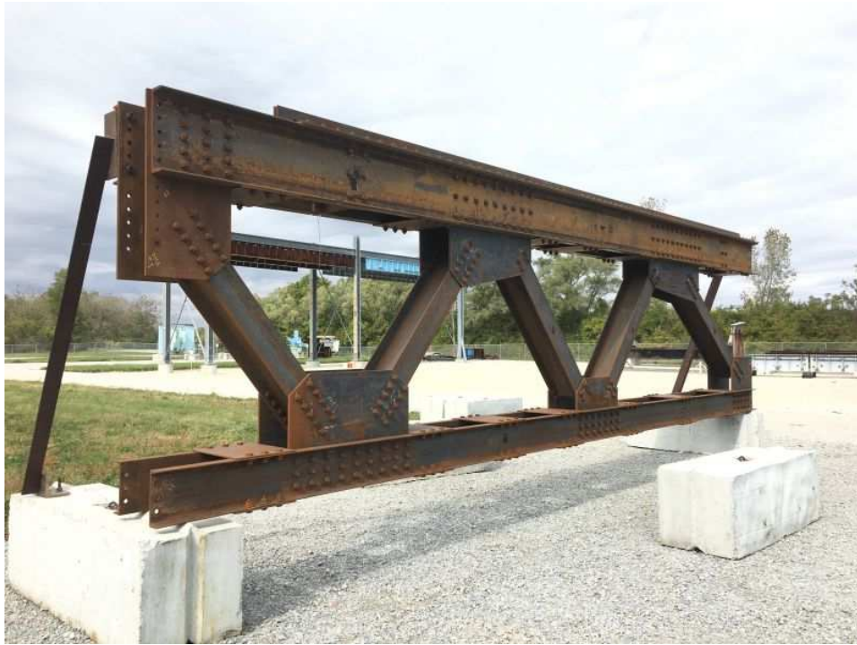
Photograph 3 – Bolted Steel Truss Specimen
