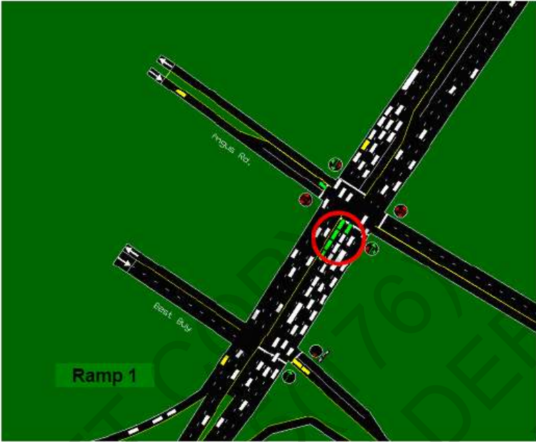
B. Subfigure of lane change difficulty at an intersection downstream from ramp 1.
