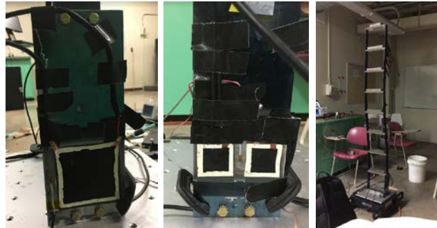
Figure 5.7: Test Specimens, Shear Building on a Shake Table
