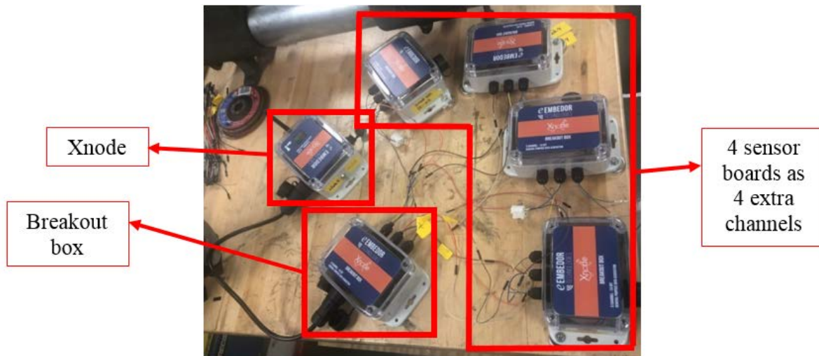
Figure 6.23: Connection of Sensor Boards to Xnode Through the Breakout Box
