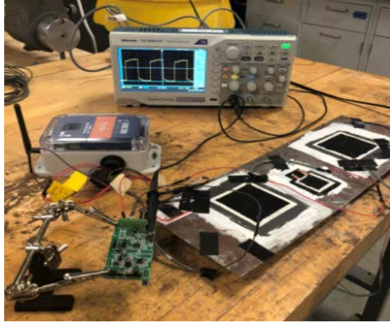
Figure 6.7: Capacitance Sensor Board Setup for Balancing and Shunt Calibration
