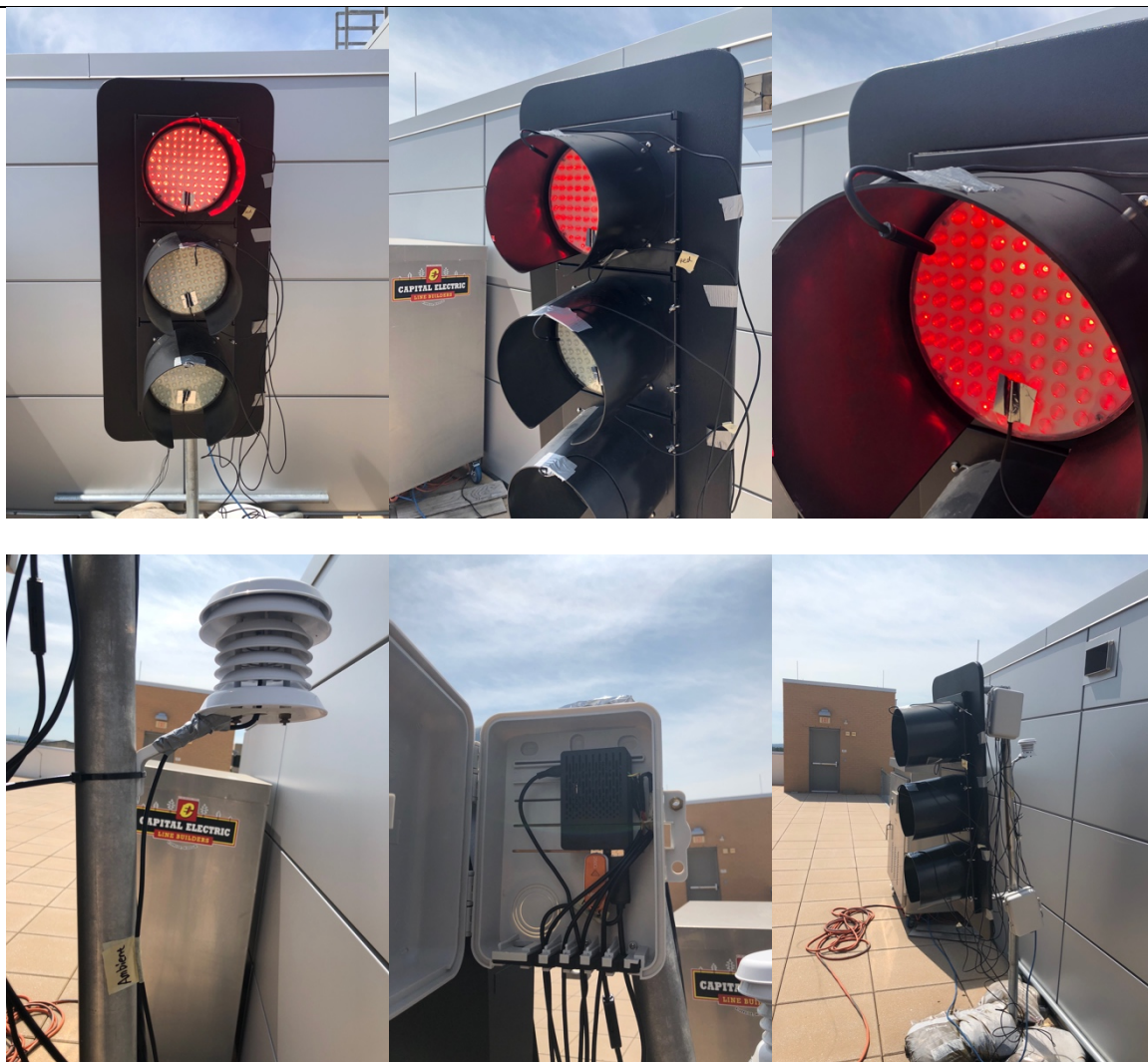
Figure 4 roof tests of the latest prototypes with a self-designed and custom built in-house field monitoring system. This is the whole system to be mounted at every field test site for year-around real-time monitoring and data recording of the new signals in the field.
