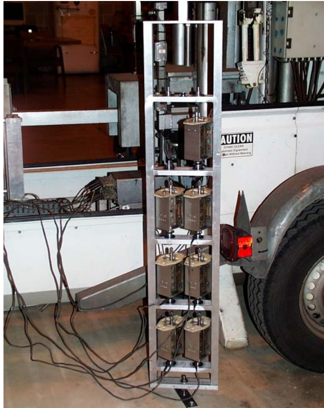
Figure 83. Photo. Seismometer stand with sensors attached.
