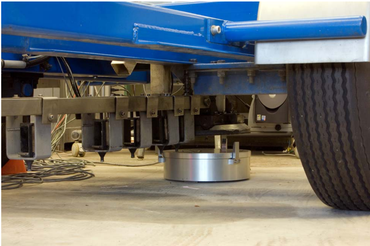
Figure 69. Photo. Reference load cell positioned under the FWD load plate.
