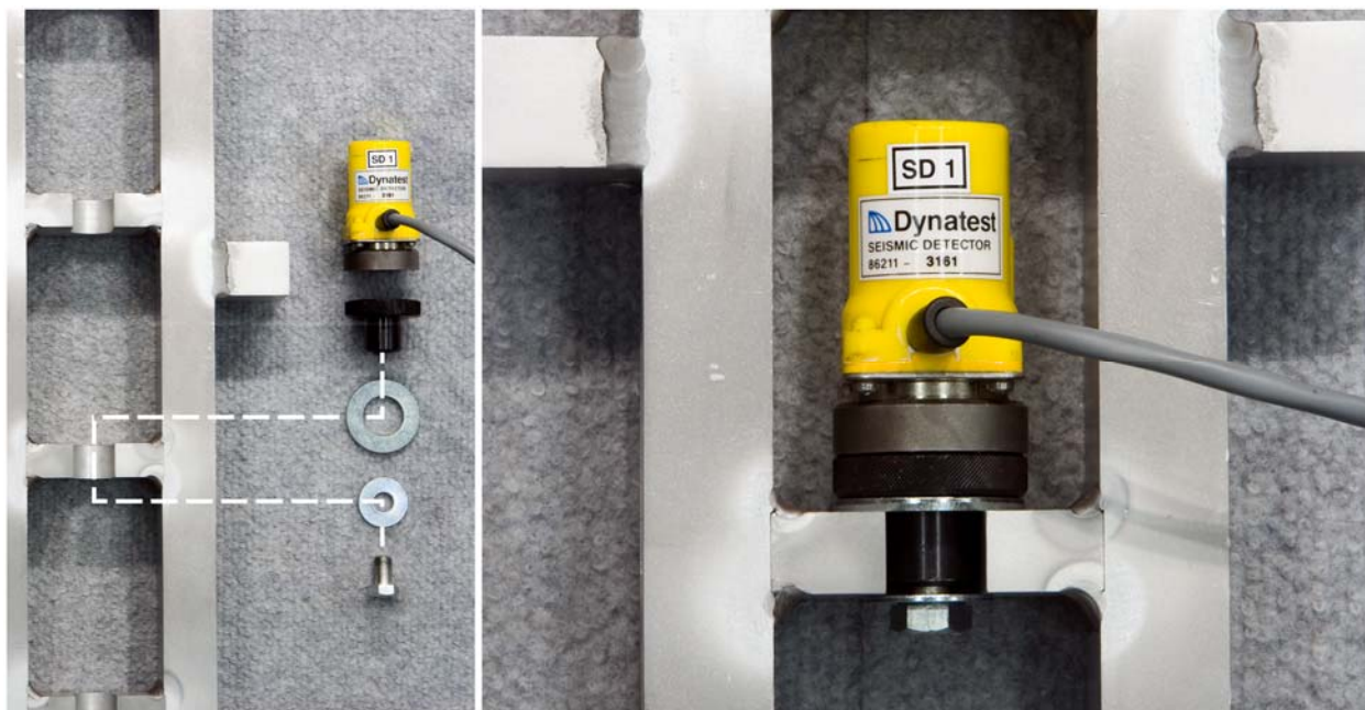
Figure 82. Photo. Attachment of a Dynatest geophone.
