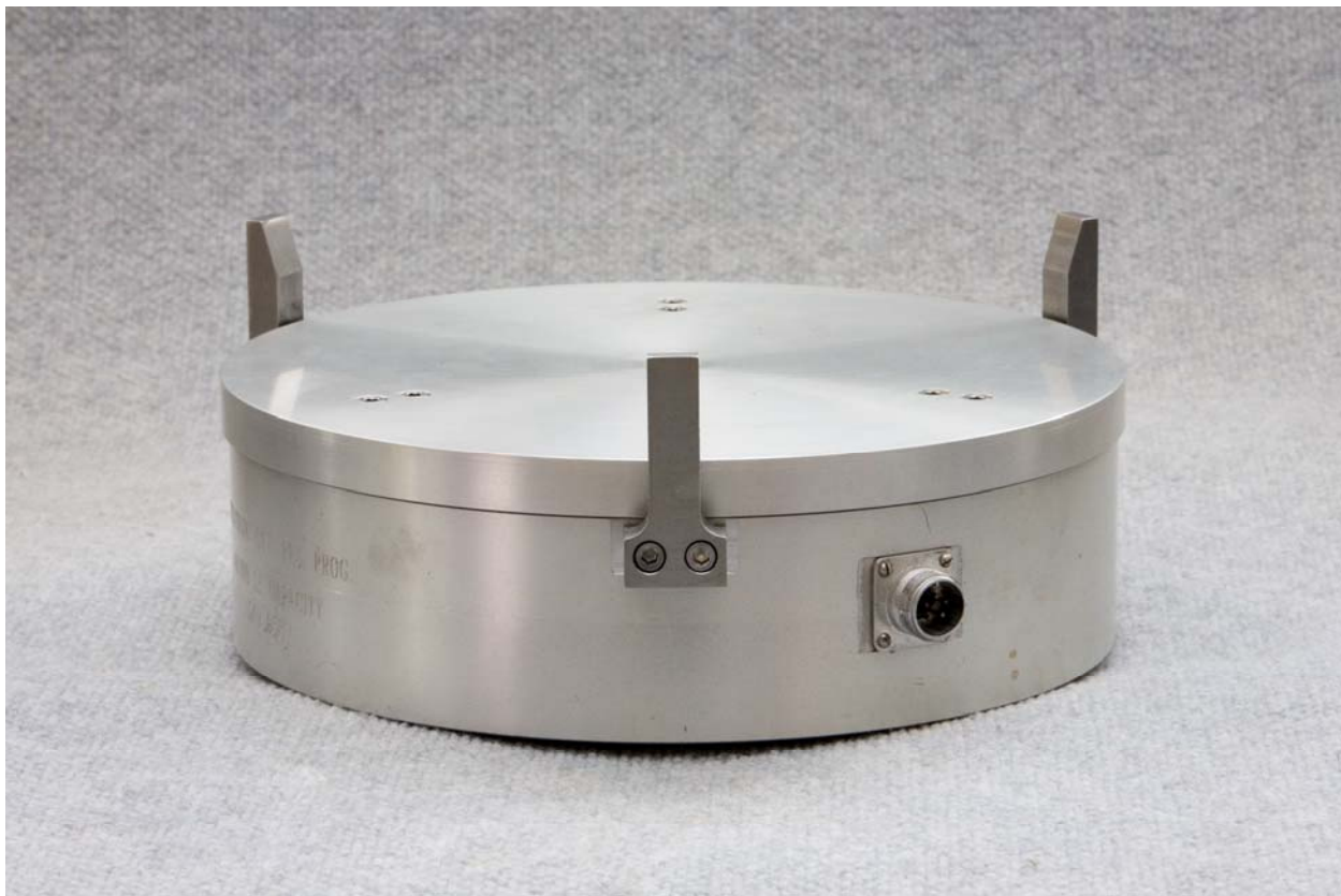
Figure 67. Photo. SHRP reference load cell.
