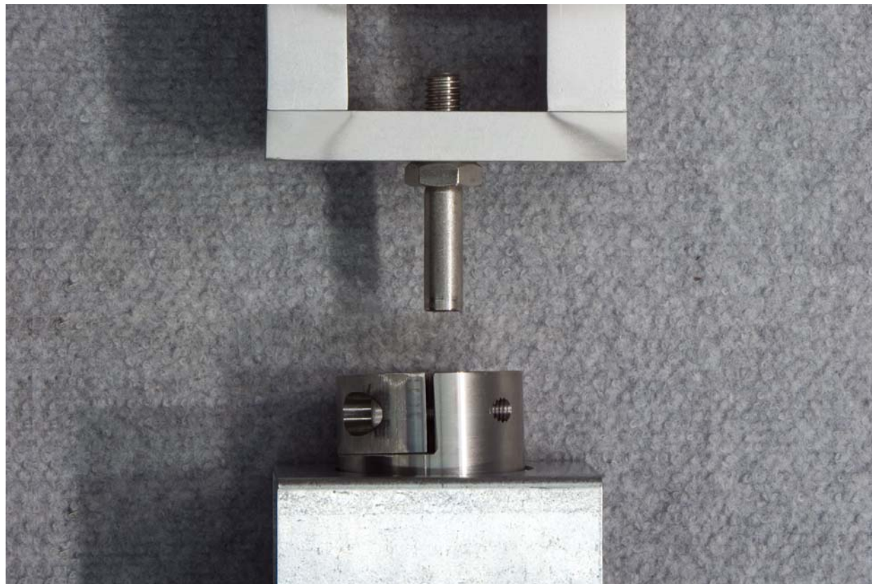
Figure 84. Photo. Coupling the calibration stand and ball joint.
