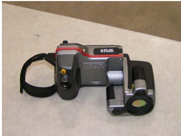
**Figure 3.** Photograph of hand-held IR camera.
