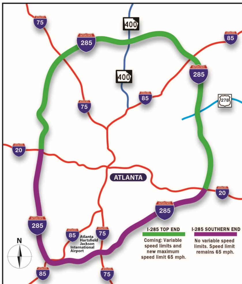
Figure 6-3. VSL Application on the Top End of I-265, Atlanta, GA (adopted from (24))
