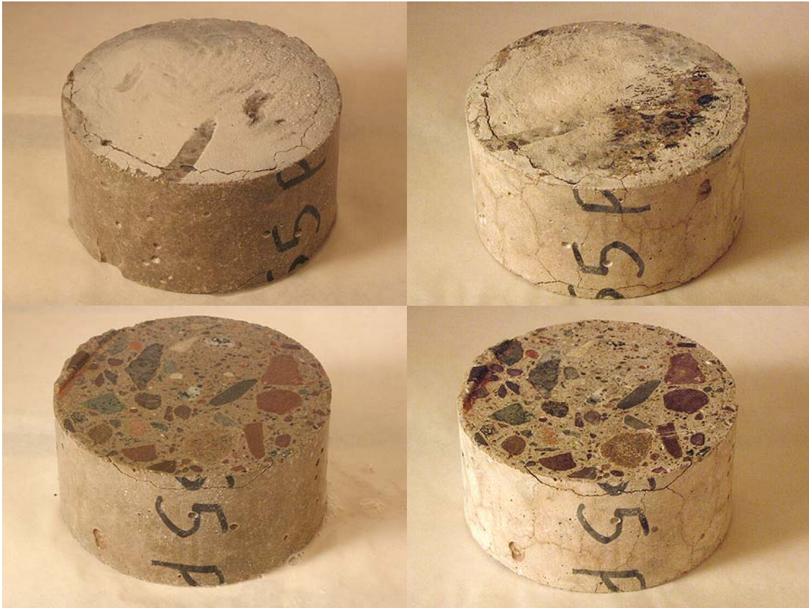
Figure 1: 0.55 w/c concrete specimen immersed in high concentration \text{CaCl}_2 brine for 270 days. Left hand side images show specimen immediately after removal from brine, right hand side images show specimen after drying in convection oven overnight at 50 degrees C.
