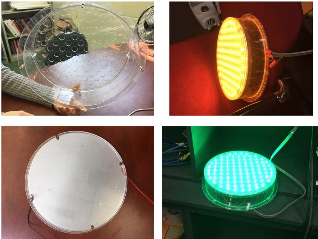
**Figure 1** Three samples the finalized design of the new housing of the fully working prototype signals of Type 1, modelled in the factory of Eco Molding. Each sample includes three plastic parts: the whole-piece of new housing that accommodate 96 small Fresnel lenses for light collimation of individual LEDs, a cover for
