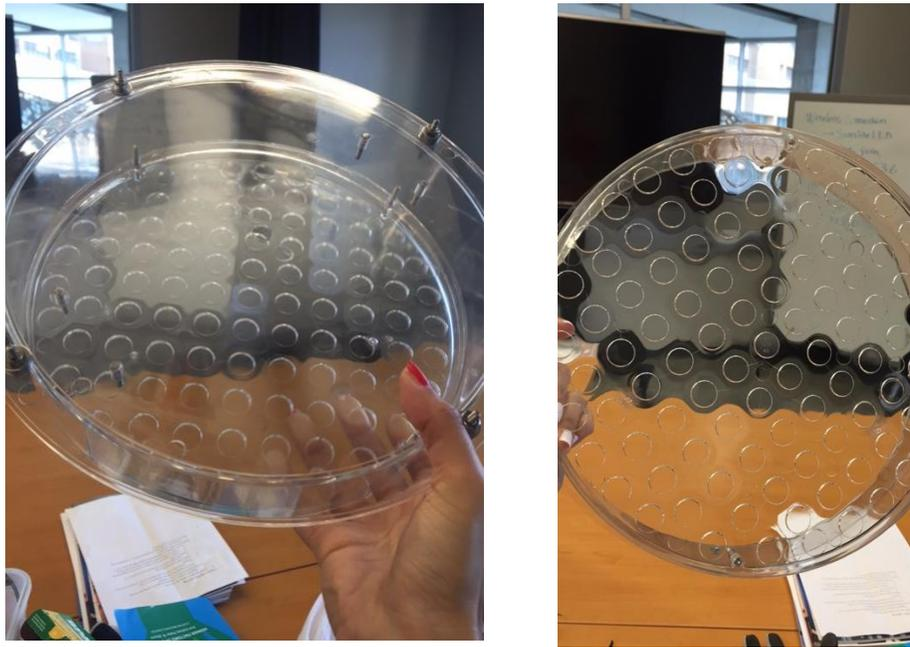
**Figure 3** Six additional samples the finalized design of the new housing of the fully working prototype signals of Type 1, modelled in the factory of Eco Molding. Each sample includes three plastic parts: the whole-piece of new housing that accommodate 96 small Fresnel lenses for light collimation of individual LEDs, a cover for the new light engine, and another back cover for the housing which will be used to mount the new custom-made LED drivers.
