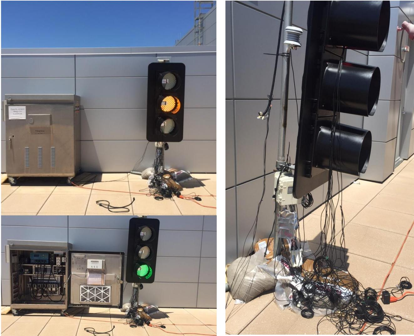
**Figure 4** The closed-course performance and reliability tests of the fully working prototypes mounted on the roof of the University of Kansas engineering complex - M2SEC building. All signal lights were powered by the signal controller cabinet. The test setup on the roof includes the power cabinet, the signal lights mounted on the tripod, a data logger mounted on the tripod pole, and temperature sensors mounted on the surfaces of the signal lights.
