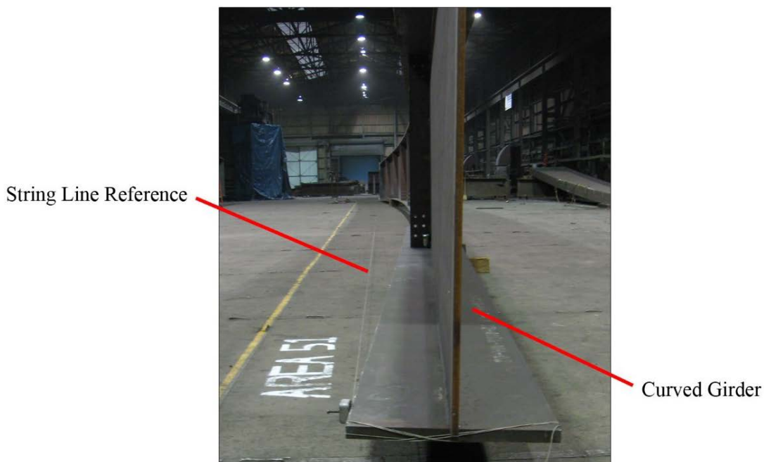
Figure 36. Conventional Measurement of Girder Sweep
