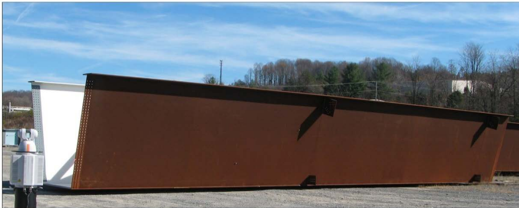
Figure 42. Measurement of a Tub Girder in the Shop Assembly Yard
