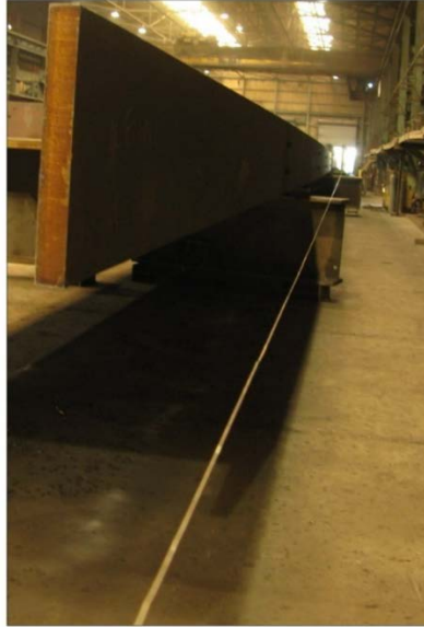
Figure 30. Conventional String Line Measurement of Camber
