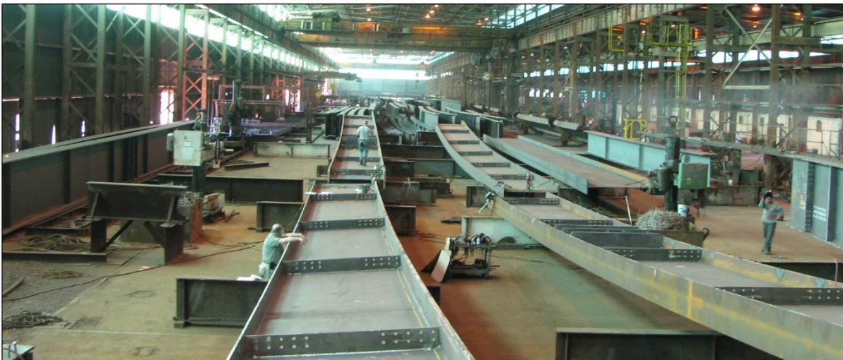
Figure 9. Conventional Laydown Match-Drilling of Girders
