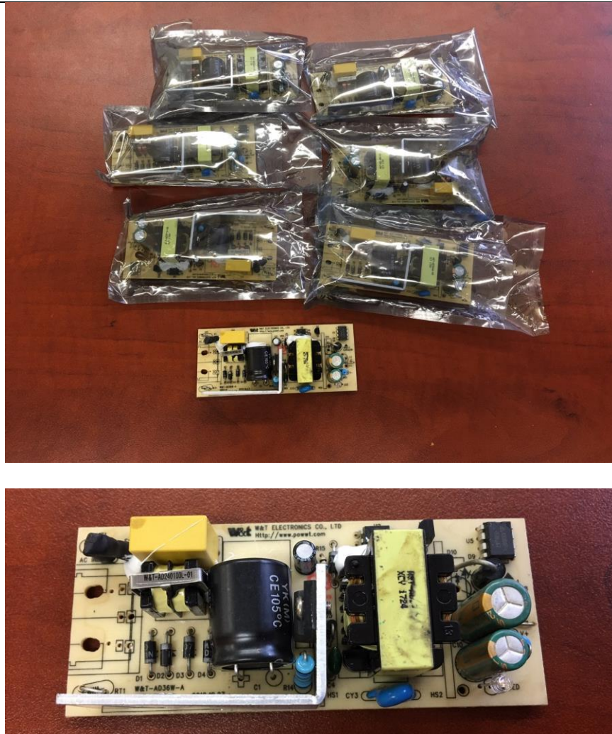
Figure 4 The custom-made LED drivers used to power the LED light engines in red, yellow, and green colors, which will be tested in the to-be-assembled fully working LED signal lights. The specifications include driver for red signal (output 1.1 A, 25.0V, 27.5 W), driver for yellow signal (0.7 A, 38.0 V, 26.6 W), driver for green signal (0.7 A, 38.0 V, 26.6 W).
