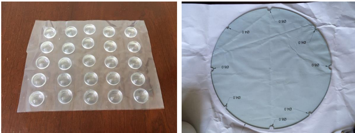
Figure 2 The latest Fresnel lens model # HX-F0150115 (diameter 15 mm, focal length 11.5 mm, and thickness 2.0 mm) and their supporting glass disc (diameter 260 mm, thickness 3mm) custom made in a factory.
