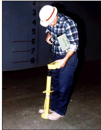
**Figure 24. Clegg hammer test.**
