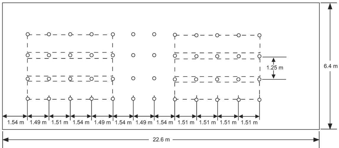
**Figure 22. Locations of elevation and Clegg hammer points.**
