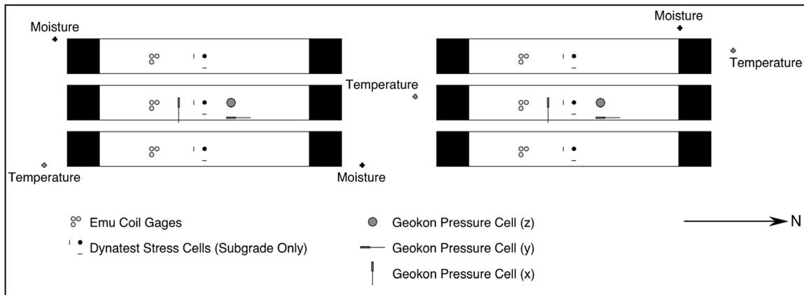
**Figure 29. Proposed locations of instrumentation in test section.**
