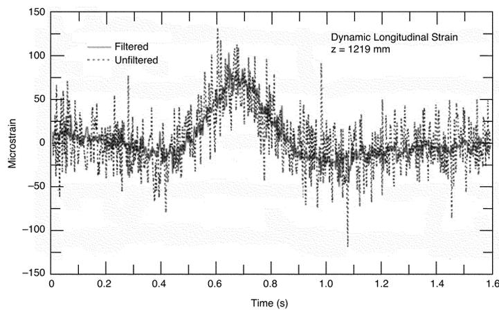
**d. Longitudinal strain at 1219 mm from the surface of the AC layer.**
