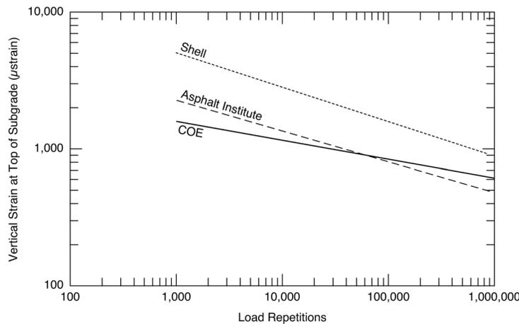
**Figure 4. Different subgrade strain failure criteria.**
