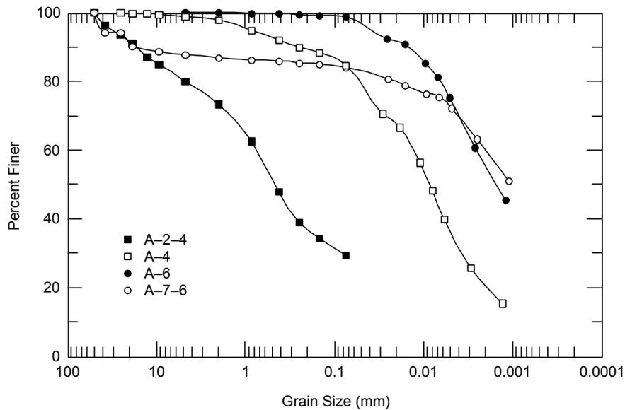
**Figure 6. Grain size distribution of test soils.**
