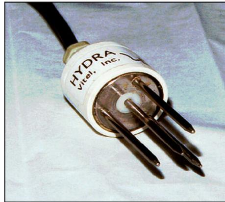
**Figure 30. Thermocouple gage. Figure 31. Vitel Hydra moisture sensor.**
