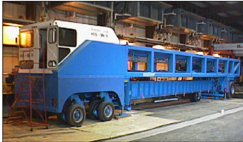
**Figure 21. Heavy Vehicle Simulator (HVS).**
