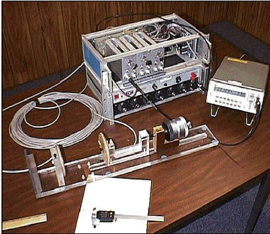
**Figure 48. Calibration system of coaxial coil gages.**
