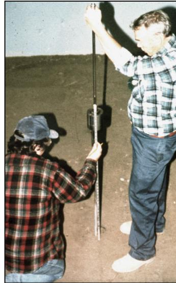
**Figure 27. Dynamic cone penetration test.**
