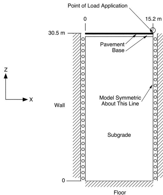
**Figure 15. Finite element model geometry for the control section.**
