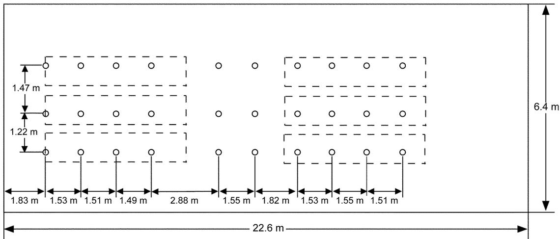
**Figure 28. Locations of moisture and density measurement points.**
