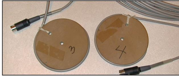
**Figure 40.  $\epsilon$ mu soil strain measurement coils.**
