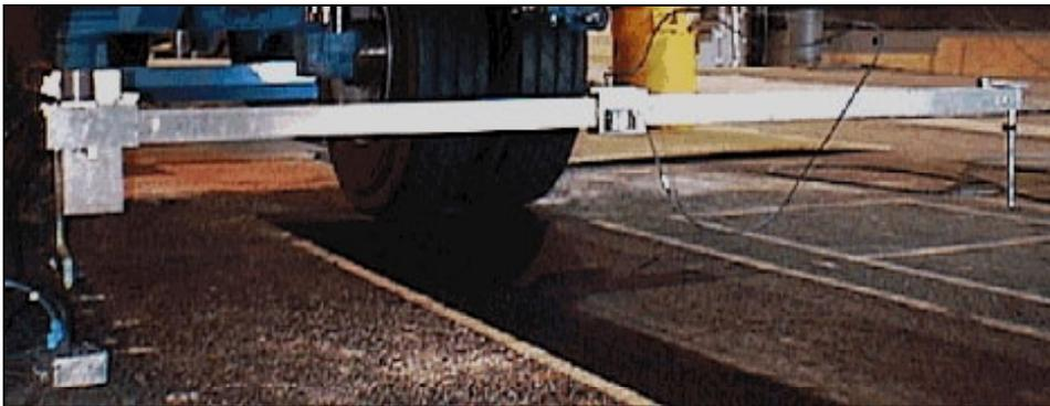
**Figure 51. CSIR surface deformation measurement system.**
