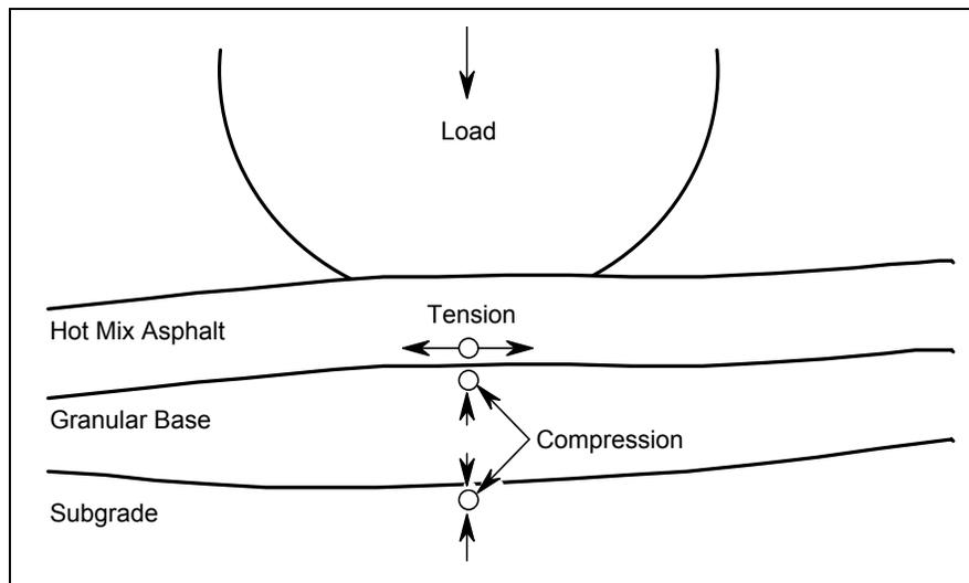
**Figure 1. Tensile and compressive strains in flexible pavements.
