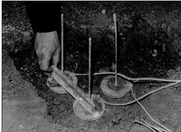
**Figure 47.  $\epsilon$ mu coil placement in a test section.**
