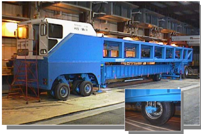
Figure 36. The Heavy Vehicle Simulator (HVS), Mark IV.
