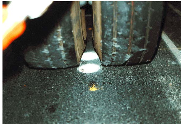
Figure 35a. Location of test wheels over coil and stress cells for Position 1 measurements.
