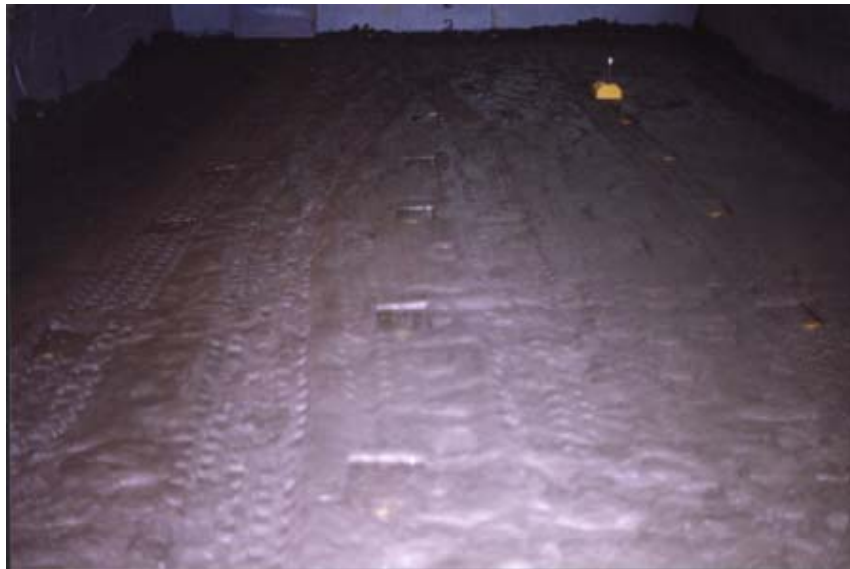
Figure 10a. Degree of softness of subgrade soil at 15% moisture content.
