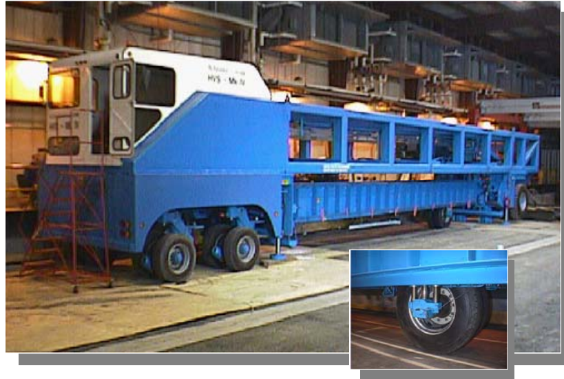
Fig. 21. The Heavy Vehicle Simulator (HVS), Mark IV, used for accelerated testing of the pavement.
