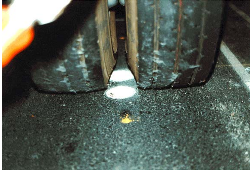
Figure 20b. Location of test wheels over coil and stress cells for Position 2 measurements.
