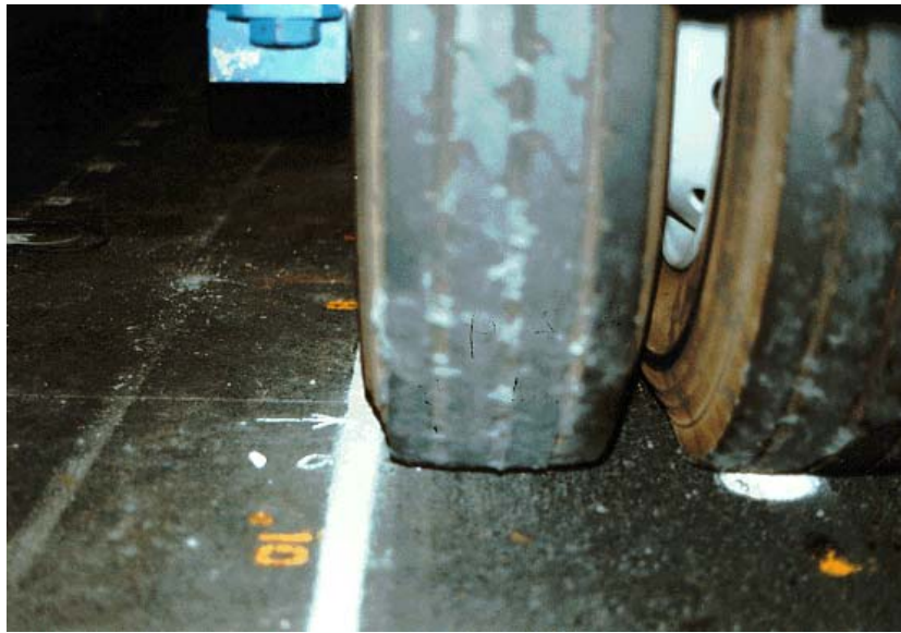
Figure 20c. Location of test wheels over coil and stress cells for Position 3 measurements.
