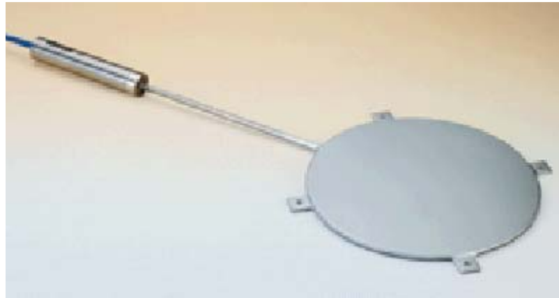
Figure 20. Geokon® stress cell used in the base course.
