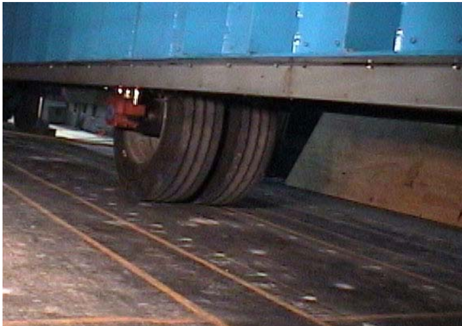
Figure 30. Tire assembly used to apply accelerated traffic
