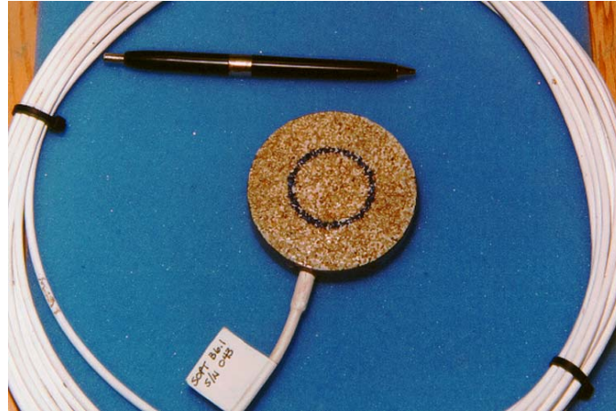
Figure 19. Dynatest® stress cell used in the subgrade.
