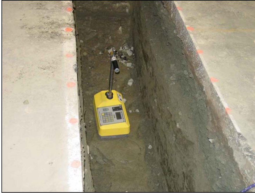
Figure 28. Nuclear gauge density measurement in a trench.
