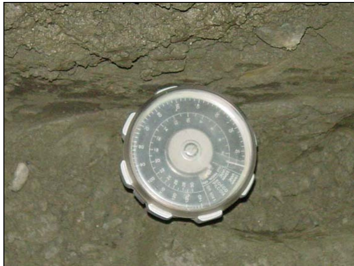
Figure 25. Vane shear measurement in the subgrade.
