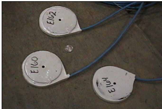
Figure 5. Emu coils. A US 25-cent coin is included for scale reference.
