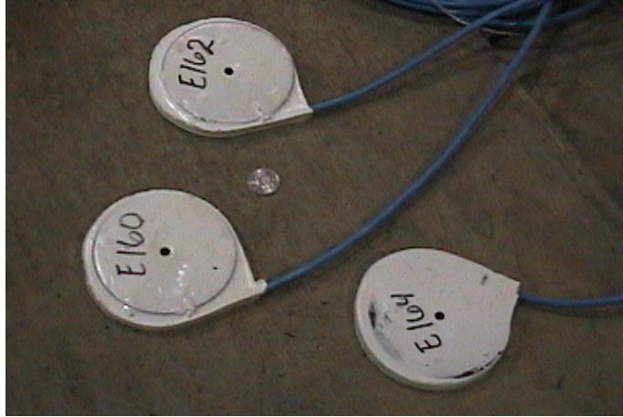
Figure 9. Emu coils in a co-planar arrangement to measure longitudinal and transversal displacements. A US 25-cent coin is included for scale reference.
