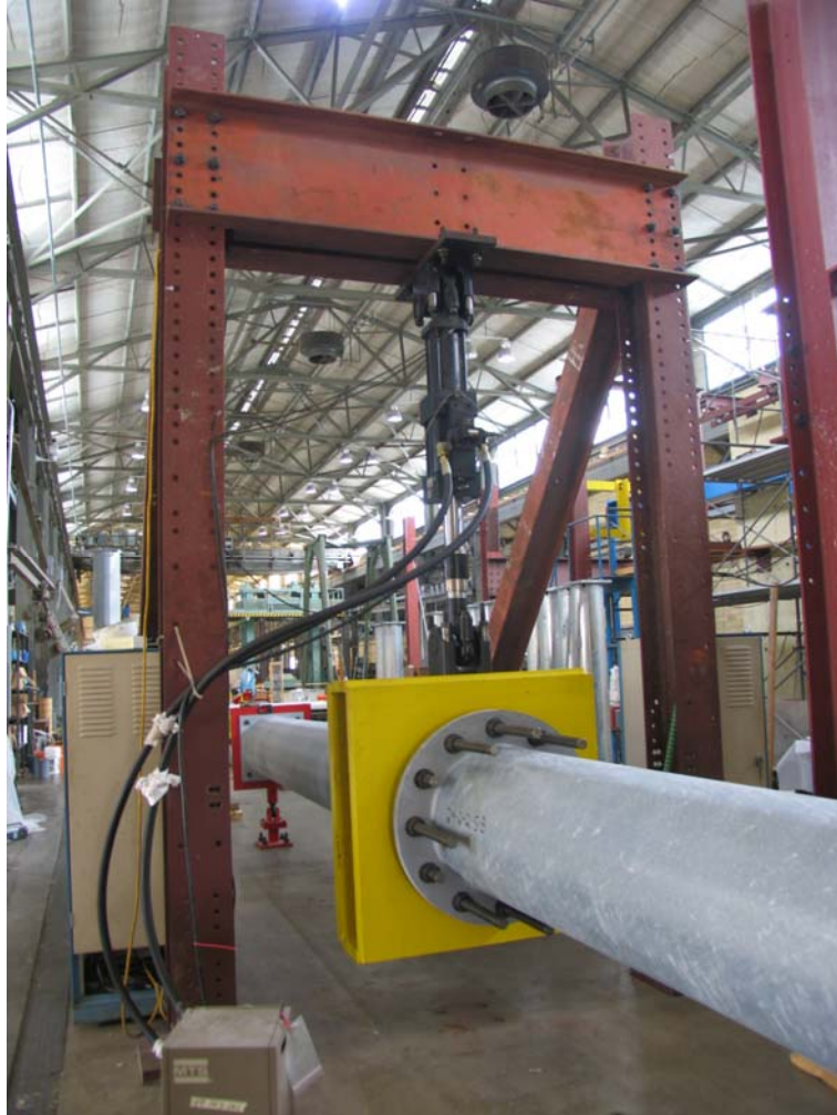
Figure 2: Test Setup for 24" high mast poles
