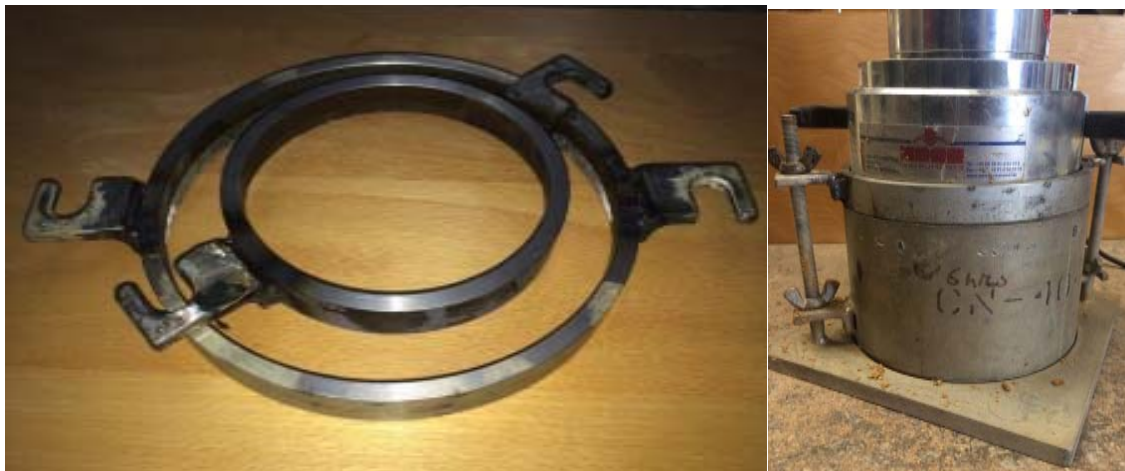
Figure 4-14. Attached collar during LWD on mold testing
