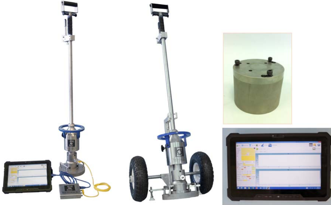
Figure 2-8. Olson LWD-01 with the new ruggedized DELL tablet and optional lighter (~8.5 lbs) drop weight (pictures courtesy of Olson Engineering Inc.)
