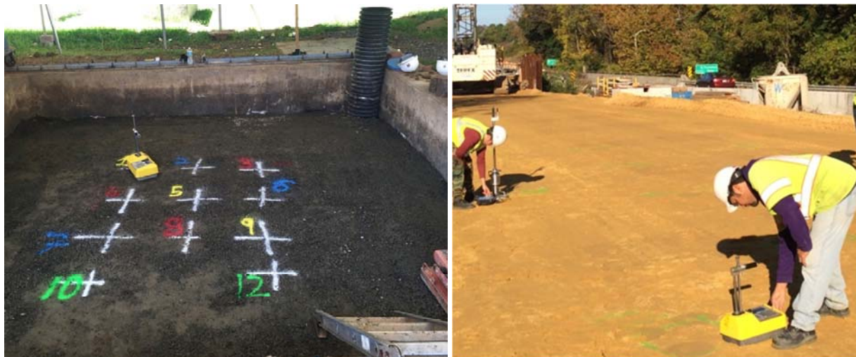
Figure 2-13. Troxler 3440 nuclear moisture-density gauge on the test pit (left picture) and in the field (right picture)
