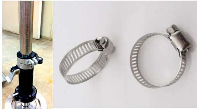
Figure 4-13. Dynatest LWD's movable release handle and laser engraved scale on the guide shaft (left), and adjustable pipe clamps to set lower drop heights for Zorn LWD (right)
