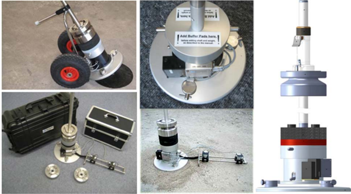
Figure 2-7. Dynatest LWD 3031, including LWD set up with the optional external geophones (pictures courtesy of Dynatest Consulting Inc.)
