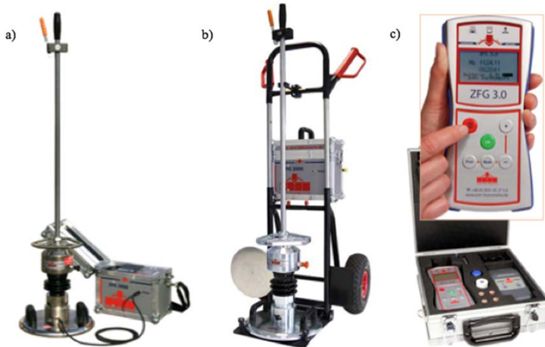
Figure 2-6. Zorn ZFG 3.0 LWD: (a) Zorn LWD with the older data logger and printer system, (b) new Zorn transportation trolley, and (c) new data logger and separate printer (pictures courtesy of Zorn instruments)
