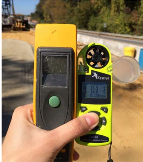
Figure 4-2. Fluke Infrared Thermometer (left) and Kestrel 4300 Construction Weather Tracker (right)
