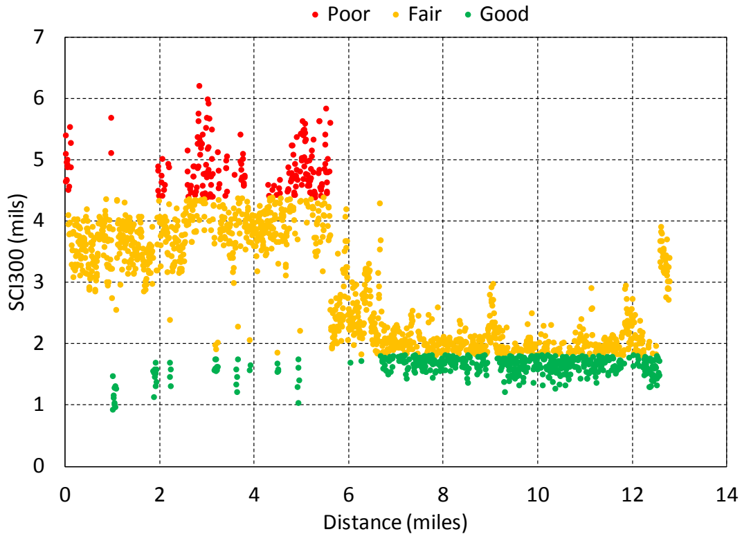
Figure 13 Classification of structural condition on I580 North south based on percentile: 25 th percentile and lower represents good structural condition and 90 th percentile and higher represents poor structural condition
