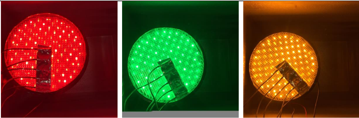
Figure 3 The improved signals of Type 1 with TIN coating.
