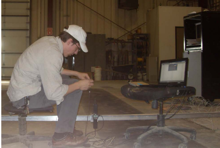
Figure 4.8: Transverse Profile Being Taken Using a Chicago Dial Indicator
