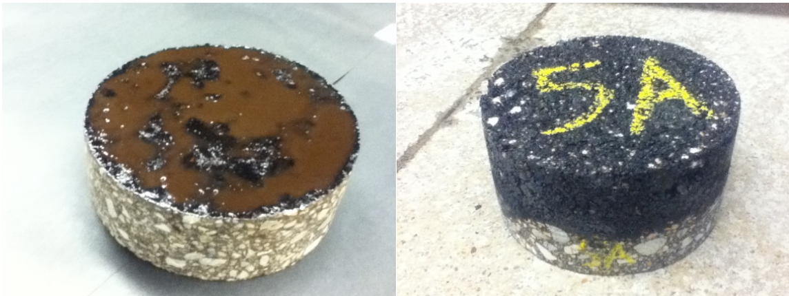
Figure 3.4: Core with Tack that is Breaking and Core with Compacted Overlay
