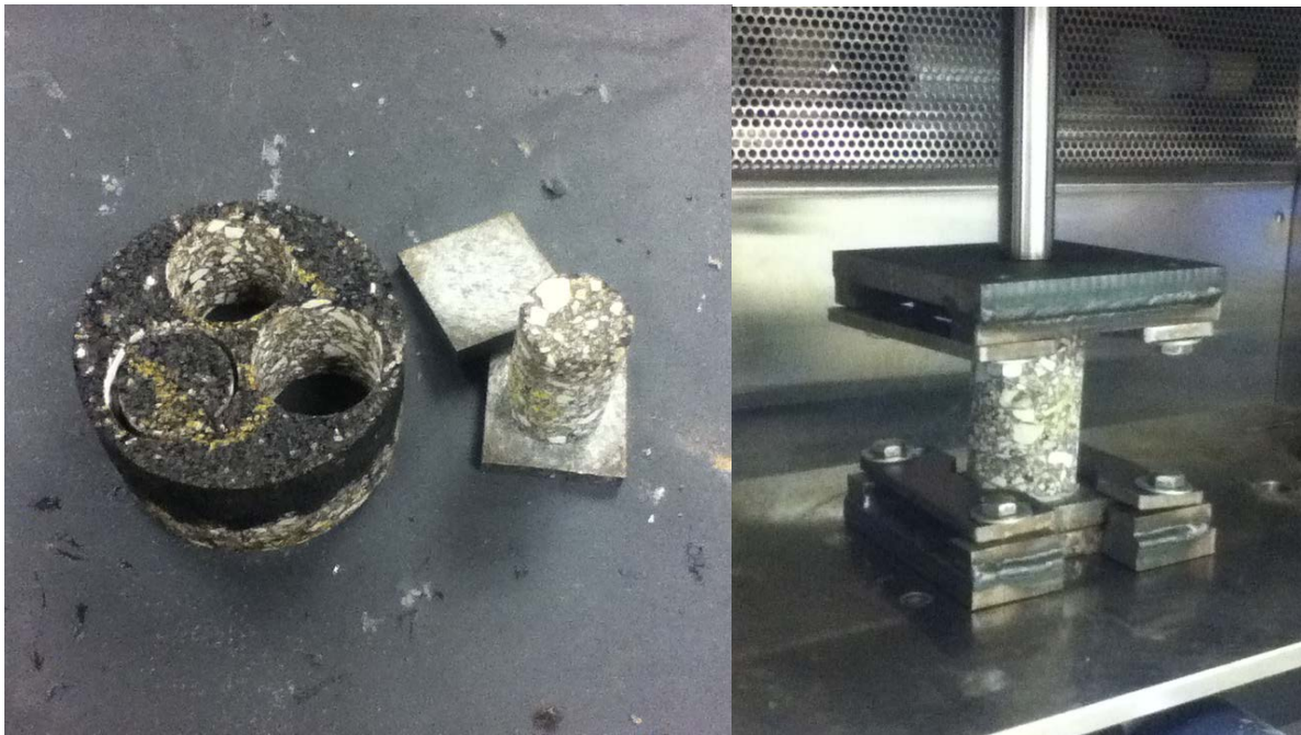
Figure 3.5: (a) Epoxying to Steel Plates, (b) Sample Loaded in the UTM
