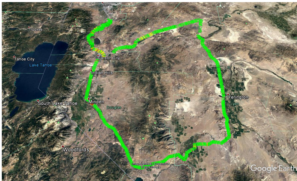
Figure 5. Google Earth color-coded pavement structural condition of tested pavements in Nevada with good (green), fair (yellow), and poor (red) ratings (© 2016 Google Image Landsat/Copernicus).
