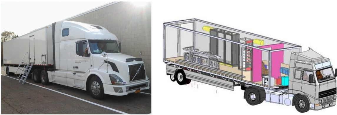
Figure 1. TSD used during testing (left) and computer-generated schematic (right) (Krarup, 2012).
